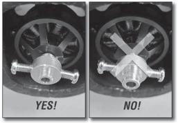
2. It may be necessary to flip the aluminum propeller adapter to the correct orientation.
