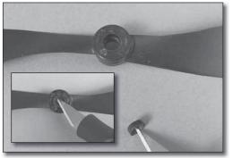
1. Remove the black plastic adapter ring from the rear of the propeller using a hobby knife.
