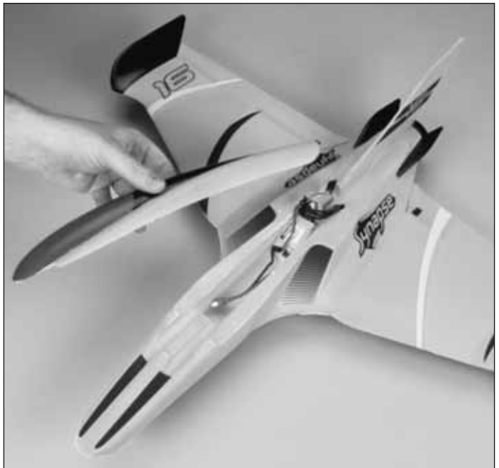
Canopy hatch and fuselage with Ammo Brushless Motor, SS-25 Speed Control, and HyperFlow Ducted Fan installed.
