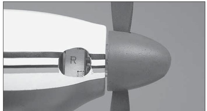
8. Fit one of the spinners all the way onto the propeller and collet assembly. Adjust the cowl so there will be approximately a 1/16" [1.5mm] gap between the spinner and the cowl.
