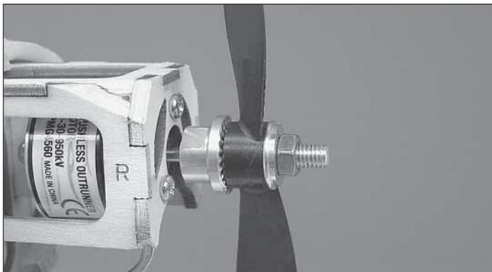
3. Slide the cowl off of the nacelle. Temporarily mount the prop adapter and the propeller to the motor shaft. Use an 8mm wrench to tighten the prop nut while holding the collet with a 10mm wrench to lock the prop adapter onto the shaft.
