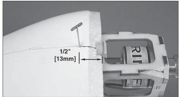
5. Insert a pin into the motor pod 1/2" [13mm] behind the middle of the wood block for the top cowl mounting screw.
