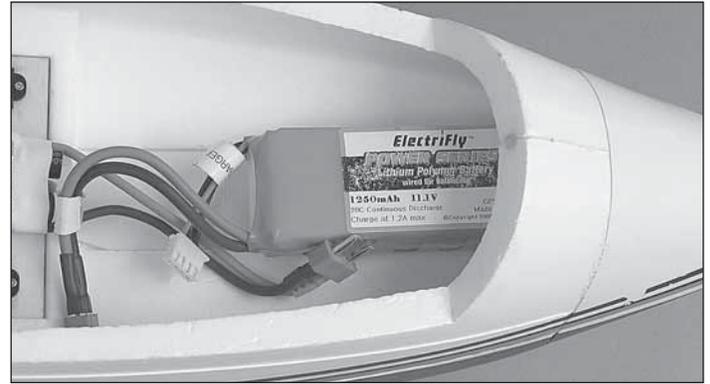
❑ 4. Mount the motor battery as far forward as possible in the fuselage with one strip of the included hook-and-loop material on the battery and the opposing strip in the bottom of the fuselage.
