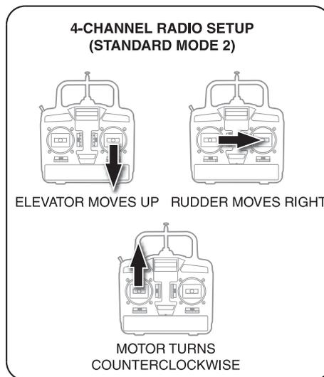
❑ 8. Operate the controls on the transmitter to make sure the elevator, rudder and motor respond in the correct direction.
