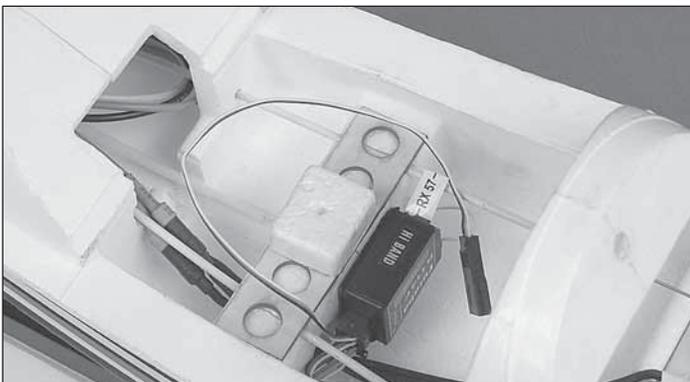
❑ 3. Use the included hook-and-loop material (or optional double-sided foam mounting tape—not included) to mount the receiver where desired. The location shown is preferable because all the wires can easily reach and the receiver will be raised off the cabin floor, making it less likely to get wet if any water leaks in.
