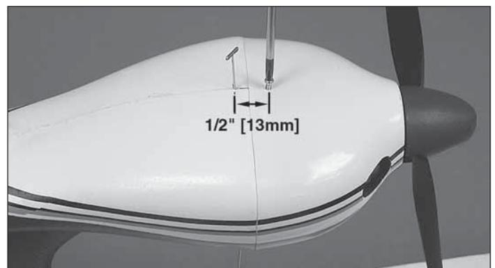
9. Drill a 1/16" [1.6mm] hole through the cowl and the cowl mounting block 1/2" [13mm] ahead of the pin in the top of the motor pod—this should put the screw hole right in the middle of the cowl mounting block. Screw in one of the three larger wood screws that came with this kit.
