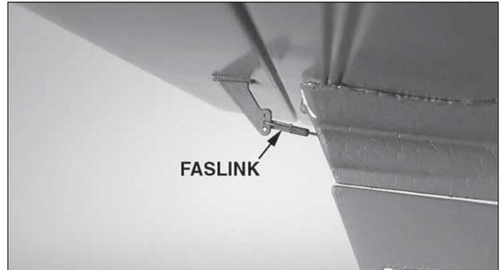
❑ 5. Install the elevator pushrod wire into the middle hole of the elevator control horn. Secure it with the nylon Faslink.
