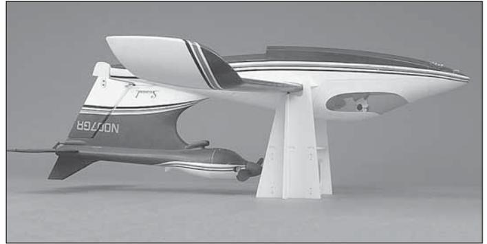
❑ 2. Place the model upside-down on the balance stand as shown. The leading edge of the wings should contact the vertical “stop” on the stand, thus supporting the wing on the correct C.G. location which is 1" [25mm] from the leading edge.
