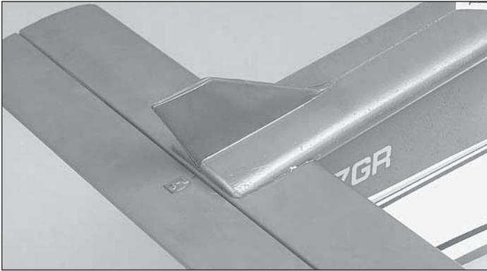
❑ 7. Glue in the fin with the same glue used for the stab—do not clog the receiver antenna tube that comes out of the fuselage by the left side of the fin. View the fin from behind the model to make sure it is vertical.
