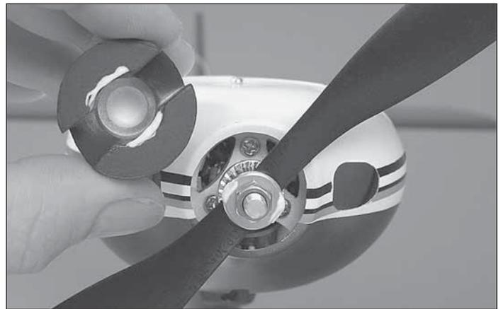
❑ 2. Mount the propeller with the included aluminum propeller washer. Use a few dabs of RTV silicone, R/C 56 or waterproof white glue to glue on the spinner. Using just a few dabs of any of the soft glues recommended should allow the spinner to be removed if ever necessary in the future. If the spinner becomes damaged two spares are provided.
