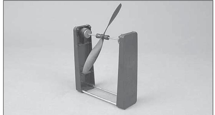
❑ 1. For optimum performance and motor efficiency balance the propeller using a Top Flite® Precision Magnetic Prop Balancer (TOPQ5700) or other suitable balancer. Use a hobby knife or sandpaper to sand the one side of the heavier blade until you can get the prop to balance.
