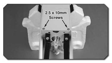
() 5. Line the top and sides of the tank with additional foam rubber. The tank should be held securely by the foam rubber. Fit the fuel tank hatch cover in place and drill two 1/16" [1.6mm] pilot holes through the forward end of the hatch cover and into the firewall. Thread a 2.5x10mm washer head self-tapping
