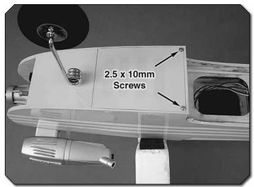
() 12. Install the bottom hatch cover with two 2.5x10mm washer head self-tapping screws. Be sure to harden the wood surrounding the holes with thin CA.
