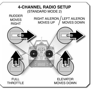
③ 3. Make certain that the control surfaces and the throttle respond in the correct direction as shown in the diagram. If any of the controls respond in the wrong direction, use the servo reversing in the transmitter to reverse the servos connected to those controls. Be certain the control surfaces have remained centered. Adjust if necessary.
