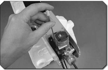
⑦ 7. Position your engine 4-1/4" [108mm] from the firewall. Use a Great Planes Dead Center Hole Locator to mark the location of the engine mount holes onto the engine mount halves. If necessary, carve away any portion of the fuselage that interferes with the needle valve or exhaust. Drill 1/8" [3.2mm] holes through the marks you made.
