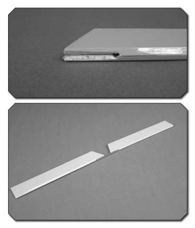
♦ 6. Trim the covering away from the elevator joiner wire slots at the LE of the elevator halves. Confirm that the joiner wire fully seats into the slot. Use a hobby knife to enlarge the slot as necessary. When satisfied, test fit both elevator halves onto the joiner wire and lay them on a flat surface. If both elevator halves do not lay flat, "tweak", or bend the joiner wire until they do. Do not attempt to bend the joiner wire with it inside the elevators.
