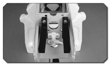
() 3. Use a 4x20mm machine screw, engine mount half, and a 4mm flat washer to draw the four 4mm blind nuts tight into the engine mounting holes. Confirm that the holes you are using line up with the holes in the engine mount halves (the unused holes are for a brushless motor mount). Install the motor mount halves using four 4x20mm machine screws, four 4mm flat washers, and thread locking compound.
