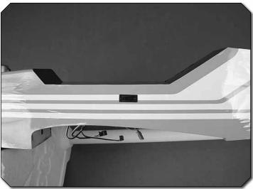
I. Pre-cut slots are provided on both sides of the fuselage for an on/off switch. The slots may need to be enlarged depending on what brand switch harness you are using.
