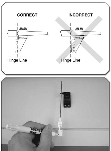
() 6. Position the control horn onto the aileron using the position of the servo arm as a guide. Align the holes in the control horns directly over the aileron hinge line and mark the location of the control horn mounting holes.
