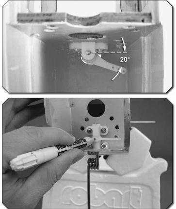
♦ 4. Fit the nylon steering arm between the two nose gear bearing block halves. Slide the nose gear wire up through the bearing blocks and the steering arm. Square the axle of the nose gear wire with the length of the fuselage. Rotate the steering arm so it is approximately 20 degrees to the firewall as shown. Mark the location of the threaded hole in the steering arm onto the nose gear wire.
