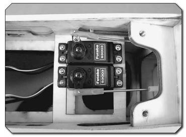
Install the elevator pushrod in the same manner as you installed the rudder pushrod.
