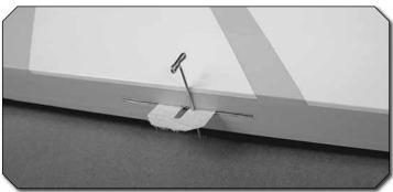
③ ③ 2. Test fit a CA hinge into each of the hinge slots in the wing panel and aileron. If necessary, enlarge the slots with a hobby knife. When satisfied with the fit, insert a CA hinge halfway into each hinge slot in the wing panel. Push a pin through the middle of each hinge to keep them centered.
