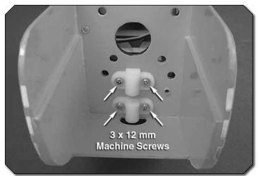
③ 3. Cut apart the nose gear bearing block halves and rotate them around 180 degrees. Install the bearing block halves onto the firewall using four 3x12mm washer head machine screws and thread locking compound.
