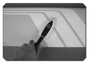
♦ 2. Remove the tape and separate all the control surfaces. Use a covering iron with a covering sock on high heat to tighten the covering if necessary. Apply pressure over sheeted areas to **thoroughly** bond the covering to the wood.
