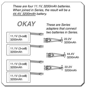
$\Box$  1. Connecting batteries in "**Series**" means to connect the +'s to the -'s and the -'s to the +'s. This combines the batteries' Voltages, but the capacity remains the same.
