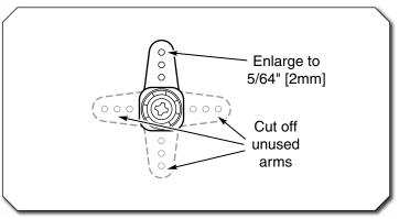
() () 2. Cut three arms from a four-armed servo arm for the aileron servo. Enlarge the outer hole of the remaining arm with a 5/64" [2mm] drill bit.
