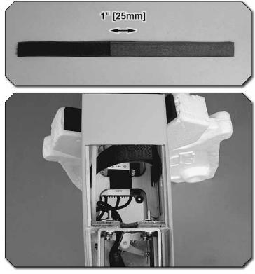
♦ 4. Apply a piece of self-adhesive hook and loop material inside the battery compartment (don't forget a coat of epoxy to improve adhesion). Make a strap from the included hook and loop strap material to fit around your battery packs by overlapping the mating ends by approximately 1" [25mm]. Fit the strap ends through the slots in the battery tray. Cut the strap to length as needed.
