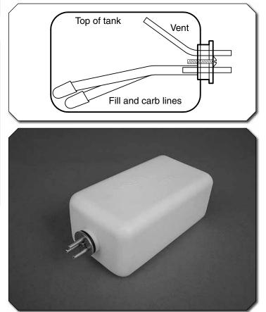
③ 2. Fit the stopper assembly into the tank with the vent line pointing toward the top of the tank, but not touching. The fuel tubing and clunks (fuel pickup) on the carb and fill lines should almost reach the back of the tank but not touch. The clunks must be able to move freely inside the tank when assembled. Adjust the length of the fuel tubing accordingly. When satisfied, remove the stopper from the tank. It will need to be reinstalled after the tank is fit into the fuselage.
