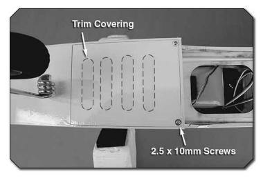
() 6. Fit the ESC hatch cover in place and drill through the pre-cut mounting holes into the hardwood rail using a 1/16" [1.6mm] drill bit. Thread a 2.5x10mm washer head self-tapping screw into each hole and back it out. Apply a drop of thin CA to each hole to harden the wood. Install the hatch cover using two 2.5x10mm washer head self-tapping screws. Trim the covering from the cool air exit slots in the hatch cover.
