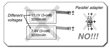
**NEVER** connect battery packs with different Voltages in **Parallel**–only combine in **Series**. Otherwise, the batteries will try to "equalize" with the larger one trying to "charge" the smaller one, thus causing heat and likely a fire.
