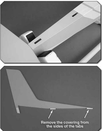
$\circledast$  8. Trim the covering from the **vertical fin** slots in the fuselage. If necessary, remove the covering from the sides of the tabs on the vertical fin.
