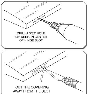
( ↓ 1. Drill a 3/32" [2.4mm] hole 1/2" [13mm] deep into the center of each hinge slot in the **aileron** and **wing panel**. Trim the covering away from each hinge slot to ensure that the hinges will be properly glued in place.
