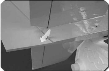
$\circledast$  13. Install a control horn onto the right side of the rudder in the same manner.
