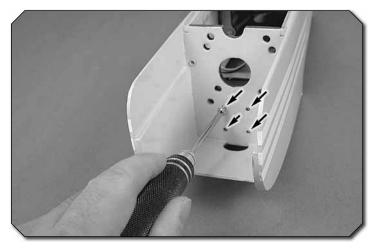
2. Push a 3mm blind nut into the back of each nose gear bearing block mounting hole in the firewall. Use a 3x12mm washer head machine screw to draw the blind nuts tight against the firewall.
