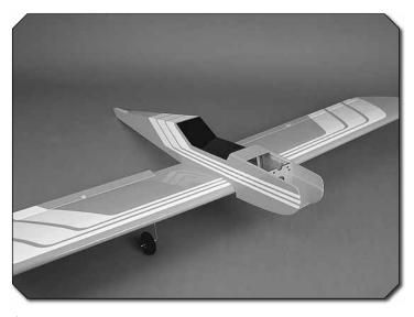
② 2. Place the horizontal stab onto the stab saddle as shown. Center the stab left and right on the fuse (making a center mark on the stab is helpful) and make the distance between wing and stab tips equal on both sides. When satisfied, use a felt-tip pen to trace around the saddle where it meets the underside of the stab. We used a small clamp to hold the stab in place while we did this.
