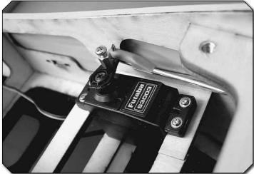
2. Thread a nylon clevis 20 complete turns onto a 29-1/2"
