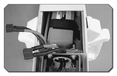
♦ 5. Test fit your battery packs in the battery compartment. They can be secured together with additional self-adhesive hook and loop material, but the packs may need to be inserted into the compartment one at a time.
