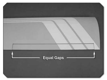
() () 3. Join the aileron to the wing panel and remove the pins from the hinges. Center the aileron on the wing. Remove the pins and adjust the aileron so there is a small gap between the LE of the aileron and the wing. The gap should be small, just enough to see light through the gap or to slip a piece of paper through.
