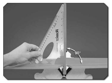
(▶ 10. Use 30-minute epoxy to glue the fin into place. Be sure to put a coating of epoxy along the entire underside length of the fin as well as the side of the tabs. Wipe away any excess epoxy with denatured alcohol. Use a triangle or measure to confirm that the vertical fin is installed perpendicular to the
