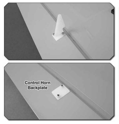
( 7. Drill 5/64" [2mm] holes at the marks you made through the aileron (drill perpendicular to the aileron chord line). Apply a couple drops of thin CA glue to each hole to harden the surrounding wood. When the glue has dried, install the control horn onto the aileron using two 2 x 20mm machine screws and a control horn backplate. The excess length of screw protruding beyond the backplate can be cut off.
