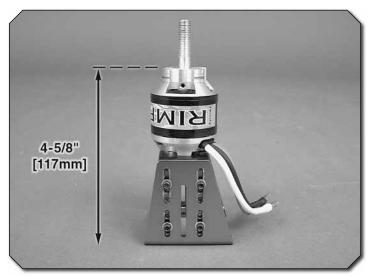
● 1. Attach the out-runner motor to the brushless motor mount using the included 3 x 8mm machine screws and thread locking compound. If you haven't done so yet, install the prop adapter to the motor case with the hardware included with the motor and thread locking compound. Loosen the screws that hold the two motor mount halves together and set the distance from the back side of the mount to the front of the prop washer to be 4-5/8" [117mm]. Retighten the screws using thread locking compound.
