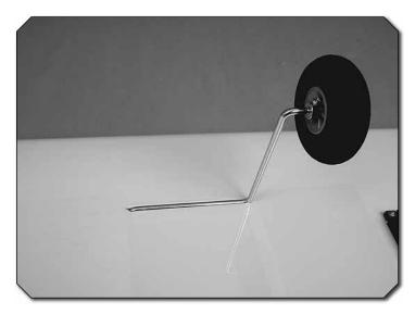
③ 2. Press the landing gear into the slots on the underside of the wing.
