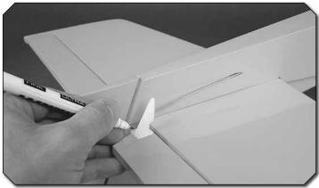
() 11. Trim the covering from the tail servo pushrod exits on the left and right sides of the fuselage. Temporarily insert a 29-1/2" [749mm] pushrod into the elevator outer pushrod tube that exits the left side of the fuselage. Use the position of the pushrod to mark the location for the elevator control horn onto the underside of the elevator.
