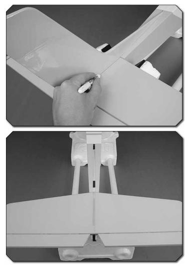
$\oplus$  9. Fit the vertical fin onto the fuselage and use a felt-tip pen to trace around it onto the fuselage. Remove the covering 1/16" [1.6mm] inside the lines you drew.
