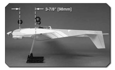
( ) 2. With the wing attached to the fuselage, all parts of the model installed (ready to fly) and an empty fuel tank, place the model upside-down on a Great Planes CG Machine,<sup>™</sup> or lift it upside-down at the balance point you marked.
