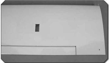
() () 1. Trim the covering from the aileron servo bay on the underside of the wing panel.
