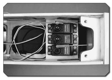
Image 9. Mount the throttle servo onto the servo tray. Make sure that it is not touching the elevator servo. Use your radio system to center the servo.
