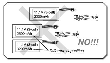
Also **NEVER** connect battery packs with different capacities in Series or in Parallel.
