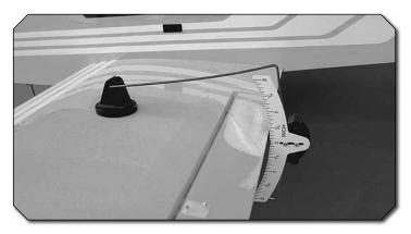
Use a Great Planes AccuThrow<sup>™</sup> (or a ruler) to accurately measure and set the control throw of each control surface as indicated in the chart that follows. If your radio does not have dual rates, we recommend setting the throws at the **low** rate setting.
