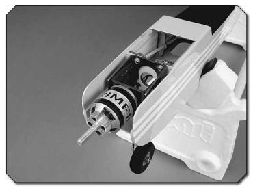
♦ 2. Locate the pre-drilled holes in the firewall that match up with the Great Planes medium motor mount. Use a 4x20mm machine screw and a 4mm flat washer to draw four 4mm blind nuts tight into the holes. Attach the motor mount to the firewall using four 4x20mm machine screws, four 4mm flat washers, and thread locking compound.
