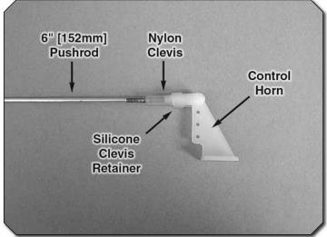
() ③ ⑤ 5. Thread a nylon clevis 20 complete turns onto a 6" [152mm] pushrod. Slide a silicone clevis retainer onto the clevis and connect the clevis to the outer hole of a control horn.
