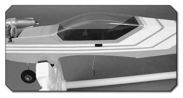
③ 3. Apply the instrument panel decal (see Apply the Decals section). Use canopy glue to glue the canopy in place as shown. Tape the canopy down and allow the glue to dry overnight. The canopy can also be screwed into place (additional screws not included).
