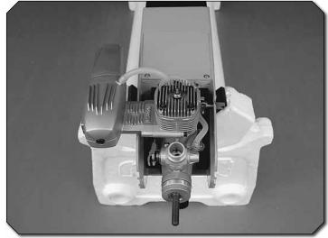
11. Make any final connections to the engine such as the pressure line to the muffler, carb line, etc. If you assembled the fuel tank with a fill line, cut the fill line to length and plug the line with a fuel line plug (not included).
