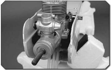
8. Attach the engine to the engine mount halves using four
