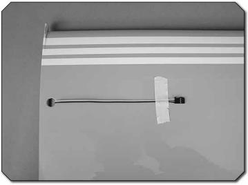
() 9. Route the servo lead through the hole in the top of the wing panel and tape it back and out of the way.
