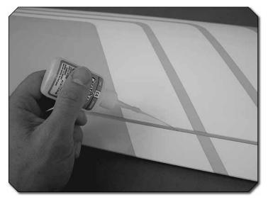
♦ 4. Apply six drops of thin CA to the top and bottom of each hinge without using accelerator. After the CA glue has hardened, confirm that the aileron is secure by pulling on it and deflecting it up and down.
