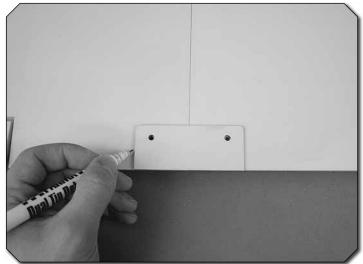
4. Trim the covering from the holes in the plywood wing bolt plate as shown. Position the wing bolt plate over the wing bolt holes on the underside of the wing and use a felttip pen to trace around it.
