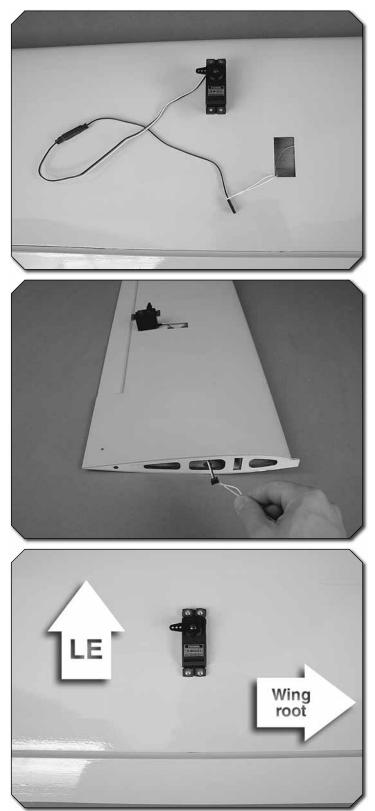
♦ 4. Use the string taped inside the aileron servo bay to pull the servo lead through the wing ribs. Fit the servo into the servo bay with the spline toward the LE of the wing. Drill 1/16" [1.6mm] holes through the mounting tabs on the servo case into the wing. Thread a servo mounting screw (included with the servo) into each hole and back it out. Apply a drop of thin CA to each hole to harden the wood. When the CA has dried, install the servo using the hardware supplied with the servo.
