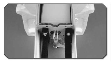
♦ 4. Cut a piece of 1/4" [6mm] foam rubber (not included) to fit the fuel tank. Lay the foam rubber inside the fuel tank compartment. Fit the fuel tank into the compartment and pull the fuel tank neck through the hole in the firewall. Install the stopper into the tank (be sure the correct side is facing up). Do not over-tighten the stopper screw.
