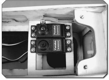
③ 3. Install the elevator servo next to the rudder servo using the hardware included with the servo. Be sure that the two servos are not touching each other.
