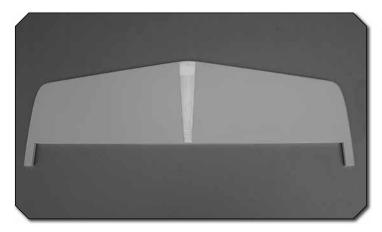
♦ 4. Remove the stab from the fuse and trim the covering 1/16" [1.6mm] inside the lines you drew. Be careful not to cut into the wood structure beneath the covering. Use denatured alcohol to wipe away the lines.
