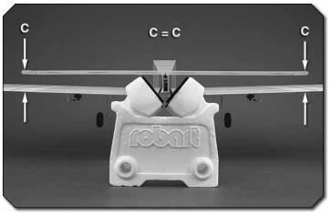
3. Stand back 5-6 ft [1.5 - 1.8m] and view the model from behind. Confirm that the stab and wing are parallel. If not, sand the fuselage as necessary until they are parallel.
