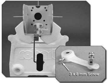
♦ 5. Remove the nose gear wire from the bearing blocks. As you did with the main gear, install two 4mm wheel collars and a wheel onto the nose gear wire and mark the positions of the wheel collar screw holes onto the axle. Grind flats spots for the wheel collar screws at your marks as well as for the
