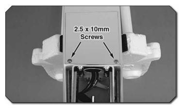
⑦ 7. Mount the battery hatch cover using two 2.5x10mm washer head self-tapping screws.
