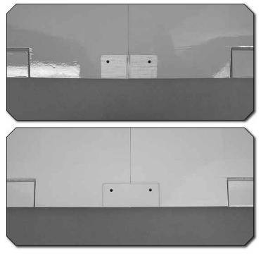
() 5. Use a sharp #11 hobby knife or use the following **Expert Tip** to cut the covering 1/16" [1.6mm] inside of the lines you marked. Use care to cut **only in the covering** and **not into the wood**. Use alcohol to wipe away the lines. Glue the wing bolt plate in position. If necessary, clean out the wing bolt holes using a 11/64" [4.4mm] drill bit.
