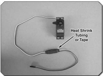
() () 3. Attach a 9" [229mm] servo extension to the aileron servo and secure the connector using tape, heat shrink tubing (not included), or a product designed specifically for securing servo lead connections. Center the servo with your radio system and install the servo arm to the servo perpendicular to the servo case as shown. Be sure to reinstall the servo arm screw into the servo.
