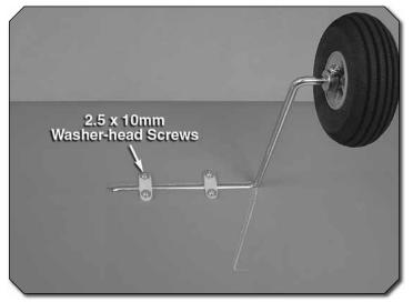
③ 3. Position two landing gear straps evenly spaced apart over each landing gear and mark the location of the strap holes onto the wing. Drill holes at your marks using a 1/16" [1.6mm] bit. Thread a 2.5x10mm self-tapping washer head screw into each hole and back it out. Apply a drop of thin CA to each hole to harden the wood. When the glue has dried, install the straps using eight 2.5x10mm self-tapping washer head screws.
