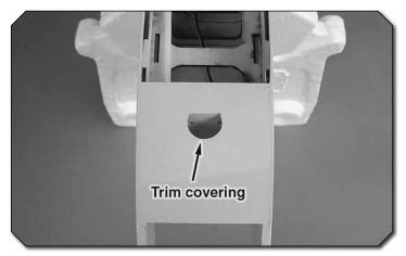
I. Trim the covering from the nose gear exit at the front underside of the fuselage.
