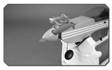
♦ 4. Install the spinner backplate, propeller, prop washer, prop nut, and spinner cone onto the engine crankshaft. The spinner backplate (and propeller) may need to be drilled or reamed larger to match the crankshaft diameter. Be sure to balance your prop!
