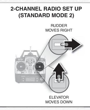
() 3. Make certain that the control surfaces respond in the correct direction as shown in the diagram. If any of the controls respond in the wrong direction, use the servo reversing in the transmitter to reverse the servos connected to those controls. Be certain the control surfaces have remained centered. Adjust if necessary.
