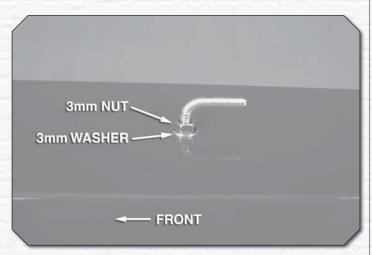
() 3. Trim the covering from the forward tow hook hole (approximately 11-13/16" [300mm] back from the front of the fuse). Thread the 3mm nut and 3mm washer all the way onto the tow hook. Tighten the tow hook into the blind nut. With the hook threaded almost all the way into the blind nut and pointing straight back, tighten the 3mm nut to secure it.
