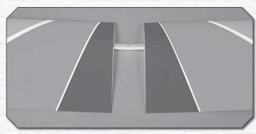
() 1. Test fit the **wing joiner** into the **wing panels**. The point of the "V" shaped joiner should point to the bottom of the wing panels. Sand the wing joiner or root ribs if necessary to achieve the correct fit. The root ribs should join together tightly with no gaps and the joiner should be just slightly loose in the joiner pockets to allow room for epoxy.
