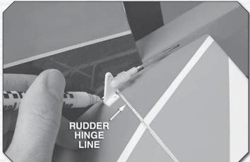
() 6. Insert the rudder pushrod into the rudder outer pushrod tube from the aft end. Align the holes in the control horn over the rudder hinge line and mark the locations of the control horn mounting holes onto the rudder. Drill two 5/64" [2mm] holes at the marks on the rudder. Apply a drop of thin CA into each hole to harden the balsa.
