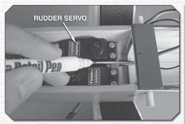
③ 8. Use a small clamp or tape to hold the rudder in the neutral position. Mark the pushrod where it crosses the outer hole in the rudder servo arm.
