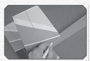
$\bigcirc$  7. Fit the fin post into the slot in the stab. Trace around the fin, being sure it is aligned over the fuse center line (a reference line drawn on the fuselage is helpful to keep the fin aligned with the center of the fuselage. Cut the covering 1/16" [1.6mm] inside the lines you drew and use alcohol to wipe away the lines.
