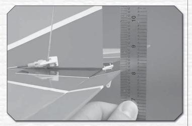
Use a Great Planes AccuThrow (or a ruler) to accurately measure and set the control throw of each control surface as indicated in the chart that follows. If your radio does not have dual rates, we recommend setting the throws at the **low** rate setting.
