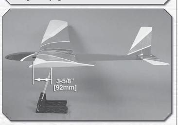
③ 2. With the wing attached to the fuselage and all parts of the model installed (ready to fly), place the model on a Great Planes CG Machine, or lift it at the balance point you marked, using your fingertips.
