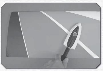
Remove the tape and separate all the control surfaces. Use a covering iron with a covering sock on high heat to tighten the covering if necessary. Apply pressure over sheeted areas to **thoroughly** bond the covering to the wood. JOIN THE WING PANELS
