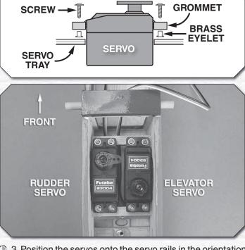
$(\ensuremath{\triangleright}$  3. Position the servos onto the servo rails in the orientation shown. Drill servo mounting holes using a 1/16" [1.6mm] drill
