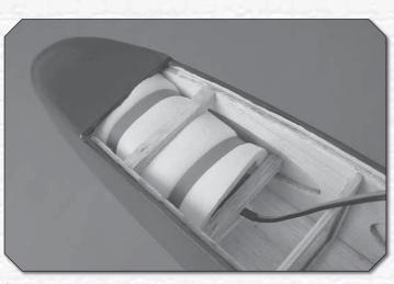
() 2. Wrap your receiver battery in 1/4" [6mm] foam rubber (not included). Fit it into the front radio compartment. Cut pieces from the included 6x6x200mm balsa stick and glue them along the top and back of the battery to hold it in place using CA or epoxy. When gluing the sticks, be sure that the radio hatch cover can be installed without interference.
