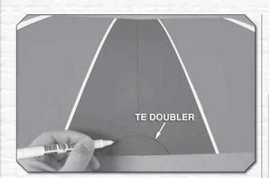
③ 3. Center the plywood **TE doubler** along the TE of the wing as shown. Use a felt-tip pen to trace around the doubler onto the wing.
