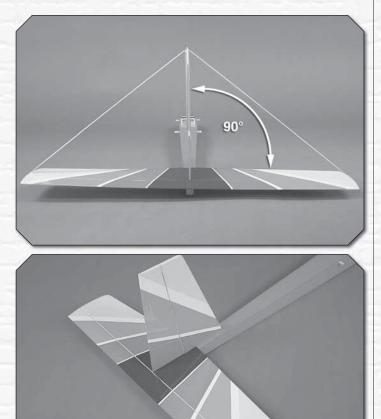
() 8. Epoxy the fin in place. Confirm that the fin is perpendicular to the stab. Use tape if necessary to hold the fin square to the stab while the epoxy cures.
