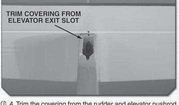
③ 4. Trim the covering from the rudder and elevator pushrod exit slots.
