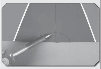
Guide the soldering iron at a rate that will just melt the covering and not burn into the wood. The hotter the soldering iron, the faster it must travel to melt a fine cut. Peel off the covering.
