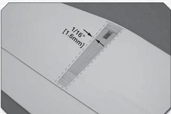
③ 4. Remove the stab from the fuse and trim the covering 1/16" [1.6mm] inside the lines you drew. Be careful not to cut into the wood structure beneath the covering. Use denatured alcohol to wipe away the lines.
