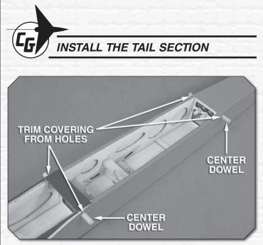
① 1. Trim the covering from the rubber band dowel holes in the sides of the **fuselage**. Center the dowels in the holes as shown and glue them in place with CA or epoxy.
