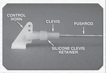
() 5. Thread a nylon clevis onto a 31-1/2" [800mm] pushrod 20 complete turns. Slide a silicone clevis retainer over the clevis. Temporarily attach the clevis to the second inner hole of a control horn (separate the control horn backplate from the control horn).
