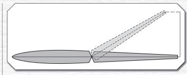
**NOTE**: The throws are measured at the **widest part** of the elevator and rudder. If you are using a ruler to set your control surface throws, the deflection distance is measured as the height from the center trailing edge of the control surface when moved from the neutral position as shown in the sketch. Deflection in degrees is also provided for an alternative measuring method.
