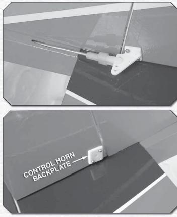
7. Install the control horn using two 2x10mm machine screws and the control horn backplate.
