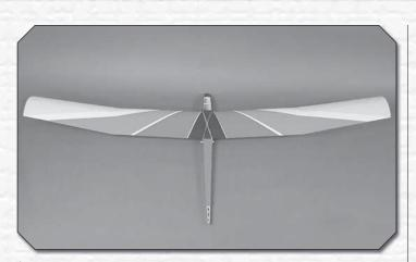
③ 2. Center the wing on the fuselage and secure it using two crisscrossed rubberbands as shown.
