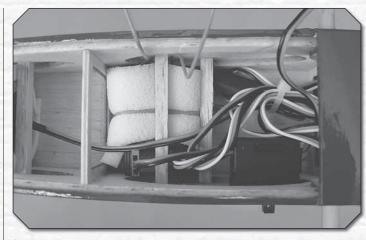
③ 3. Connect the battery to the switch. It is highly recommended to secure the connection using tape, heat shrink tubing (not included), or a clip designed specifically for that purpose. Connect the elevator and rudder servo leads to the receiver. Wrap the receiver in foam rubber and install it behind the battery using pieces of the 6x6x200mm stick. We used a zip tie (not included) to neatly bundle the excess wires behind the receiver. A rubberband could also be used.
