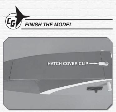
○ 1. A small hole is pre-drilled behind the radio hatch opening. Thread the 2.5x5mm self-tapping screw into the hole and remove it. Apply a drop of thin CA to the hole to harden the wood. When the glue has hardened, install the nylon radio hatch cover clip using the 2.5x5mm screw and 2.5mm washer. The screw should be tight, but still allow the clip to swivel on the screw. Fit the hatch cover in place and secure it with the clip as shown.
