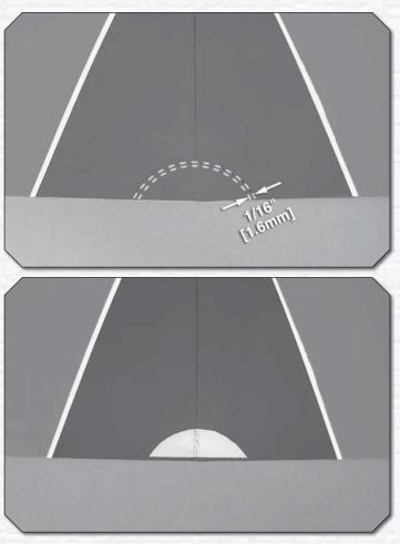
() 4. Use a sharp #11 hobby knife or use the following **Expert Tip** to cut the covering 1/16" [1.6mm] inside of the lines you marked. Use care to cut **only the covering** and **not into the wood**. Use alcohol to wipe away the lines. Glue the doubler in position with CA or epoxy.
