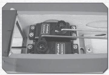
① 11. With the elevator in the neutral position, mark the pushrod where it crosses the hole in the elevator servo arm. Remove the pushrod from the fuse. Make a "Z" bend in the pushrod and reinstall the pushrod. Make any adjustment to the clevis necessary so the elevator is centered when the servo is centered. Be sure to slide the silicone clevis retainer to the end of the clevis and that the servo arm screw in the elevator is installed.
