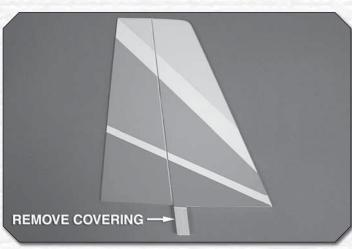
() 6. Trim the covering from the **vertical fin** post as shown. Be careful not to cut into the wood.
