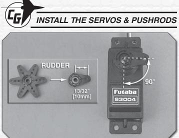
() 1. Select a servo arm that offers a hole location of 13/32" [10mm] from the center. Remove all but one of the arms of the servo arm. Trim the servo arm beyond the hole that is 13/32" [10mm] from the center. Use a file or sandpaper to round over the corners of the arm. Enlarge the outer hole with a 5/64" [2mm] drill bit. Center the rudder servo with your radio system and install the servo arm perpendicular to the servo case as shown.
