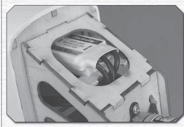
() 3. Mount the ESC to the ESC mounting plate with doubleside foam mounting tape (not included).
