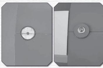
() 13. If necessary, use a 1/8" [3.2mm] drill to clear any epoxy from the wing bolt hole near the trailing edge of the wing. Cut the covering from the bottom of the wing around the wing bolt hole for the plywood **wing bolt washer**. Glue the washer into position while simultaneously mounting the wing to the fuselage with a 3 x 20mm Phillips screw and a 3mm washer. (The wing will be used as a reference for stab alignment in the following steps.)
