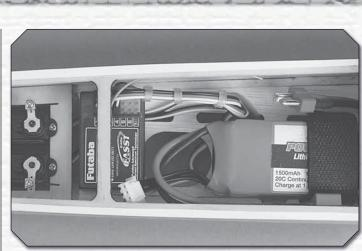
() 3. Connect the servo wires and a dual aileron extension wire to the receiver. Use double-sided foam mounting tape to mount the receiver where desired. If your receiver is small enough, it could be mounted next to the battery on the left side of the fuselage, but this one was mounted behind the battery.
