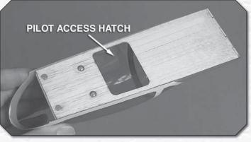
() 4. Mount the pilot to the cockpit floor with two #2 x 1/4" [6mm] or #2 x 1/2" [12mm] screws and #2 washers (not included).
