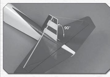
4. Glue the fin into position, making certain it is perpendicular to the stab—use strips of tape—varying the tension on whichever side necessary, to hold it vertical.
