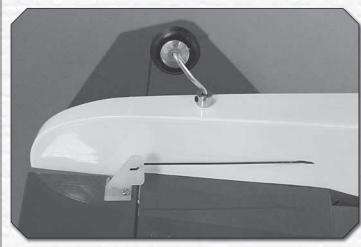
() 3. Connect the other pushrod to the last control horn and mount it to the elevator the same way.
