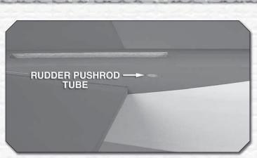
() 1. Use a hobby knife with a sharp blade to cut the covering from the fuselage over the exit slot for the elevator pushrod guide tube (located just under the leading edge of the slot for the horizontal stabilizer) and from the exit slot for the rudder pushrod guide tube (located just behind and below the slot for the vertical stabilizer). The stab is shown already in position, but yours should not yet be in place.
