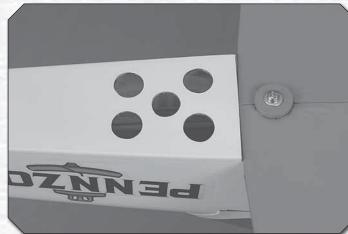
③ 12. Cut the covering from the holes in the bottom of the fuselage to allow cooling air to exit.
