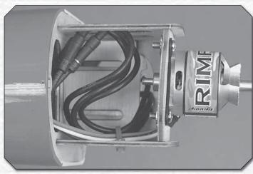
() 4. Using 3.5mm male bullet to 2.0mm female bullet adapters (GPMM3122, not included), connect the ESC wires to the motor wires, keeping as much of the wiring as you can in front of the fuselage in the cowl area so it will not be in the way of the battery—when installing the battery later, it should be placed forward to reduce any nose ballast that will be required to get the proper C.G.
