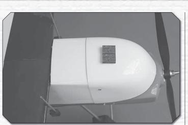
③ 2. Place the model on your C.G. Machine or lift it with your fingers at the balance point you marked on the top of the wing. When the model is balanced correctly the wing and horizontal stabilizer will be level as shown in the photo. If the tail is low additional ballast will be required in the nose. To find out how much, carefully lay segments of Great Planes "stick-on" lead (GPMQ4485) on the fuselage over the location where it will be permanently attached inside.
