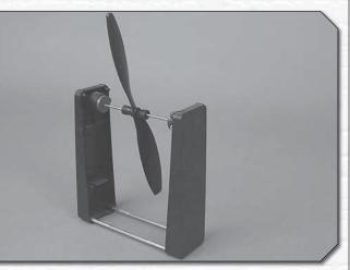
() 1. For optimum performance and motor efficiency, balance the propeller using a Top Flite Precision Magnetic Prop Balancer (TOPQ5700) or other suitable balancer. Use a hobby knife or sandpaper to sand the one side of the heavy blade until you can get the prop to balance.
