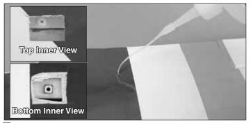
□ 2. Using medium CA insert the CA tip 1/8" into the dimple. Next, squeeze a small amount of CA into the wing. (This is also a good time to add CA to the four strut inserts on the bottom of the upper wing and the top of the lower wing.) After you have completed this on all four dimples turn the wing over to allow the CA to cure or harden and properly secure the nylon insert.
