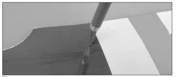
□ 1. On the underside of the wing, use a hobby knife to remove the covering from the four dimples that locate the cabane strut attachment points. Be careful not to insert the knife tip more than 1/8" into the dimple. (Do not use the drilling method mentioned in step 4 as this could dislodge the insert.)
