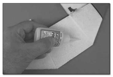
☐ 2. Apply thick or medium CA to the center section of the horizontal tail where it contacts the fuselage.
