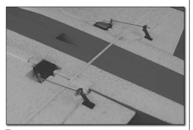
□ 4. Install the 1 x 60mm wire pushrods onto each aileron servo so that the Z-bend is in the hole you drilled on the servo arm. Deflect each aileron up and fit the pushrod into the screw-lock pushrod connector. Apply a drop of thread locking compound to the screw threads and install the locking screw. Set each aileron at neutral throw and tighten the locking screw.
