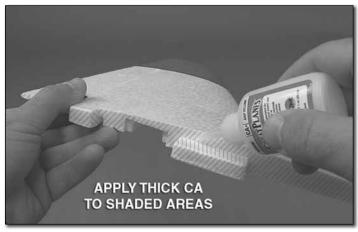
☐ 5. Apply thick CA to the wing tabs and the wing root of each wing where the wing will join with the fuselage. **Note:** Wipe the glue across all mating surfaces. Remove excess glue so that the CA does not run when the wings are joined.
