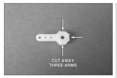
☐ 5. Cut three arms from two four-armed servo arms. Enlarge the outer holes in the servo arms with a 1/16" [1.6mm] drill bit.
