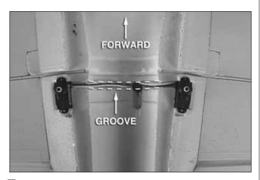
☐ 1. Begin by gluing the elevon servos into the servo bays with the servo splines facing forward. Thick foam safe CA glue or epoxy can be used. Guide the servo wires down the grooves molded into the ducted fan channel and through the hole as shown.
