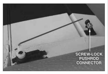
☐ 6. Attach a pushrod wire with a Z-bend at one end to the outer hole of each servo arm. Secure the servo arms to the servos parallel to the elevon hinge line using the servo arm screws included with the servos. Attach a screw-lock pushrod connector to each control horn using a screw-lock pushrod connector retainer.
