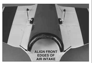
☐ 10. Use thick CA glue or mix up approximately 3/8oz [5cc] of epoxy to glue the lower duct channel half onto the fuselage. Coat the area in duct channel half between the fan unit mold lines with a thin coat of glue or epoxy. Coat the edges of the duct channel half (being sure to use enough adhesive along all contact surfaces) and press the piece into place aligning the front air intake edges with the underside of the fuselage. Wipe away any excess glue with a dry paper towel.
