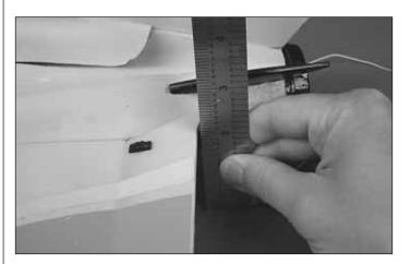
Use a Great Planes AccuThrow (or a ruler) to accurately measure and set the control throw of each control surface as indicated in the chart that follows. If your radio does not have dual rates, we recommend setting the throws at the **low** rate setting.
