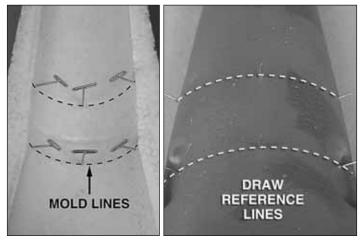
9. After your model is assembled, the only way to remove the ducted fan unit in case of repair or replacement is to cut
