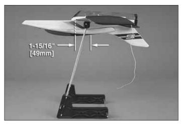
☐ 2. With all parts of the model installed (ready to fly), place the model upside-down on a Great Planes CG Machine, or lift it upside down at the balance point you marked.
