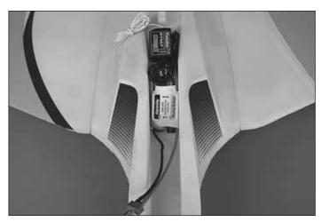
☐ 12. Connect the servos and ESC to the receiver. Install the receiver and ESC in the locations shown. They can be secured using small pieces of the included hook and loop material or double-sided foam servo tape (not included).
