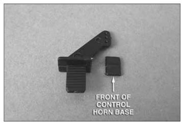
☐ 3. Cut away the front of the control horn base at the tab of both control horns. Enlarge the outer holes of the elevon control horns with a 1/16" [1.6mm] drill bit.
