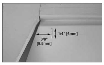
☐ 2. Use a sharp hobby knife to cut slots for the control horns 3/8" [9.5mm] from the inside edge of the elevons at the leading edge just behind the bevel. The slots should be
