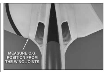
☐ 1. Use a felt-tip pen or 1/8" [3mm]-wide tape to accurately mark the C.G. on the top of the wing on both sides of the fuselage. The C.G. is located 1-15/16" [49mm] back from the leading edge of the wing at the fuselage (the seam where the wing panels have been joined to the fuselage).
