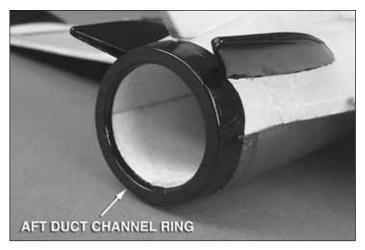
☐ 11. Glue the aft duct channel ring into place with thick CA glue or epoxy.
