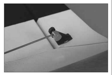
☐ 7. Insert the other end of the pushrod wires into the screw-lock pushrod connectors. Position the elevons in the neutral position and thread a knurled thumb screw into the screw-lock connectors. Tighten the screws against the pushrod wires.
