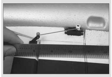
**Note:** When setting the neutral points of the elevons, place a straight edge on the underside of the wings from the carbon tube back to the elevons. For your first few flights, position the neutral points of the elevons level with the wings as shown.
