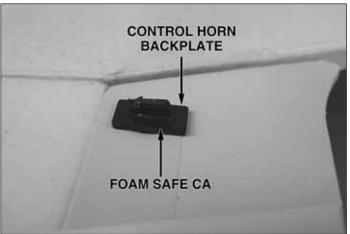
4. Install the control horns onto the undersides of the elevons by fitting the control horn tabs into the slots you made. Secure the control horns to the elevons with a couple drops of foam safe CA. Clip the control horn backplates onto the tabs at the tops of the elevons. Add another drop of **foam safe CA** to each backplate to hold it in place.
