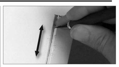
3. Again, using care not to cut through the cloth hinge, use the tip of a sharp #11 blade in a side-to-side motion to scrape excess paint from the leading edge of the aileron—begin at the root end and work all the way down to the tip. The way that works best is to use your finger as a "depth gauge" to keep the tip of the blade from going in too far. And rather than pushing down hard, use light pressure and several strokes to remove a little at a time.
