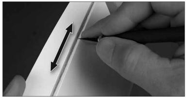
4. Use the same procedure to scrape excess paint from the hinge gap on the wing.
