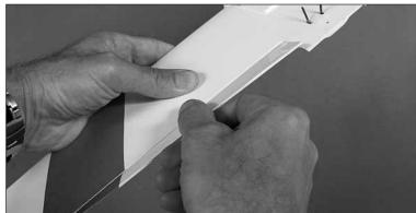
5. Once you think you've got enough paint out of the way, flex the aileron up and down a few times to see if it's free. Repeat as necessary, then perform the same procedure for the other aileron. You should be surprised by how quick and easy the process is and pleased with how much it frees up the ailerons.
