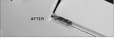
1. Using care not to cut through to the top of the wing, "shave" excess glue from where the torque rod goes into the aileron.
