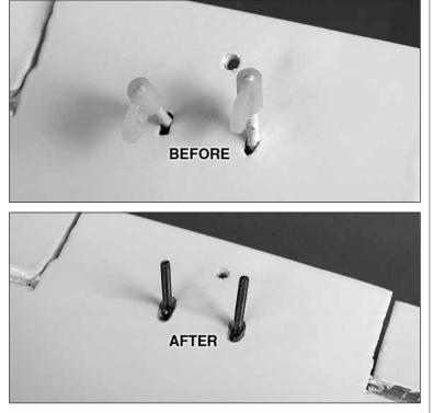
2. Use a #11 blade to cut excess paint from the holes in the bottom of the wing around the aileron torque rods. If you want to "go the extra mile," you can also remove the nylon torque rod horns and use a hobby blade and a Dremel<sup>®</sup> Moto-Tool with a wire brush to remove the paint from the torque rods.
