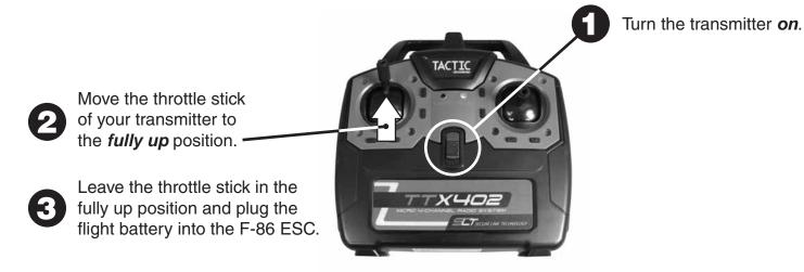
The LED on the ESC will illuminate solid red. Wait 4-5 seconds. The ESC will emit *ONE or TWO* high pitched beeps quickly.
