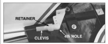
☐ 3. Verify that the **rudder** clevis is attached to the 4th hole from the inside of the rudder's control horn. Also, make sure that the silicone retainer is properly installed on the clevis.
