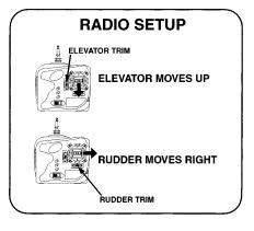
Center the surfaces using the trims on your radio transmitter. Use the sketch above to make sure the control surfaces are moving in the correct directions.
