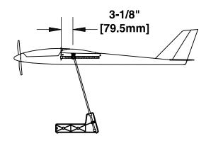
Note: This section is very important and must not be omitted! A model that is not properly balanced will be unstable and possibly unflyable.
