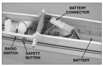
Turn the transmitter switch on. Install the motor battery in the airplane under the speed control and connect it to the receiver. Turn the receiver switch on. Mark the "ON" position of the switch. **Note:** The position of the receiver switch and safety button may vary slightly from what you see in the above image.
