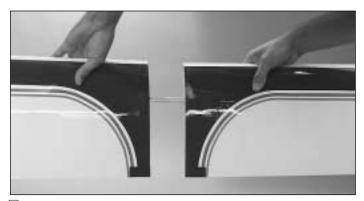
☐ 2. Insert the other side of the wing joiner into the left wing joiner pocket and slide the **wings** together.
