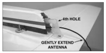
☐ 4. Completely undo any antenna knot. Gently extend the antenna and let it dangle freely out the end of the aft fuselage. Connect the elevator clevis to the elevator control horn at the 4th hole from the inside. **Note:** Never cut or shorten the antenna wire.
