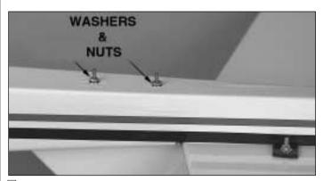
□ 2. The **fin** comes pre-installed on the Spectra Select, but you should check that the hex nuts are tight. Also, you should use some Great Planes Pro Threadlocker to prevent the nuts from coming loose.
