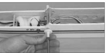
☐ 1. Install the wing dowels into the wing dowel holes as shown. Be sure that the smaller dowel (7mm x 90mm) should be installed into the aft holes. **Note:** The canopy was removed in this image for clarity.
