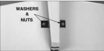
☐ 1. Find and open the holes in the stabilizer covering for the attachment bolts. Attach the **stabilizer** to the **fuselage** using two 2mm x 15mm bolts, two 2mm nuts and four 2mm washers. Use thread lock on the nuts to prevent loosening. **Note:** The fin was removed on these images for clarity.
