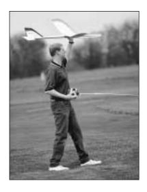
Turn on the transmitter first and then the receiver. Hold the SPECTRA SELECT under the wing with the nose pointed slightly down and directly into the wind. Do not run the motor for these test flights. It is very important that you launch the model
