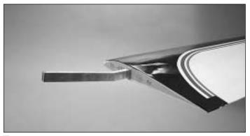
☐ 1. Locate the wing joiner and insert it into the right wing joiner pocket as shown in the above picture.
