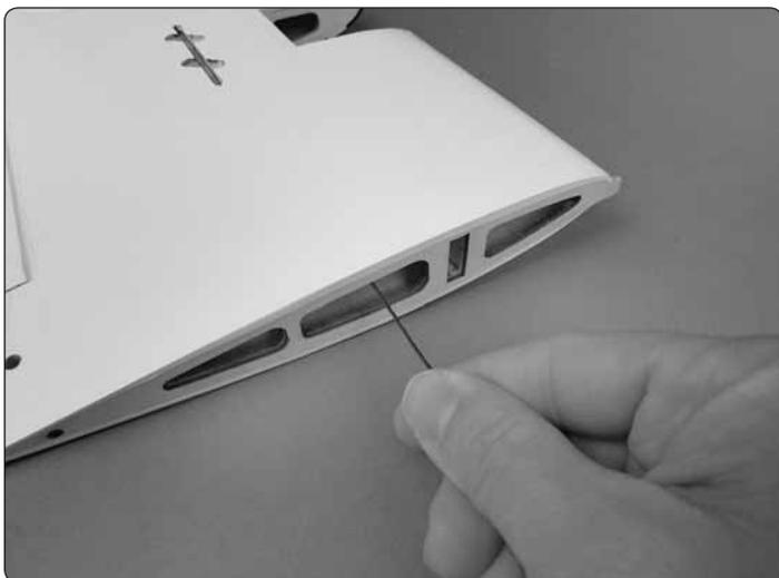
❑ 3. Pull the strings through the root ribs. Be careful not to damage the wing ribs as you pull the servo leads through them.
