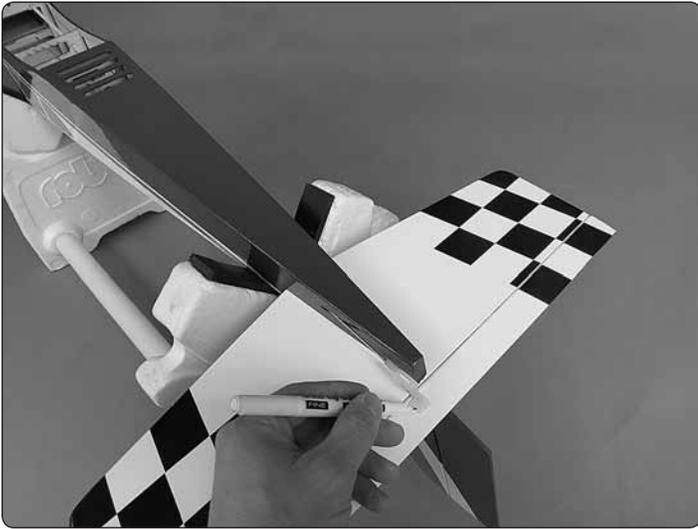
❑ 6. Thread a nylon clevis onto a 27" [685mm] pushrod. Attach the clevis to a control horn and slide the pushrod into the outer pushrod tube on the right side of the fuse. As you did with the ailerons, align the control horn over the elevator hinge line and mark the location of the screw holes. Drill 5/64" [2mm] holes at your marks and install the horn using two 2-56 x 3/8" [9.8mm] machine screws and the control horn backplate.
