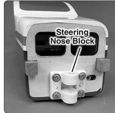
❑ 1. Mount the steering nose block onto the front of the fuselage using four 3x12mm machine screws, four 3mm flat washers and thread locking compound.
