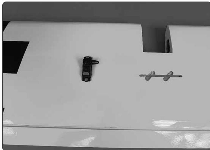
❑ 4. Fit the servos into the servo openings and drill 1/16" [1.6mm] holes through the mounting tabs on the servo cases into the rails. Thread a servo mounting screw (included with the servo) into each hole and remove it. Apply a drop of thin CA to each hole to harden the surrounding wood. When the CA has hardened, install the servos into the openings as shown using the screws supplied with the servos.
