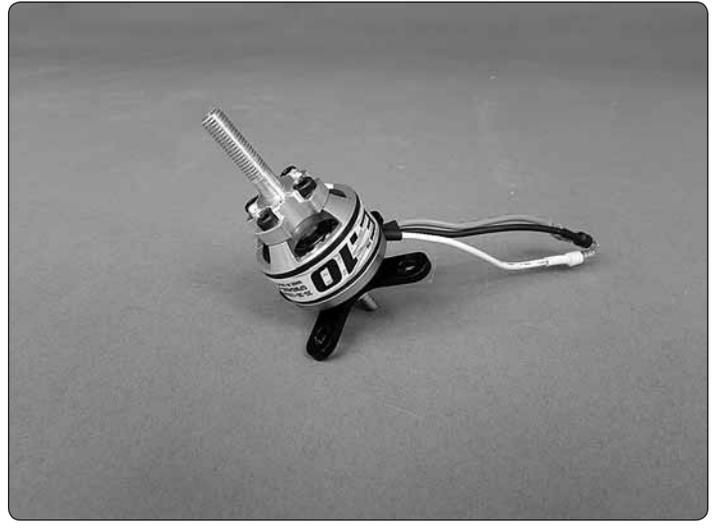
□ 11. Install the aluminum X-mount onto the motors using the screws included with the motors and thread locking compound. Install the prop adapters using the screws included with the motors and thread locking compound.
