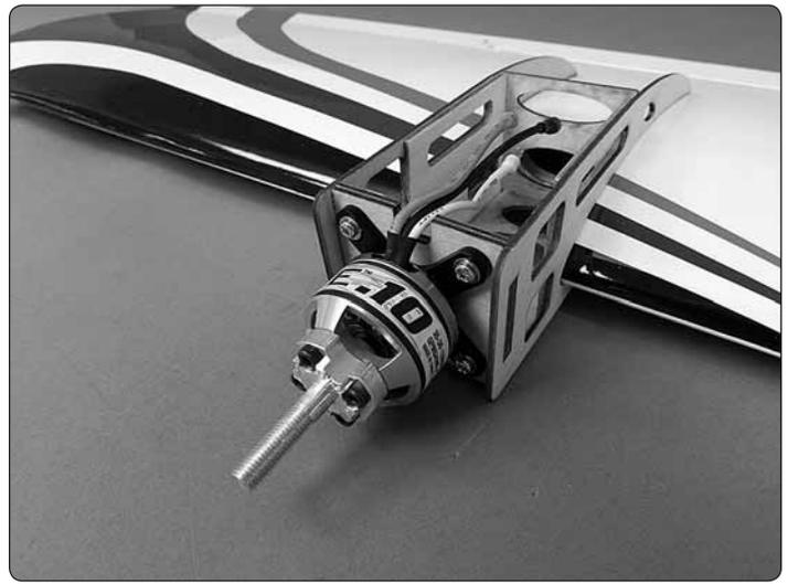
□ 12. Mount the motors to the nacelle firewalls using 3 x 12 mm machine screws, 3mm flat washers, and thread locking compound. Be sure that the motor leads are towards the top of the wing.
