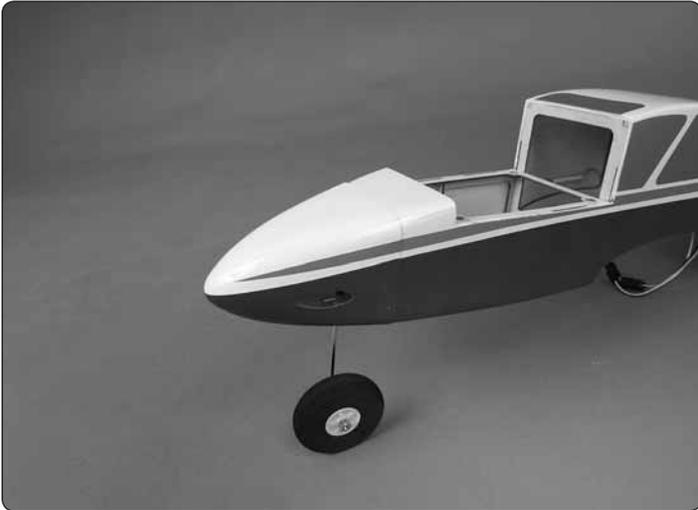
□ 13. Mark the location of the nose gear wire onto the nose cone when you hold it up in place. Use a rotary tool to cut a slot for the wire. The nose cone can be glued, screwed (screws not included) or taped on. We prefer using tape on this model because it allows easy access to the nose gear as well as looking better. If you decide to glue it on then we recommend RTV silicone.
