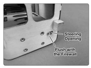
3. When the tube is flush with the firewall it is fully installed. Add medium CA to secure the tube to the formers and firewall (as shown).
