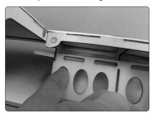
2. Use your index finger to lift the pushrod tube and slide it through the openings in formers 1, 2, and 3 so it extends to the servo tray.
