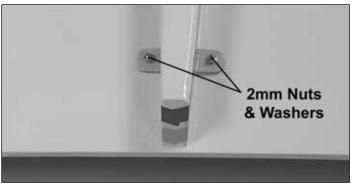
☐ 2. Find and open the holes in the **stabilizer** covering for the attachment screws. Attach the stabilizer to the **fuselage** using two **2mm x 15mm screws**, two **2mm nuts** and four **2mm washers**. Use thread lock on the nuts to prevent loosening. **Note:** The fin and rudder have been removed for clarity in the photo above.
