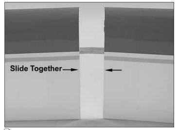
✓ 1. Check the fit of the wing joiner in the wing panels. Remove any excess material from the joiner to allow the panels to fit together. The joiner does not have to be glued into the wing. This will allow the wing panels to be separated for easier transportation.
