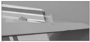
☐ 3. Attach the clevis in the second hole from the outside of the control horn. Trim the opening at the rear of the fuselage as necessary to allow the pushrod to move freely.
