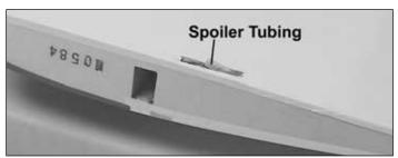
2. Pull the end of the spoiler tubing out of the wing just far enough to glue it in place using thick CA.
