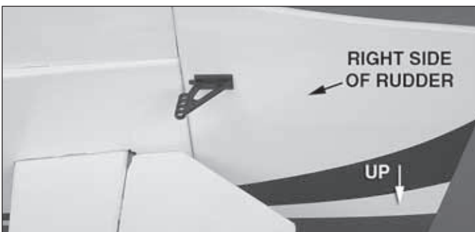
2. Install the other horn on the right side of the rudder.
