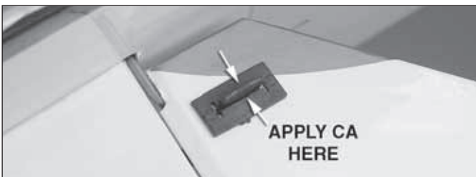
1. Locate two control horns and two horn retainers. Fit one horn to the bottom of the left elevator . Turn the model over and install a horn retainer onto the stud of the control horn. Apply one drop of medium CA to each side of the stud. You may trim off the tip of the stud after the glue has cured.
