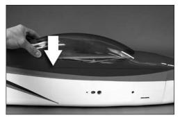
□ 2. Slide the aft end of the hatch down while aligning the hatch hook tabs in the slots in the fuselage.
