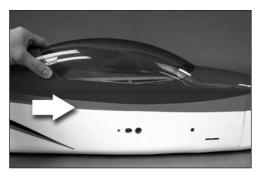
□ 3. With the aft end of the hatch fully seated, slide the hatch forward to engage the hatch hook tabs on the forward edges of the slots.
