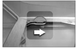
□ 4. Confirm that both hook tabs are locked into place in the fuselage.
