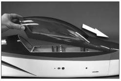
□ 1. Insert the canopy hatch pins into the holes in the firewall.
