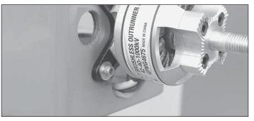
□ 4. Push the motor wires through the **cooling hole cutout** on the firewall as shown to prevent them from contacting the rotating motor case.
