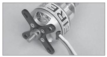
$\Box$  2. Install the brushless motor onto the aluminum **motor mount** (included with the motor) using four 3 x 8mm machine screws (included with the motor) and threadlocking compound.
