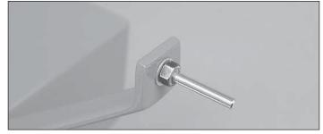
□ 7. Slide the axles through the landing gear brace as shown. Secure each axle with a #8 washer and 3/16" [5mm] nut. Be sure to use threadlocking cement.
