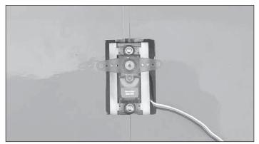
■ 8. Use your radio system to center the servo. Install the servo arm perpendicular to the servo case.
