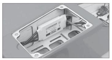
□ 5. Use hook and loop material or double-sided tape (not included) to secure the ESC to the side of the fuselage as shown. You may connect the motor wires at this time but leave them accessible in case you need to reverse the direction of the motor. Feed the receiver and battery leads on the ESC through the second former. Connect the receiver lead of the ESC to the receiver.
