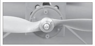
□ 11. Push the **spinner backplate** all the way onto the motor shaft. The center hole may be enlarged with a prop reamer or drill if necessary. Place the prop on the shaft so that it is perpendicular to the screw receptacles as shown. Finger tighten the prop nut and washer. Hold the prop shaft and tighten the prop nut securely with a prop wrench.
