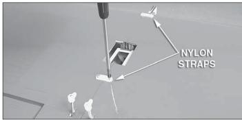
$\Box$  3. Fasten the wing halves together using the two included nylon straps and four #2 x 3/8" [9.5mm] self-tapping screws as shown.
