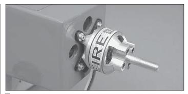
□ 3. Attach the brushless motor to the firewall using four  $4-40 \times 5/8$ " [15.9mm] hex head screws, four #4 flat washers and threadlocking compound. If you haven't done so already, install the prop adapter using the hardware included with the motor.
