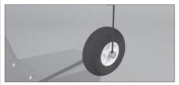
□ 8. Slide the main wheels onto the axles. Secure them in place by putting a 6-32 set screw in a 5/32" [4mm] wheel collar and tightening it down as shown. Use threadlocking cement on the set screw.
