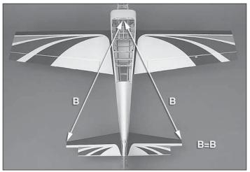
$\Box$  3. Measure the distance from the tip of the stab to the center of the fuselage. Adjust the position of the stab until they are equal. The stringer is centered in the front of the fuselage.
