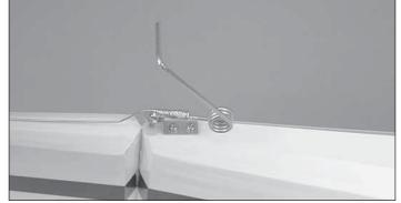
□ 2. Insert the tail gear wire through the aluminum tail gear bracket. Insert the tail gear wire and bracket in the tail gear bushing. With the tail gear bracket aligned with the bottom of the fuselage, mark and drill a 1/16" [1.6mm] pilot hole at both tail gear bracket mounting hole locations. Secure the tail gear bracket to the fuselage with two 2 x 12mm sheet metal screws.
