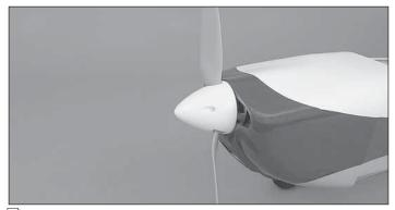
$\Box$  2. Use a prop reamer or drill bit to enlarge the spinner backplate to fit your motor's prop adapter. Install the spinner backplate, propeller with washer and prop nut and the spinner cone. Secure the spinner cone to the backplate with two 3 x 10mm sheet metal screws.
