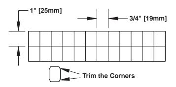
$\Box$   $\Box$  3. Cut six 3/4" x 1" [19 x 25mm] hinges from a CA hinge strip. Snip off the corners so they go in easier. Insert three hinges in each elevator.
