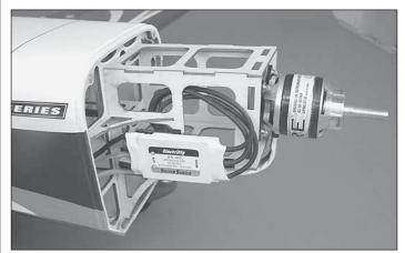
□ 2. Connect the ESC to the motor. The ESC can be attached to the side of the motor box with hook and loop material.
