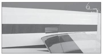
□ 1. Cut the covering away from the upper opening on the right side, in the rear of the fuselage for the rudder servo.
