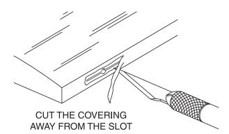
□ □ 2. Use a sharp #11 blade to cut a strip of covering from the hinge slots in the wing and aileron.
