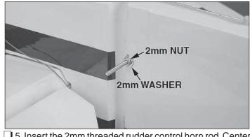
□ 5. Insert the 2mm threaded rudder control horn rod. Center the rod in the rudder with two 2mm flat washers and 2mm nuts on each side. A drop of threadlocker on the threads will help prevent the nuts from coming loose.
