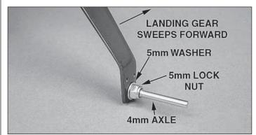
□ □ 1. Insert a 4mm axle through the right main landing gear. Secure the axle to the landing gear with a 5mm flat washer and 5mm lock nut. **Note:** The front of the main landing gear sweeps forward.
