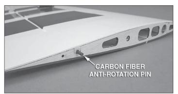
$\Box$  9. Glue the carbon fiber anti rotation pin in the hole as shown. The pin should protrude approximately 1/4" [6.4mm].
