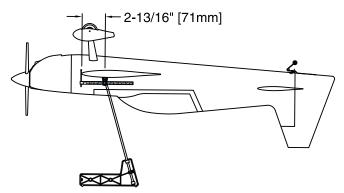
□ 2. With the wing attached to the fuselage, all parts of the model installed (ready to fly), lift the model at the balance point you marked.
