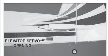
□ 1. Cut the covering away from the lower opening on the left side, in the rear of the fuselage for the elevator servo.
