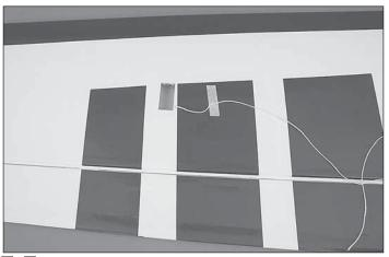
□ □ 1. Inside the servo bay a string is taped. Carefully remove the string from the servo bay and tape it to the outside of the wing to prevent it from dropping back into the wing. Test fit your aileron servo in the servo bay. Enlarge the opening if required.
