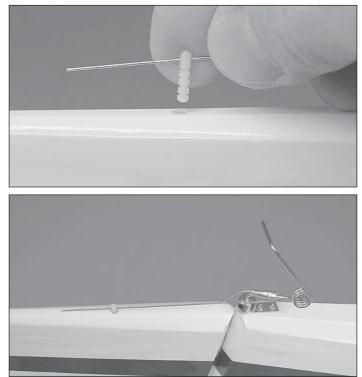
□ 3. Thread a 4-40 set screw into the 2.5mm wheel collar. Remove the tail gear wire from the tail gear bracket and position the 2.5mm wheel collar under the bracket. Slide the
