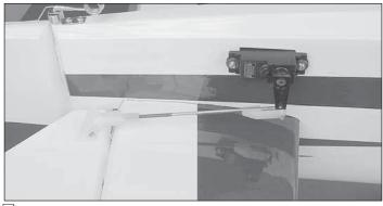
□ 5. Slide a silicone clevis retainer over the clevis. With the elevator servo and the elevator centered, mark the elevator pushrod where it crosses the elevator servo arm. Make a 90° bend at the mark. Cut the pushrod 3/8" [9.5mm] past the bend. Attach the pushrod to the elevator servo arm with a nylon FasLink.
