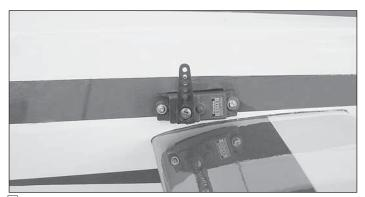
□ 3. Install the rudder servo into the servo opening. Drill through the servo mounting holes with a 1/16" [1.6mm] drill bit. Remove the servo from the servo opening. Install and then remove a servo mounting screw into each of the holes you have drilled. Apply a drop of thin CA into the holes to harden the threads. Once the glue has hardened install the servo into the servo opening using the 2 x 7 x 9mm servo retaining plates. Center the servo, and then install a servo arm as shown.
