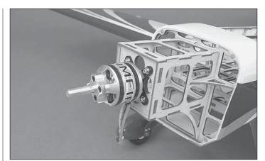
□ 1. Install the RimFire motor using four 4-40 x 1/2" [12.7mm] SHCS, four 3mm lock washers and four 3mm flat washers. Before installing, apply a drop of threadlocker to the threads of the SHCS.
