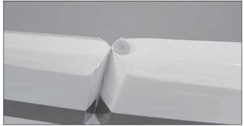
□ 1. Glue the nylon tail gear bushing in the hole in the aft bottom of the fuselage.
