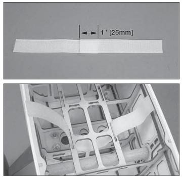
□ 8. Overlap by 1" [25mm] two strips of non adhesive backed hook and loop material. Route the hook and loop material
