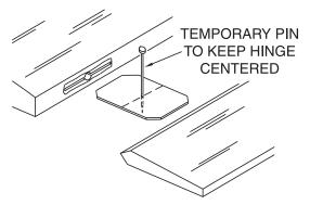
□ □ 4. Test fit the elevators to the stab with the hinges. If the hinges don't remain centered, stick a pin through the middle of the hinge to hold it in position.
