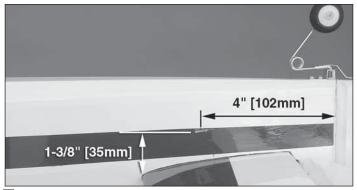
□ 2. Cut the covering from over the two pull-pull exits at the aft end of the two servo openings, between the openings.
