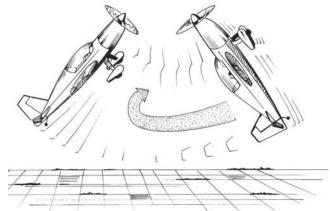
With the model pointing vertically (almost in a hover), push full down elevator and full throttle. As the model rotates and begins to point downwards, reduce the throttle (to keep the model from being pulled downwards). As the model flattens out, add power to pull the model around. Many models will require some rudder correction (usually right rudder) during this maneuver. Some planes will require aileron correction to keep the wings level.
