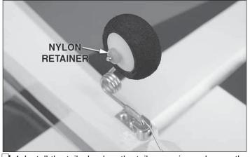
□ 4. Install the tail wheel on the tail gear wire and press the silicone retainer on the tail gear wire to secure the tail wheel.
