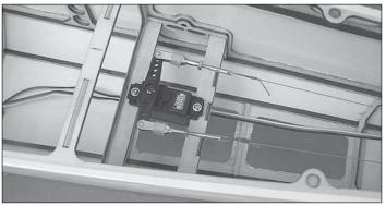
$\Box$  9. Attach the clevises to the rudder servo horn in the holes 3/4" [19mm] from the center.
