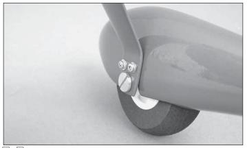
$\Box$  3. Position the right wheel pant over the wheel and secure it to the main landing gear with two 2-56 x 3/8" [9.5mm] machine screws, 2mm flat washers and 2mm lock washers.
