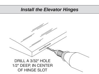
□ □ 1. Drill a 3/32" [2.4mm] hole, 1/2" [12.7mm] deep in the center of each hinge slot to allow the CA to "wick" in. Follow-up with a #11 blade to clean out the slots. **Hint:** If you have one, use a high-speed rotary tool to drill the holes.
