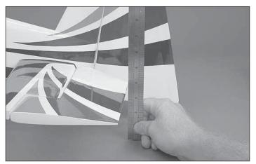
Use a ruler to accurately measure and set the control throw of each control surface as indicated in the chart that follows. If your radio does not have dual rates, we recommend setting the throws at the **low rate** setting.
