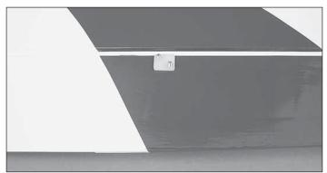
$\Box$   $\Box$  7. Insert two 2-56 x 5/8" [16mm] machine screws through the control horn and aileron. Secure the control horn to the aileron with the nylon control horn backplate.
