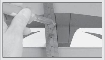
Use a straightedge to guide the soldering iron at a rate that will just melt the covering and not burn into the wood. The hotter the soldering iron, the faster it must travel to melt a fine cut. Peel off the covering.
