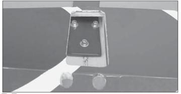
$\Box$  4. Attach the main landing gear to the fuselage with three 4-40 x 1/2" [12.7mm] SHCS, 3mm lock washers and 3mm flat washers.
