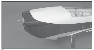
□ 1. The cowl is held on with four magnets. It fits over the small lip and snaps into place. **Note:** If you will be performing violent maneuvers, a piece of clear tape should be applied to both sides of the cowl to help hold it in place.
