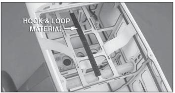
□ 9. Attach a strip of sticky backed hook material to the center of the battery tray. The loop material can be attached to the battery.
