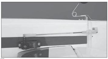
□ 5. Slide a silicone clevis retainer over the clevis. With the rudder servo and the rudder centered, mark the rudder pushrod where it crosses the rudder servo arm. Make a 90° bend at the mark. Cut the pushrod 3/8" [9.5mm] past the bend. Attach the pushrod to the rudder servo arm with a nylon FasLink.
