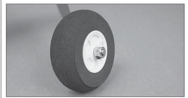
$\Box$  2. Install two 5mm flat washers on the axle, then the foam main wheel, followed by a 4.2mm wheel collar. Secure the wheel collar on the axle with 6-32 set screw. Mark the
