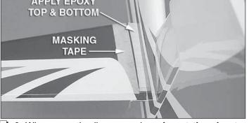
□ 6. Wipe away the lines you drew. **Insert the elevator joiner wire in the notch at the back of the stab saddle.** Use epoxy to glue the stab in place, being careful that the stab is properly aligned.
