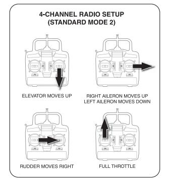
□ 3. Make certain that the control surfaces and the throttle respond in the correct direction as shown in the diagram. If any of the controls respond in the wrong direction, use the servo reversing in the transmitter to reverse the servos connected to those controls. Be certain the control surfaces have remained centered. Adjust if necessary.
