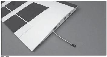
□ □ 3. Tie the string to the servo extension. Pull the string and the servo lead through the wing. Untie the string from the lead.
