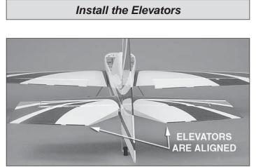
□ 1. Install the elevators onto the stab with the elevator joiner wire in each elevator half. Check that both elevator halves are aligned. If not, remove the elevators and while holding one leg of the elevator joiner wire, slightly bend the other. Reinstall the elevator halves and check again.
