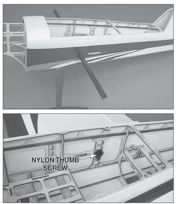
□ 1. Center the wing tube in the fuselage. Slide the wing halves onto the wing tube and secure the wing halves to the fuselage with the nylon 10-24 thumb screws. Be careful putting pressure on the wing and fuselage. The wings may be tight the first time they are slid on the tube.
