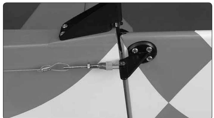
12. Attach the clevises to the control horns and pull the cables tight. Crimp the brass tubes with pliers.
