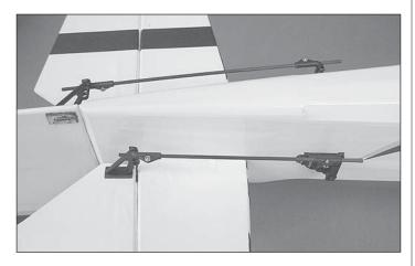
4. Install the elevator pushrod in the same manner using the remaining 6-3/4" [170mm] pushrod. Use some diagonal cutters or a rotary tool to trim the pushrod so that it extends 1/2" [13mm] past the clevis.
