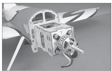
4. Once the epoxy has had plenty of time to cure, remove the tape and install the motor using the "X" shaped mount provided with the motor. Secure the motor to the motor mount with four 3 x 8mm machine screws and 3mm washers. Do not forget to use threadlocking compound when installing the "X" mount to the motor and when installing the motor to the airplane.
