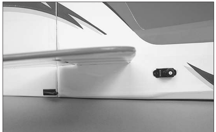
❑ 2. Attach a 12" [305mm] slim servo extension to the elevator and rudder servos. Use your radio system to center the servos. Before installing the servos, test fit double-sided servo arms to determine which arm is closest to perpendicular with the tail servo case sides. Cut off the arm that is not used. If neither of the servo arms are close to perpendicular with the servo case sides, locate the single-sided servo arm and check it. Secure the servos in the servo bays with the splines facing forward. If using CA glue to mount the servos, do not forget to trim the covering so that the servo mounting tabs can be glued directly to the wood underneath.
