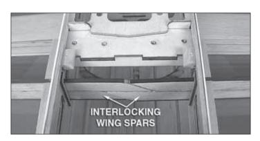
The design of the interlocking wing spars has changed slightly to make alignment much easier and quicker. Use this photo when performing step #2 on page 9 of the manual. This change will not affect the procedure for gluing the wing panels to the fuselage as described in step #3 on page 10 of the manual.
