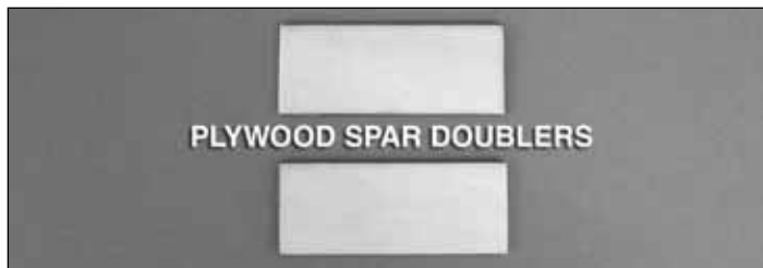
SPAR DOUBLERS GLUED TO FRONT AND BACK OF WING SPARS
