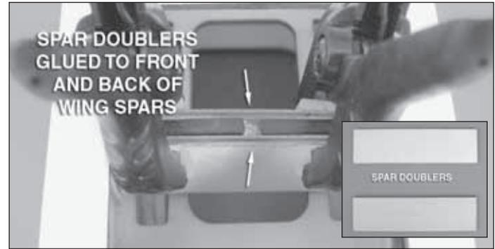
Step #6 on page 10 of the manual shows a single balsa spar doubler. Two spar doublers are now included instead of just one, and they are made of plywood instead of balsa. Coat one side of each spar doubler with epoxy as well as the front and back sides of the spars. Position a spar doubler on each side of the spars as shown and use clamps to hold them in place while the epoxy cures.
