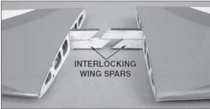
The design of the interlocking wing spars has changed slightly to make alignment much easier and quicker. The procedure in the manual on pages 9 and 10 for gluing the wing panels into the fuselage remains the same.
