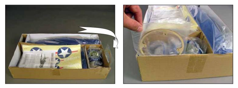
The cowl ring for the Combat Corsair ARF is located in the packaging between the inner cardboard insert and the lower cardboard box.
