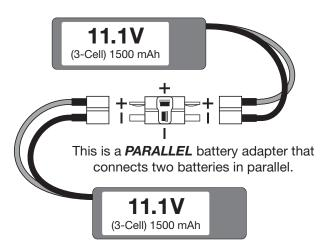
2. Connecting batteries in "Parallel" means to connect the +'s to the +'s and the -'s to the -'s. This combines the battery's capacities, but the Voltage remains the same.
