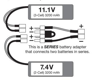
1. Connecting batteries in "Series" means to connect the +'s to the -'s and the -'s to the +'s. This combines the battery's Voltages, but the capacity remains the same.
