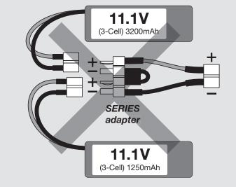
Also **NEVER** connect battery packs with different capacities in Series or in Parallel.
