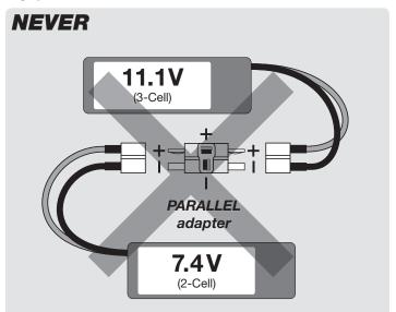
**NEVER** connect battery packs with different Voltages in **Parallel**–only combine in **Series**. Otherwise, the batteries will try to "equalize" with the larger one trying to "charge" the smaller one, thus causing heat and likely a fire.
