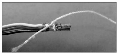
Once the lead is pulled through the wing, reinstall the pins to the connector in the same order as removed. Failure to properly reinstall the wires to the connector can result in damage to equipment or even fire.
