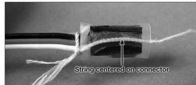
Locate the string at the center section of the top wing. You may need to trim the two small openings to locate the string. Once located, gently pull a small portion of the string through the center section. Note: The string extends through the entirety of the top wing and is intended to be used during installation of both aileron servo leads.
