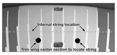
Next, feed the connector and string through the hole in the rib near the aileron servo compartment. Gently pull the string at the center section through the hole located on the same side of the wing as the aileron servo lead you're pulling through. Once the lead is at the opening at the center section, pull the connector through the hole. If you are unable to pull the aileron servo extension through the wing skip to section below.
