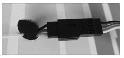
Once the lead is pulled through the opening, attach one end of the Y-harness. Use the included heat shrink to secure the extension to the Y-harness. While heating the heat shrink material be careful not to damage the covering on the aircraft.
