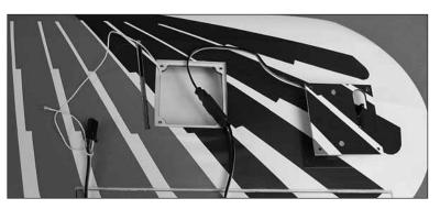
Getting the lead through the opening in the rib may require trimming a portion of the servo lead.
