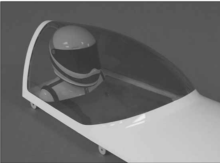
❑ 2. On the bottom of the pilot are two holes and inside the pilot there are blind nuts to secure the pilot. Align the holes on the bottom of the pilot with the holes located at the back of the cockpit. Secure the pilot to the cockpit with 4-40 x 1/2" [12.7mm] machine screws, #4 flat washers and #4 lock washers.
