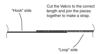
□ 14. Locate the non-adhesive backed hook and loop material. Make two sets of straps for your receiver and battery by joining a piece of non-adhesive backed "hook" material to a piece of "loop" material.
