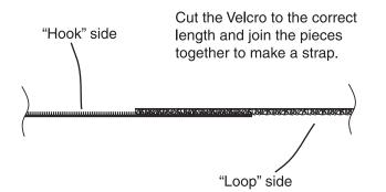
□ 22. Cut two 5" [127mm] strips of non-adhesive backed hook and loop material. Make two sets of straps for your ignition unit and ignition battery by joining a piece of "hook" material to a piece of "loop" material.
