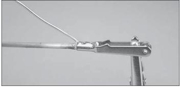
□ □ 4. Use a hobby torch to heat both the clevis and the pushrod. Apply silver solder to the joint. The heat of the clevis and the pushrod should melt the solder, not the direct flame of the torch.
