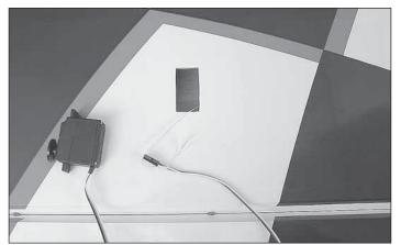
□ □ 3. Starting with the outboard servo bay, tie the guide string to the 24" [610mm] servo lead extension. Pull the extension through the wing.
