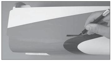
□ 6. Trim the covering from the main landing gear slots in the fuselage.
