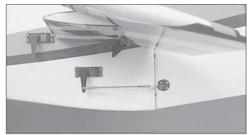
□ 6. Install a 4-1/2" [114mm] pushrod to the rudder servo and rudder. The pushrod should be installed on the servo arm so that it is 1-1/4" [32mm] out from the center of the servo arm and in the outermost hole of the control horn. Turn on your radio and center the rudder by adjusting the clevis.
