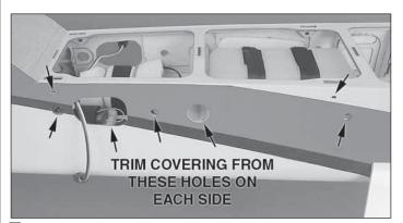
□ 1. Trim the covering from the fuselage sides in the following locations: four canopy screw holes, two wing tube holes, four wing bolt holes, two TE wing dowel holes, and two servo wire holes.
