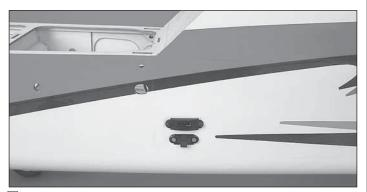
□ 4. Trim the covering from over the switch plate holes and install the ignition switch and charge jack.
