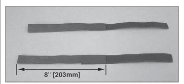
□ 32. Cut two 8" [203mm] strips of hook and loop material. Join each "hook" side to each "loop" side with a 2" [51mm] overlap.
