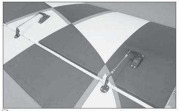
□ 5. When you're done installing all of the control horns, adjust the length of your pushrods using the threaded clevis and attach them to the control horns. Tighten the lock nuts and position the silicone retainers after you have centered the flight controls.
