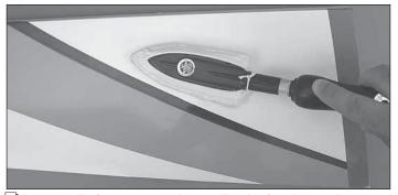
Lay out all of your covered parts like the fuselage, wings, and control surfaces. Inspect the covering for wrinkles and peeled edges. Use a covering iron set for low to medium/high heat and tack down the covering. Medium heat may be necessary to stretch out any wrinkles, but be careful not to apply too much heat to areas where covering is applied over covering.
