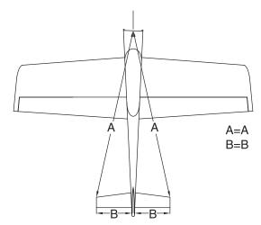
□ 2. Slide the stab into the fuselage. Center it from left to right and fore and aft, making sure that the distances are equal.
