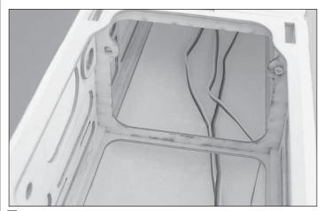
□ 4. Fit your rudder and elevator servos in place. Route the wires under the formers as shown.
