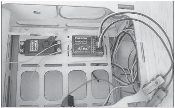
□ 15. Connect a Y-connector to each aileron channel. Connect the other servo leads and the battery switch to your receiver.
