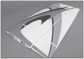
□ □ 9. Use masking tape to hold the aileron snug up against the hinge line. Set the wing aside and allow the epoxy to fully cure before you remove the tape or move the ailerons.
