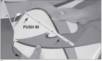
□ 5. Install both elevators. Push each one up against the hinge line. Deflect them up and down so that the hinges align properly. Use tape to hold the elevators level and up against the hinge line like you did with the ailerons.
