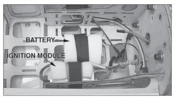
□ 23. Wrap your ignition module in 1/4" [6.4mm] thick R/C latex foam rubber. Mount the ignition module to one of the uprights or to the forward compartment floor using one of the straps that you made.
