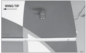
□ 1. Use your radio to center your aileron servos. Attach a 1-1/2" [38mm] single-sided servo arm (GPMM1105) to each servo so that the arm is parallel with the hinge line when the servo is centered. Install the arms so that they point outward toward the wing tip.
