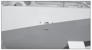
□ 20. Trim the covering from over the switch plate holes and install the ignition switch and charge jack.
