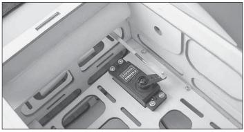
□ 10. Install a servo arm. Set your throttle servo to the fullthrottle position and connect the pushrod.
