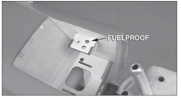
□ 19. Turn the model over. Use epoxy to glue the fuel filler mount to the exhaust tunnel. Use sandpaper to roughen the surface of where the fuel filler mount will adhere to.
