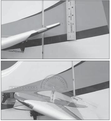
Use a ruler, an inclinometer, or a protractor to accurately measure and set the control throw of each control surface as indicated in the chart that follows. If your radio does not have dual rates, we recommend setting the throws at the **high rate** setting.
