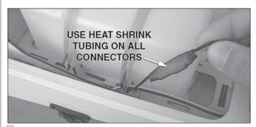
■ 8. Connect the battery to the switch and the switch to the radio. Use heat shrink tubing to secure the connection between the battery and the switch.
