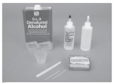
□ 1. You will need the following supplies: Denatured alcohol, 30-minute epoxy, epoxy mixing cups, mixing sticks, round toothpicks, petroleum jelly, masking tape, and some paper towels.
