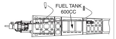
$\Box$  8. Locate the wood pushrod standoffs. Fit them to the gray outer pushrod tube and install the tube. Route it clear of the bellcrank and around the fuel tank. Trim the tube to fit and test fit the standoffs.
