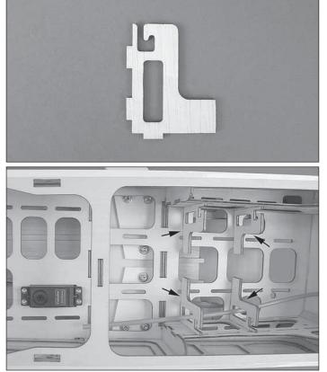
□ 7. Dry-fit the fuel tank supports and route the plastic outer pushrod tube from the firewall to the servo.
