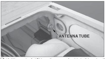
□ 18. We used a 2.4GHz radio system for this build-up, but if you're using a 72MHz radio system an antenna routing tube is provided for you in the upper left side of the fuselage.
