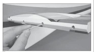
□ 3. Thoroughly coat the hinge pockets and the tips of each hinge with 30-minute epoxy.
