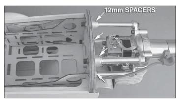
□ 6. Obtain four  $1/4-20 \times 1-1/2$ " [38mm] SHCS, four 1/4" [6.4mm] lock washers, and four 1/4" [6.4mm] washers (not included). Locate the four included 12 x 20mm aluminum spacers. Install the engine to the firewall using threadlocking compound on the threads of the bolts as an added safety measure.
