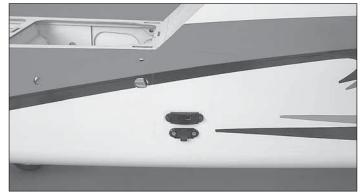
□ 5. Trim the covering from over the switch plate holes and install the switch and charge jack. Iron the covering to the switch plate before you begin trimming.
