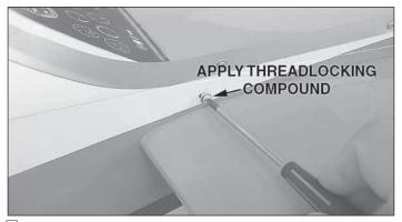
□ 4. Fit the canopy hatch to the model and use four 4-40 x 5/8" [16mm] Phillips head screws, four #4 lock washers, and four #4 washers. Apply a drop of threadlocking compound to the screw threads periodically so that you don't lose these screws in flight.
