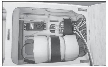
□ 16. Wrap your receiver and battery pack with 1/4" [6.4mm] thick latex foam. Use the straps you made to mount your battery and receiver to the aft equipment tray.
