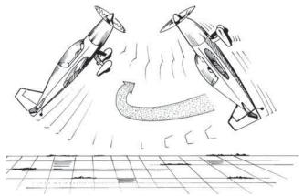
With the model pointing vertically (almost in a hover), push full down elevator and full throttle. As the model rotates and
