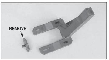
□ 4. Break the tangs out of each molded engine mount half and grind off any remaining portion.
