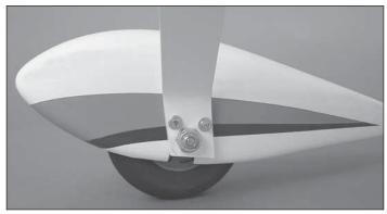
□ 8. Attach the wheel pants to the landing gear legs using four 4-40 x 1/2" [13mm] SHCS, four split ring lock washers, and four #4 washers. Use threadlocking compound on the screw threads.
