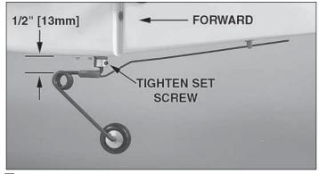
■ 8. Adjust the tail gear's position in the main bushing so that the tail gear wire is 1/2" [13mm] from the bottom of the fuselage. Use threadlocking compound on the set screw and tighten the collar.
