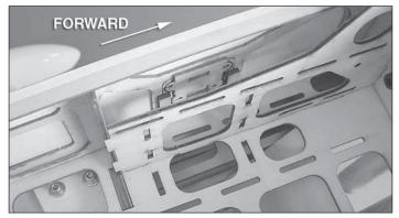
□ 18. Install the switch plate on the model using epoxy to attach it. There are two forward locations reserved for the gas engine's ignition module. We chose the one on the left side.
