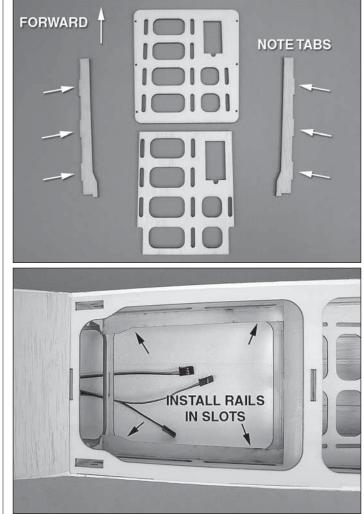
□ 5. Locate the aft equipment tray, the tray doubler and the two side rails. Glue the tray doubler to the bottom of the tray. Align the tabs on each rail with the corresponding slots in the fuselage and glue each rail in place as shown.
