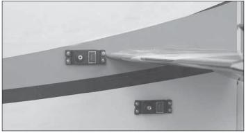
5. Install the elevator and rudder servos. Use a 1/16" [1.6mm] drill bit to drill the holes and use thin CA to harden the wood.
