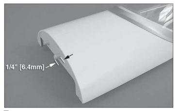
□ 1. Locate the two 1" [25mm] wooden dowels and glue them into the canopy so that they are 1/4" [6.4mm] from the front face of the former.
