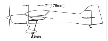
□ 2. With the wing attached to the fuselage, all parts of the model installed (ready to fly) and an empty fuel tank, place the model on a Great Planes C.G. Machine, or lift it at the balance point you marked.
