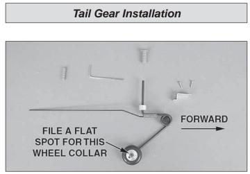
□ 1. Locate the tail gear assembly. Remove the wheel collar and file a flat spot on the axle where the set screw contacts the axle. Apply threadlocking compound to the wheel collar set screw and reinstall it.
