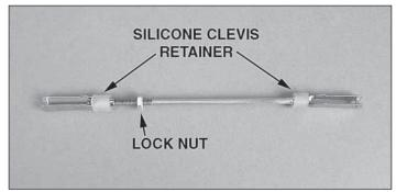
□ □ 7. Fit a silicone retainer onto the rod, a 4-40 hex nut, another silicone retainer, and a 4-40 threaded clevis onto the rod in that order. The threaded end of your pushrod should look like the picture above.
