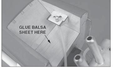
□ 20. Test fit the covered balsa sheet as shown. The sheet is not "square." It matches the angle of the firewall. **Note:** One side has clear covering which must face outward.
