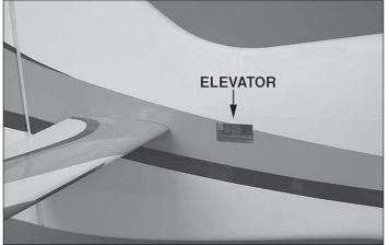
□ 1. Trim the covering from the elevator servo bay on the right side of the fuselage as shown.
