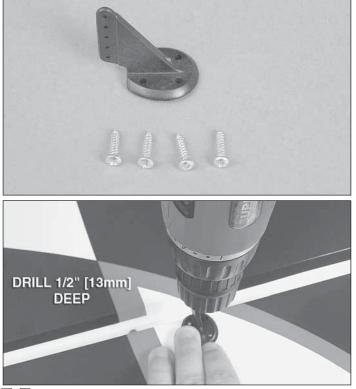
□ □ 3. Center a control horn over the line that you made, making sure that the clevis holes are also centered over the hinge line. Hold the horn in position and use a 1/16" [1.6mm] drill bit to drill four 1/2" [13mm] deep holes in the aileron. You can wrap a piece of tape around the drill shank to help keep you from drilling the holes too deep.
