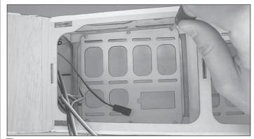
□ 6. Position the aft equipment tray in the aft bay and use a 1/16" [1.6mm] drill bit to drill six pilot holes through the side rails. Harden the holes with thin CA. Use six #2 x 3/8" sheet metal screws with six #2 washers to attach the aft equipment tray.
