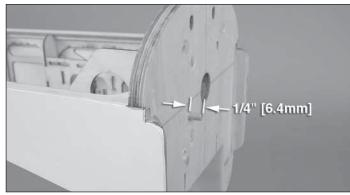
□ 5. Cut a 1" [25mm] piece of outer pushrod tubing from the 36" [914mm] length supplied. Install it in the firewall as shown so that 1/4" [6.4mm] of the tube protrudes forward from the firewall. Roughen the surface with sandpaper and use epoxy to glue it in place.
