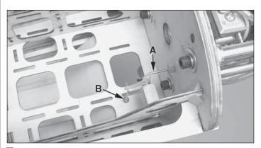
□ 12. Loosely position the bellcrank assembly as shown and connect threaded pushrod A and pushrod B as shown. Apply
