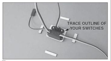
□ 1. Locate the switch plate that fits your brand of radio switch. Four plates are supplied: two Futaba switch & Ernst charge jacks and two Hobbico heavy-duty & Ernst charge jacks. Fit your switch and charge jack to the plate and use a pen or pencil to draw an outline of the switch and jack onto the back side of the plate. Remove the switch and charge jack.
