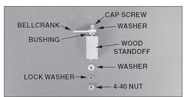
□ 11. Locate one 4-40 x 1-1/2" [38mm] cap screw, one #4 lock washer, two #4 washers, one brass bellcrank bushing, one 4-40 nut, and one 1/2" x 1/2" x 1" [13 x 13 x 25.4mm] pre-drilled wooden standoff block. Fit the bellcrank parts in the order shown.
