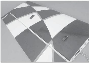
$\Box$   $\Box$  5. Install the aileron servos using the screws provided with your servos.
