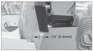
■ 8. Trim the plastic pushrod tube so that there is at least 1/4" [6.4mm] of tube protruding forward of the firewall and that there is approximately 1-1/2" [38mm] of distance between the throttle servo output shaft and the tube. When you're satisfied with the fit of the pushrod tube, epoxy the fuel tank supports in place. Roughen the outer surface of the pushrod tube and epoxy it in place.
