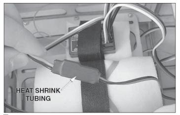
□ 11. Connect the battery to the switch. Use heat shrink tubing to secure the connection between the battery and the switch.
