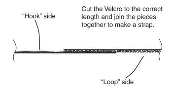
□ 6. Locate the non-adhesive backed hook and loop material. Make two sets of straps for your receiver and battery by joining a piece of "hook" material to a piece of "loop" material.
