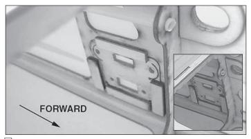
□ 2. Install the ignition switch plate on the model using epoxy. A cutout for the switch plate is provided in the left and right rear fuselage. You may choose either location.
