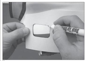
$\Box$  7. Fit the cowl to the plane so that the cowl centering tool bottoms out on the engine's drive washer. Position the paper template and trace the muffler cutout onto the cowl using a felt-tip pen.
