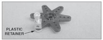
□ 9. Install a screw-lock pushrod connector onto a short servo arm. Use a plastic retainer to hold this to the servo arm and a 4-40 x 1/4" [6.4mm] SHCS. Turn on your radio and position the servo arm. Install the arm to your throttle servo using the servo screw supplied with your servos.
