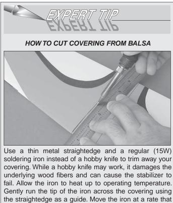
melts the covering but does not burn the wood fibers. A few gentle passes are preferable to slower passes that can damage the wood.
