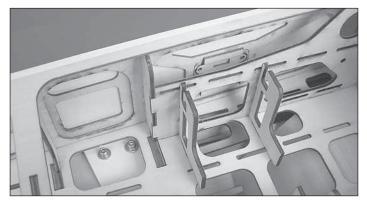
□ 3. Install the switch plate on the model using epoxy to attach it. There are six places to mount the switch plate, so choose the one that suits you best.
