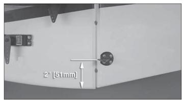
□ 5. Make a line 2" [51mm] from the bottom edge of the rudder. Drill the holes for the rudder horn and install it with four #4 x 1/2" [13mm] sheet metal screws.
