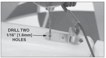
$\Box$  4. Fit the tail gear assembly into the bushing and fit the tail gear retainer to the fuselage bottom as shown. Drill two 1/16" [1.6mm] holes into the fuselage using the retainer as a guide. Remove the tail gear assembly.
