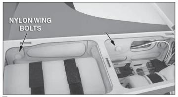
$\Box$  3. Pull the aileron servo leads into the fuselage and install the wings using four 1/4" x 1" [6.4 x 25mm] nylon wing bolts. Connect the aileron servo leads to the Y-harnesses on your receiver.
