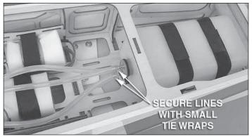
□ 33. Fit fuel lines to the tank and install it using the two straps you made. Route the fuel feed line to the carburetor. Use small tie wraps to secure the fuel lines to the lines on the tank.
