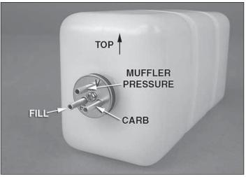
□ 16. Finish assembling your tank and tighten the stopper screw. Be careful not to overtighten the stopper. This can split the tank along the seam.
