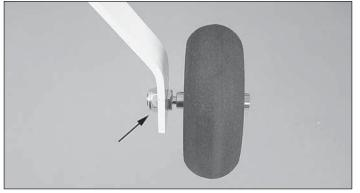
□ 5. Attach the axles to the main landing gear legs using the self-locking axle nut.
