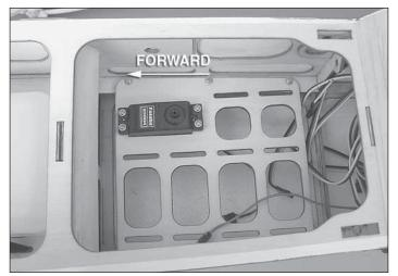
□ 7. Install the throttle servo in the aft tray. Drill four 1/16" [1.6mm] holes and harden them with thin CA. Note the position of the servo output shaft.
