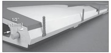
□ □ 2. Start with the right wing and aileron. Install one 1-3/8" [35mm] anti-rotation dowel in the location shown using epoxy.
