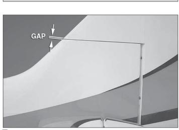
□ 1. Test fit the rudder using the four remaining hinges. Check for free rudder movement and a visible gap between the tip of the fin and the rudder counterbalance.
