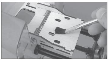
□ 7. If your ESC must be held on with double-sided tape, mix up some epoxy and thin it down with denatured alcohol. Coat the bottom surface of the ESC tray. Allow the epoxy to cure.
