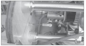
□ 13. Thread a 2-56 nylon ball link socket onto **pushrod A** as shown and attach it to the choke arm.
