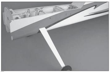
□ 7. Use six 6-32 x 5/8" [16mm] SHCS, six #6 split ring lock washers, and six #6 washers to attach the landing gear to the fuselage. Use threadlocking compound on the screws. **Note:** The landing gear is swept back.
