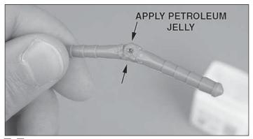
□ □ 4. Remove the aileron and the hinges. Prepare each hinge first by cleaning off any mold release compound left on the parts during manufacture. Use denatured alcohol for this. Prepare each hinge for gluing by thoroughly coating the center section with petroleum jelly.
