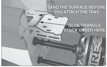
□ 6. Use 80-grit sandpaper to roughen up the coated surface of the firewall and the equipment tray where the ESC tray will mount. Use epoxy to bond the ESC tray to the fuselage as shown. A piece of triangle stock is supplied to help secure the tray to the firewall.
