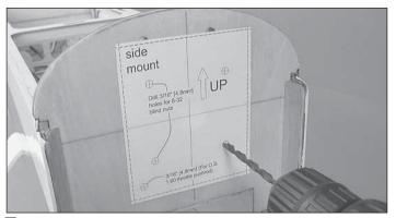
□ 1. Turn to the back of this manual and cut out the drilling template for the engine you're using. Center the template by matching the template crosshairs with the firewall crosshairs.
