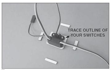
□ 16. Locate the switch plate that fits your brand of radio switch. Four plates are supplied: two Futaba switch & Ernst charge jacks and two Hobbico heavy-duty & Ernst charge jacks. Fit your switch and charge jack to the plate and use a pen or pencil to draw an outline of the switch and jack onto the back side of the plate. Remove the switch and charge jack.
