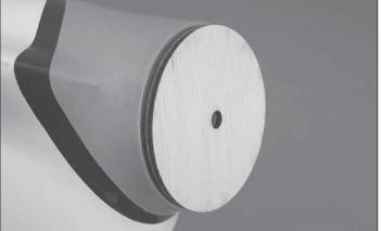
$\Box$  6. Fit the cowl centering tool to the cowl as shown. Use only two small drops of medium CA to tack the inside and the outside pieces together so that you can remove them easily later.
