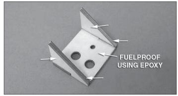
□ 14. Locate the wood parts and build the fuel filler mount as shown. Fuelproof the filler mount with a thin layer of epoxy.
