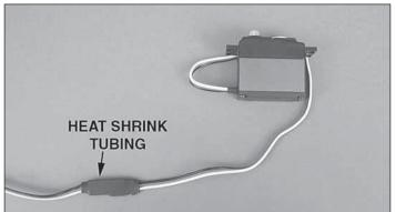
□ 3. Attach a 36" [914mm] servo lead extension to the three tail servos. If you anticipate mounting your receiver in the aft-most equipment tray, you may use shorter servo lead extensions.
