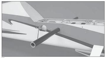
2. Locate the 24-1/2" [620mm] wing tube and slide it into the fuselage.
