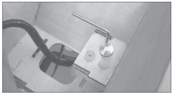
□ 34. Route the vent and fill lines through the fuel filler mount and install a fuel filler plug.
