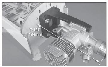
□ 5. Fit the two engine mount sides together. Center the engine mount with the cross-hairs on the firewall and fit the mount to the firewall using four 8-32 x 1-1/4" [32mm] SHCS, four #8 lock washers, and four #8 washers. Leave the screws loose enough to adjust the width of the mounting
