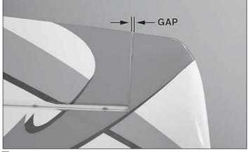
□ 1. Test fit eight hinges in the stab and then fit the elevators. Check for free movement of the elevators and that there is a visible gap between the tip of the stab and the elevator counterbalances. If the counterbalance interfers with the stab, you should remove the covering from the tip of the stab and sand off enough material until you get a good fit You'll have to re-cover the area of wood you exposed. **DO NOT attempt to re-drill the hinge holes!**
