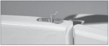
□ 5. Use the two 8mm sheet metal screws to attach the retainer to the fuselage.
