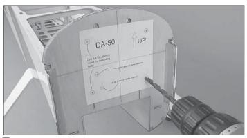
□ 3. Turn to the back of this manual and cut out the drilling template for the engine you're using. Center the template by matching the template crosshairs with the firewall crosshairs. Tape it in place and use a 1/8" [3.2mm] drill bit to drill four engine mount pilot holes in the firewall. A center punch or scratch awl can be used to make a centering mark before you drill. Follow up with a 1/4" [6.4mm] drill bit and enlarge the holes.
