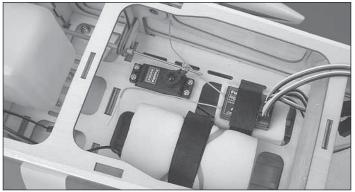
□ 9. Wrap your receiver and battery pack with 1/4" [6.4mm] thick latex foam. Use the straps you made to mount your battery and receiver to the center equipment tray.
