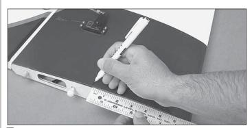
□ 1. Using a black felt-tipped pen, make a mark on the bottom of each wing that is 7" [178mm] from the LE of the root wing rib. This is the ideal balance point and this is where your plane should balance for the first few flights. If you wish to experiment with the C.G., you may do so after you have become comfortable with the plane. The forward C.G. limit is 6.5" [165mm] from the LE of the root rib. The aft limit is 8" [203mm] from the LE of the root rib.
