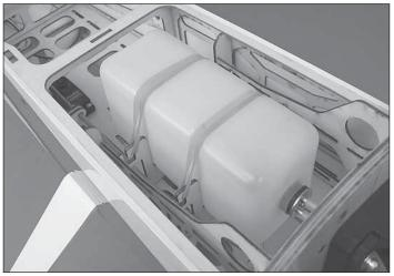
□ 17. Fit fuel lines to the tank and install it using two #64 rubber bands. You may test fit your muffler at this point and trim the vent line to length.
