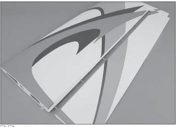
□ □ 3. Fit the aileron tightly up against the wing and deflect it up and down a few times checking for binding.
