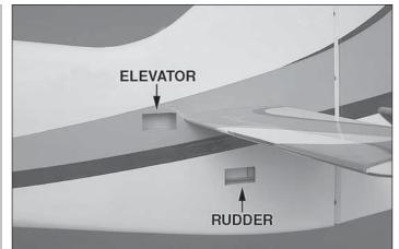
□ 2. Trim the covering from the elevator and rudder servo bays on the left side of the fuselage.
