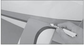
□ 3. Holding the stab in position, use a fine-point, felt-tip marker to trace lines onto the stab. Don't forget to trace lines on the bottom side of the stab, too.
