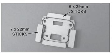
$\Box$  2. Use two 7 x 22mm and two 6 x 29mm sticks to make a flange for the charge plate.
