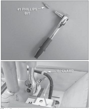
□ 26. Turn the model over. Wrap a tie wrap around the spark plug lead to make a "P" clamp. Route the spark plug lead in a fashion that keeps it away from the muffler. Use a spare servo screw to attach this to the side wall of the exhaust box. Since a screwdriver won't fit, we suggest using a 1/4" [6.4mm] socket with a #1 Phillips bit.
