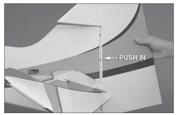
□ 3. Use 30-minute epoxy to glue your hinges in place. Remember to align them and to deflect the rudder both ways when you install it.
