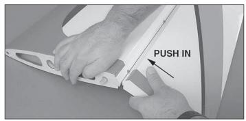
□ □ 7. Fit the hinges into the wing, making sure that you align each one. Fit the aileron tightly and deflect it a few times in both directions. This will straighten any hinges that are slightly out of alignment.
