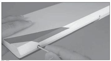
□ □ 5. Mix up a batch of 30-minute epoxy and use a toothpick to generously coat the inside of each hole or "pocket." Apply epoxy to both the wing pockets and the aileron pockets. **Warning:** This glue joint is critical and you must take the time to ensure it is done properly.
