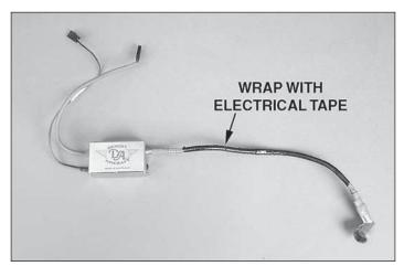
□ 21. Wrap the shielded spark plug lead of the igniter unit with electrical tape. This will help prevent damage of the braided shield. Make sure that the battery leads you have match the leads for your ignition module. We had to splice in some new Futaba "J" leads to work with our battery.
