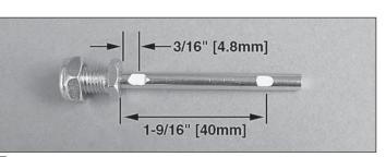
□ 1. Locate the  $3/16" \times 2" [4.8 \times 51mm]$  axles, four 3/16" [4.8mm] wheel collars, four set screws, two axle nuts, and the two main wheels. File flat spots in the axle in the locations shown above.
