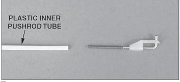
□ 9. Locate the 24" [610mm] plastic inner pushrod tube, one 2-56 x 6" [152mm] threaded one-end rod, and one nylon FasLink<sup>™</sup>. Trim the rod 2" [51mm] from the threaded end and make an "L" bend. Thread the rod into one end of the inner pushrod tube. This side will attach to your throttle servo arm.
