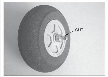
□ 3. Use a rotary tool with a cutoff wheel attachment to cut off the excess portion of the axle.
