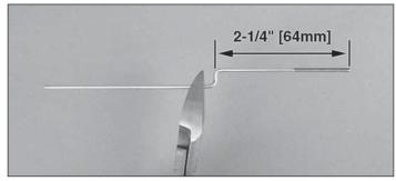
□ 7. Locate the 2-56 x 6" [152mm] threaded one end rod. Measure 2-1/2" [64mm] from the threaded end and make a mark. Start your Z-bend at the mark so that the leg of the bend is 2-1/2" [64mm] from the threaded tip. Clip off the excess rod. This will be referred to as "**pushrod A**."
