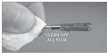
□ □ 5. While the joint is still hot but after the solder solidifies use a clean, damp cloth to wipe the flux from the joint before it hardens. Flux is corrosive and must be thoroughly cleaned from the joint.
