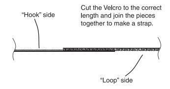
■ 8. Locate the non-adhesive backed hook and loop material. Make two sets of straps for your receiver and battery by joining a piece of "hook" material to a piece of "loop" material.
