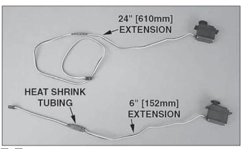
□ □ 1. Prepare your outboard aileron servo with a 24" [610mm] extension. Prepare the inboard servo with a 6" [152mm] extension. Use heat shrink tubing to secure the connectors so they do not come loose. **Note:** If you anticipate mounting your radio equipment in the aft-most equipment bay, you do not need the 6" [152mm] extensions installed.
