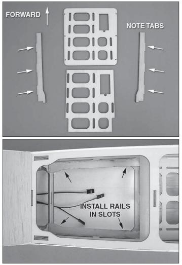
□ 6. Locate the aft equipment tray and the two side rails. Align the tabs on each rail with the corresponding slots in the fuselage and glue each rail in place as shown.
