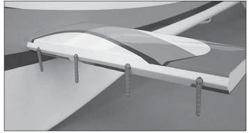
□ 4. Fit the hinges into the stab, making sure to orient them so that the hinge pin is parallel to the hingeline.
