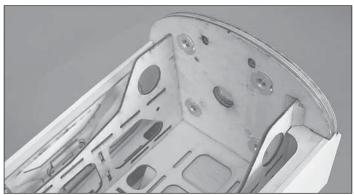
□ 3. Install four 1/4-20 blind nuts in the firewall from the back side.
