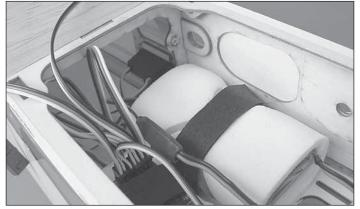
□ 12. We used a 2.4GHz radio system for this build-up, but if you're using a 72MHz radio system, an antenna routing tube is provided for you in the upper left side of the fuselage.
