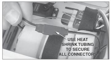
□ 17. Connect the battery to the switch. Use heat shrink tubing to secure the connection between the battery and the switch.
