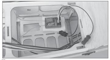
□ 9. Connect a Y-connector to each aileron channel. Connect the other servo leads, the battery switch, and your ESC signal lead to your receiver.
