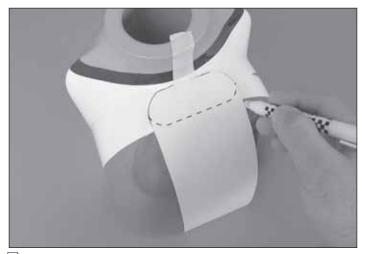
□ 1. If you're using a gas engine inverted, turn to the back of this manual and cut out the paper template. Fold along the dotted line and center the template along the bottom of the cowl. The folded edge holds the template in position. Trace a line around the template using a felt-tip marker and trim out the clearance hole.
