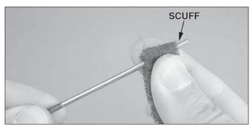
□ □ 2. Starting with the aileron pushrods, gather the four 4-40 x 3-1/2" [89mm] threaded one end rods and four solid metal (unthreaded) clevises. Roughen the unthreaded end of each with some coarse 150-grit sandpaper or a coarse Scotch Brite<sup>®</sup> pad.
