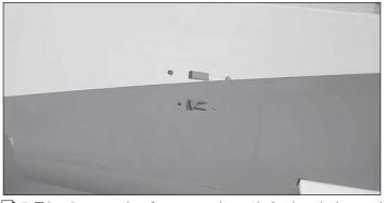
$\Box$  5. Trim the covering from over the switch plate holes and install the switch and charge jack.
