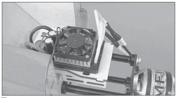
□ 8. Mount your ESC using double-sided tape or the method specified by the manufacturer.
