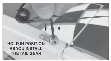
□ 6. Loosen the tail gear collar set screw and remove the collar. Position the collar under the tail gear retainer as you insert the tail gear into the bushing. Do not tighten the collar yet.
