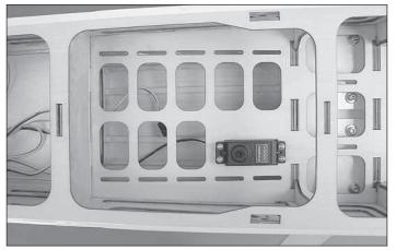
$\Box$  6. Install the throttle servo in the center equipment tray as shown. Use a 1/16" [1.6mm] drill bit for the servo screw holes.
