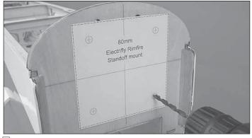
□ 1. Turn to the back of this manual and cut out the drilling template for the RimFire electric motor. Center the template by matching the template crosshairs with the firewall crosshairs.
