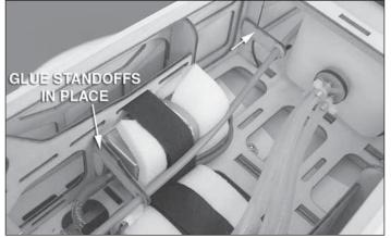
□ 13. Position and glue the pushrod standoffs and the outer pushrod tube in place.
