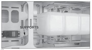
☐ 14. Fit and glue the pushrod supports to the fuselage former just ahead of the throttle servo. Glue them so that the pushrod aligns with the servo arm and won't bind up when the servo moves. Trim the excess pushrod wire, but leave enough in case you want to make adjustments later.
