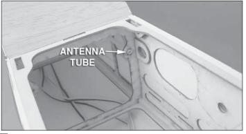
□ 10. We used a 2.4GHz radio system for this build-up, but if you're using a 72MHz radio system, an antenna routing tube is provided for you in the upper left side of the fuselage.
