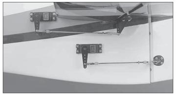
□ 7. Install the 5-1/4" [133mm] pushrod to the left elevator servo and elevator.
