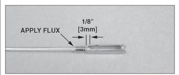
□ □ 3. Apply a few drops of soldering flux to the unthreaded end of the pushrod. Position the clevis so that 1/8" [3mm] of the pushrod protrudes past the barrel of the clevis.
