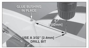
□ 3. Make a mark 4" [102mm] back from the hinge line on the bottom of the rudder. Make sure that the mark is centered and drill a 1/2" [13mm] deep hole here for the plastic tailwheel guide wire post. Use a 3/32" [2.4mm] pilot drill bit and then step up to a 5/32" [4mm] bit for the final hole.
