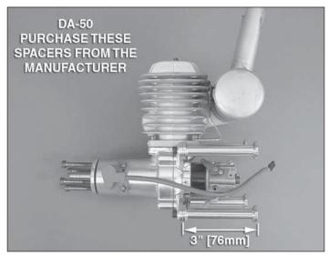
□ 1. Install the 3" [76mm] aluminum standoffs using the hardware supplied by the engine manufacturer.
