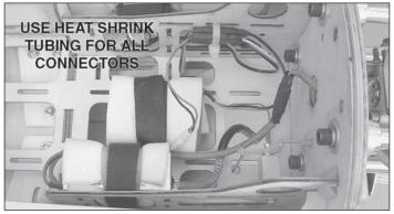
□ 25. Connect the ignition module to the ignition switch. Connect the crank pickup to the ignition module. Connect the ignition battery to the ignition switch. Use heat shrink tubing to secure the connectors and a tie wrap to secure them to the upright.
