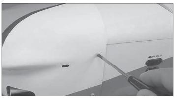
$\Box$  11. Use four #4 x 1/2" [13mm] sheet metal screws along with four Dubro #4 nylon washers to install your cowl.
