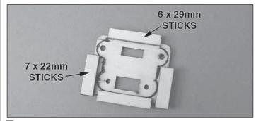
$\Box$  17. Use two 7 x 22mm and two 6 x 29mm sticks to make a flange for the charge plate.
