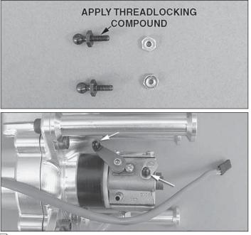
□ 2. Locate two 2-56 threaded ball links and two 2-56 hex nuts. Install one on the throttle arm and one on the choke arm using threadlocking compound. Secure the ball links using the 2-56 hex nuts.
