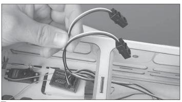
□ 7. Connect a Y-connector to each aileron channel. Connect the other servo leads to your receiver
