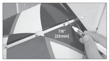
2. Turn the fuselage over (a foam building stand is helpful) here). Use a felt-tip pen to make a mark on each elevator that is 7/8" [22mm] from the side of the fuselage.
