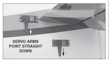
□ 1. Center your servos. Attach a 1-1/2" [38mm] singlesided servo arm to each servo so that the arm is 90° to the servo case when the servo is centered. Install the arms so that they point down.
