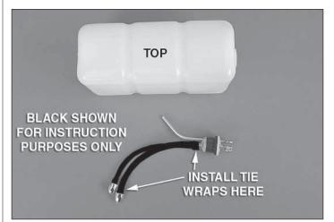
□ 30. Cut two pieces of fuel line so that each one is 5" [127mm] long. Build up the fuel tank with the vent line pointing to the top of the tank. Secure the lines within the tank with small tie wraps.
