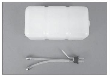
□ 15. Cut two pieces of fuel line so that each one is 5" [127mm] long. Build up the fuel tank as shown with the vent
