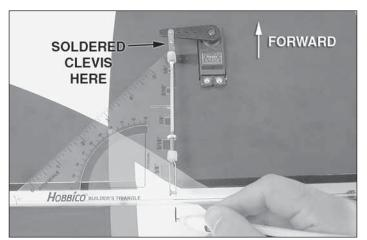
□ □ 2. Attach the soldered clevis end of each pushrod to the servo arm in the hole that is 1-1/4" [32mm] out from the center of the arm. Extend the pushrod straight back so that it is 90° to the hinge line and draw a centerline on the aileron. Use a builder's triangle to ensure that the rod is 90° to the hinge line.
