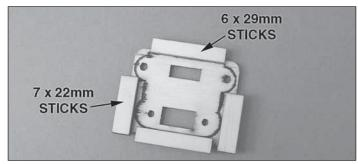
$\Box$  2. Use two 7 x 22mm and two 6 x 29mm sticks to make a flange for the charge plate.
