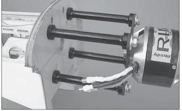
$\Box$  4. Locate four 50mm, 20mm, and 10mm standoff spacers as well as eight mounting feet, four 1/4-20 x 5" [127mm] bolts, four flat washers, and four lock washers. Install the motor using these parts as shown.
