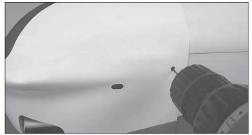
□ 9. Temporarily fit the canopy and hatch. Fit the cowl once again, making sure to slide it back until the centering tool contacts the drive washer. Use a 1/16" [1.6mm] drill bit to make four 1/2" [13mm] deep holes in the fuselage sides (two per side). Drill them so that they are 1/2" [13mm] from the rear edge of the cowl. Apply thin CA to the holes to harden the wood.
