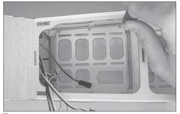
□ 7. Position the aft equipment tray in the aft bay and use a 1/16" [1.6mm] drill bit to drill six pilot holes through the side rails. Use six #2 x 3/8" [10mm] sheet metal screws with six #2 washers to attach the aft equipment tray.
