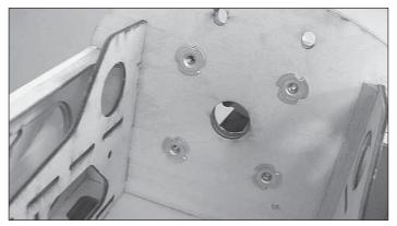
□ 3. Press four 8-32 blind nuts into the engine mount holes you drilled. Press them in from the back side of the firewall. You may need to use 8-32 bolts and washers to draw the nuts into the holes.
