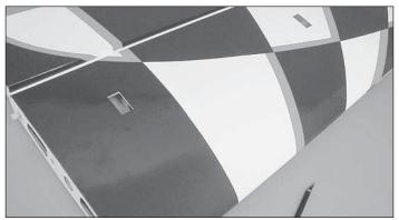
□ □ 2. Locate the aileron servo bays on the underside of the wing and trim away the covering. If you have not done so already, use a covering iron to tack down the covering before you trim.
