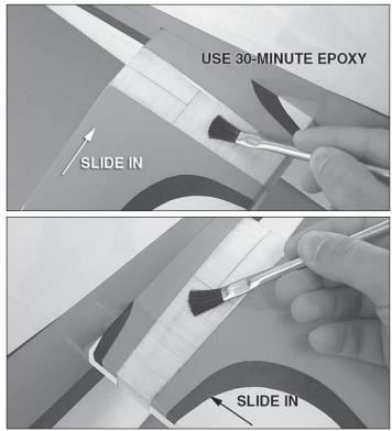
7. Apply 30-minute epoxy to the top and bottom of the stab center section and slide it into the fuselage. Pull the stab through the fuselage past center and re-coat the center section on the opposite fuselage side. Slide the stab back into the fuselage, and then center it and level it like you did earlier.
