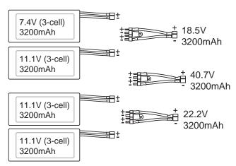
It's okay to connect batteries with different Voltages in <u>Series</u> to achieve the new, desired Voltage.
