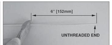
□ 8. Locate the 2-56 x 36" [914mm] threaded one end rod. Measure 6" [152mm] from the unthreaded end and make a mark. Cut the wire at the mark and retain this portion. This will be referred to as "**pushrod B.**" The remaining portion of the rod will be used for the throttle later.
