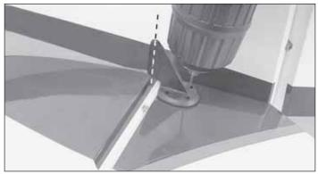
□ 3. Center a control horn over the line that you made making sure that the clevis holes are also centered over the hinge line. Hold the horn in position and use a 1/16" [1.6mm] drill bit to drill four holes in the elevator. Remember to only drill 1/2" [13mm] deep.
