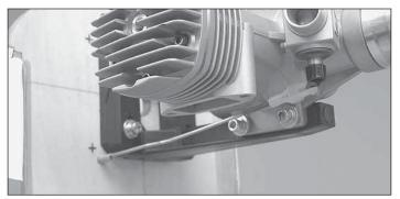
□ 12. Slide the pushrod into the plastic tube and connect the clevis to your throttle arm. Slide the other end of the pushrod into the screw-lock pushrod connector. Bend the throttle pushrod as needed to clear your muffler or any obstructions.
