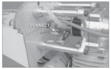
□ 12. Trim the inner pushrod tube to length and install the ball link socket onto the throttle. Keep in mind that the throttle is sprung shut and that you will have to hold it fully open when you adjust the pushrod length.
