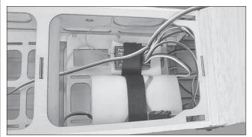
□ 10. Wrap your receiver and battery pack with 1/4" [6.4mm] thick latex foam. Use the straps you made to mount your battery and receiver to the aft equipment tray.
