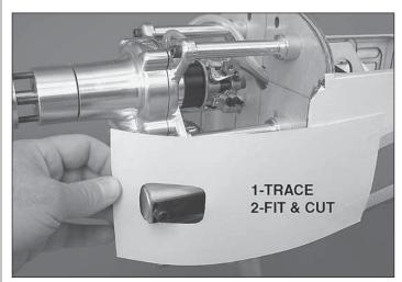
□ 2. Tape a suitably sized piece of card stock to the fuselage side and use it as a template to trim a clearance hole for your muffler. If you're working with a side mounted glow engine, you will use this method to make a template for the cylinder head. Use cardstock to trim holes for your engine's needle valves.
