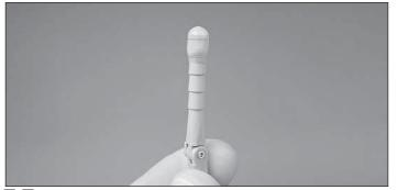
□ □ 6. Dip both ends of each hinge (about two barbs deep) into your epoxy cup.
