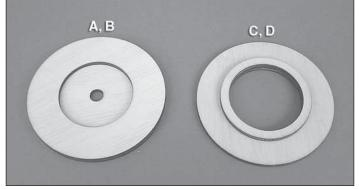
□ 5. Build the inside portion and the outside portion of cowl centering tool as shown. Use medium CA to glue them together.
