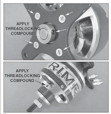
□ 2. Prepare your motor by removing the motor mount screws, the two forward motor case set screws, and the rear locking collar set screw. Apply threadlocking compound to these and reinstall them.
