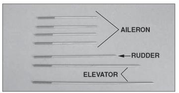
$\Box$  1. Locate the seven 4-40 x 12" [305mm] threaded one end pushrods. You'll need to cut the rods down to the following lengths:
