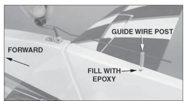
□ 7. Apply epoxy to the plastic tailwheel guide wire post and slide it onto the tailwheel guide wire. Glue the post into the hole you drilled in the bottom of the rudder.
