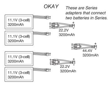
Connecting batteries in "**Series**" means to connect the +'s to the -'s and the -'s to the +'s. This combines the batteries' voltages, but the capacity remains the same.
