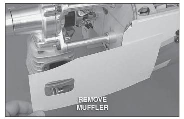
□ 3. Remove the muffler while leaving the template in place.
