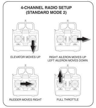
□ 3. Make certain that the control surfaces and the carburetor respond in the correct direction as shown in the diagram. If any of the controls respond in the wrong direction, use the servo reversing in the transmitter to reverse the servos connected to those controls. Be certain the control surfaces have remained centered. Adjust if necessary.
