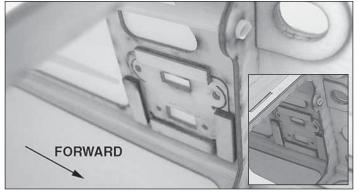
□ 3. Install the switch plate on the model using epoxy. For C.G. reasons, the radio equipment is mounted in the aft equipment bay. A cutout for the switch plate is provided in the left and right rear fuselage. You may choose either location.
