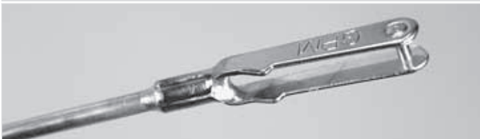
This is what a properly soldered clevis looks like—shiny solder with good flow, no blobs, flux removed.
