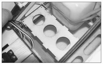
3. Test fit the radio tray as shown. Sand as needed for a good fit.
