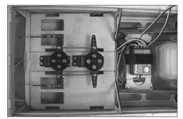
6. This is what the final installation will resemble. If you do not plan on mounting a gasoline engine in the future, the two radio trays next to the pull-pull system may be omitted.
