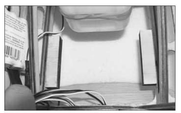
2. Glue the two rails in place as shown using epoxy.
