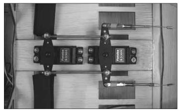
This poses a problem however, as the servo arms are unable to clear the battery and receiver when in motion. To resolve this problem, we have included a separate battery and receiver tray to be used when installing a glow engine.
