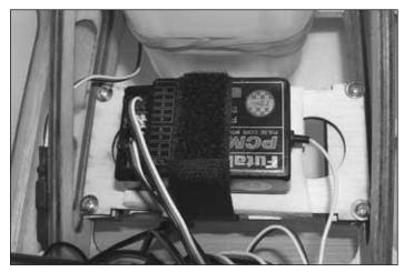
5. Attach the radio tray to the hardwood rails with the included  $3mm \times 3/8"$  [9.6 mm] wood screws and 3mm washers as shown. Sand as needed for a good fit. Remember to harden the screw holes by wicking some thin CA into them and allowing it to fully harden before final screw installation.
