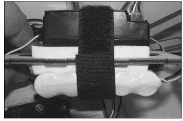
4. Assemble the radio tray as shown using the supplied hook and loop material. Use 1/4" [6.4 mm] foam (not included) under the receiver and battery for vibration protection.
