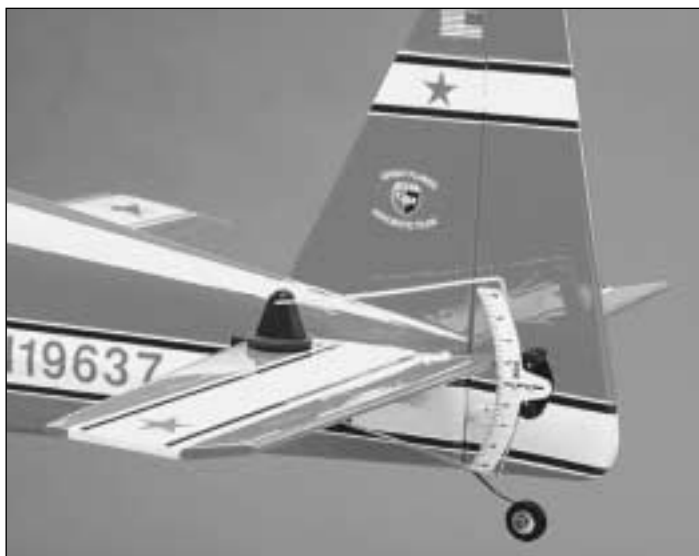
Great Planes® Accu-Throw™ Control Surface Deflection Meter GPMR2405
