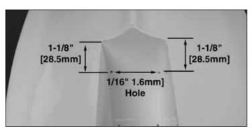
□ 13. Drill a 1/16" [1.6mm] hole in both of the aft corners, 1-1/8" [28.5mm] from the bottom of the fuselage.
