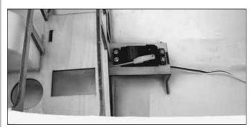
□ 9. Temporarily connect the steering servo to your receiver and center the servo arm. Position the nose gear wire so that it is perpendicular to the centerline of the fuselage. Mark the pushrod where it crosses the mounting holes in the servo arm. Make a 90° bend at the mark. Attach the pushrod to the servo arm using a nylon FasLink. Cut the excess pushrod wire so that it slightly protrudes out of the FasLink.
