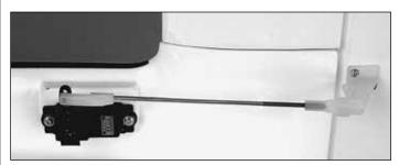
□ 6. Slide a silicone clevis retainer over the clevis. Center the elevator servo arm and the elevator. Mark the pushrod where
