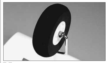
□ □ 16. Install a 5/32" [4mm] wheel collar and 6-32 [4mm] set screw on the landing gear wire, followed by one of the foam wheels and a second wheel collar and set screw.
