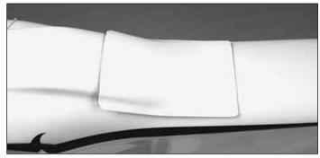
□ 7. Use a sharp canopy scissors and sanding bar to trim the throttle servo hatch cover to fit the fuselage.
