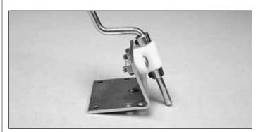
□ 2. Slide a 5/32" [4mm] wheel collar on the nose gear wire. Insert the nose gear in the nose gear bearing and install a second 5/32" [4mm] wheel collar. Secure the wheel collars to the nose gear wire with a 6-32 [4mm] set screw.
