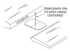
□ 5. To keep the CA hinges centered in the control surfaces while installing them, insert a T-pin in the center of the hinge. Insert the hinges in the stabilizer and install the elevator. Remove the T-pins and adjust the control surface so that the leading edge of the elevator is against the trailing edge of the stabilizer.
