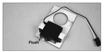
□ 1. Position the Micro servo with the top of the servo case flush and centered with the edge of the throttle servo tray. Use epoxy to glue the two hardwood servo tray blocks on each side of the servo against the servo mounting flanges.
