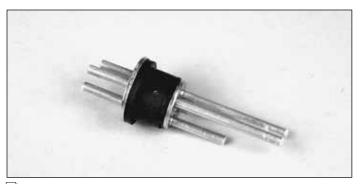
□ 1. Remove the components from inside the fuel tank. Install the three aluminum tubes in the fuel tank stopper. You will need to use a hobby knife to open the third hole in the rubber stopper. Slide the small metal plate over the tubes and thread the screw into the plate until it makes contact with the back of the rubber stopper. **Do not** tighten the screw.
