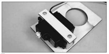
□ 4. Position the plywood servo retainer over the servo and drill a 1/16" [1.6mm] pilot hole at each end through the retainer and into the servo tray block.
