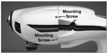
$\Box$  5. Drill a 1/16" [1.6mm] pilot hole, above and below the air exit indentation. Increase the hole in the cowl only to 3/32"
