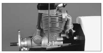
↓ 4. Use a Great Planes Dead Center<sup>™</sup> hole locator to mark on the engine mount the four engine mounting holes.
