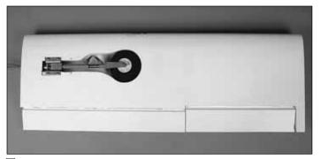
□ 6. Install the ailerons and flaps on both wing halves following the same procedure used to install the hinges in the rudder and elevator.
