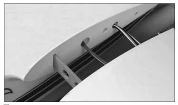
□ 2. Route the servo wires and air line tubing, if retracts are installed, through the holes in the fuselage.
