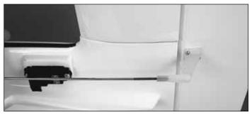
□ 4. Position the control horn on the elevator so that the elevator pushrod is parallel to the centerline of the elevator servo and over the hardwood block. Mark the location of the control horn mounting holes and drill a 1/16" [1.6mm] pilot hole at each mark. Temporarily mount the control horn to the elevator with two #2 x 3/8" [9.5mm] sheet metal screws.
