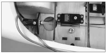
□ 7. Thread a nylon clevis approximately 14 turns onto the end of a 6" [152mm] wire pushrod. Install a silicone clevis retainer on the clevis. Install the clevis on the control valve.
