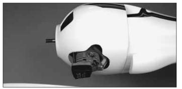
□ 3. Remove the cowl and template, and then remount the engine. Cut out the hole in the cowl, test-fitting it over the engine as you go.
