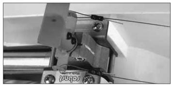
□ 18. Lower the nose gear retract and slide a metal furl on each of the steering cables. Route the cables through the attachment arms on the nose gear and back through the furls. With the steering servo arm centered and the nose gear straight, pull the cable tight. Then, crimp the two furls on the cable. Cut off the excess cable.
