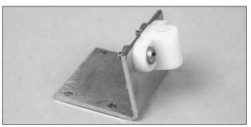
□ 1. Attach the nylon nose gear bearing to the nose gear mounting plate using two 6-32 x 1/2" [4 x 12.7mm] machine screws, two 6-32 [4mm] nuts and #6 washers.
