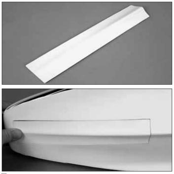
□ 2. Use a canopy scissors or a Dremel<sup>®</sup> Rotary Tool and sandpaper to trim the fiberglass nose gear cover to fit on the nose gear cover plate and in the nose gear opening.
