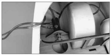
□ 5. Attach the control valve to the plywood control valve mount. Attach the air line tubing to the control valve and glue the mount to the radio tray.
