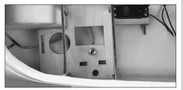
□ 4. Drill a hole in the radio tray to fit your fill valve. Attach air line tubing between the air tank and fill valve.
