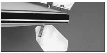
□ 5. Insert the water rudder control rod in the quick connector on the bottom of the rudder. Insert the water rudder in the fuselage and connect the water rudder control rod to the water rudder. Do not trim off the excess control rod until after the rudder throws have been set.
