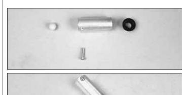
□ 1. Glue the rubber bushing in the end of the aluminum bailing tube, opposite the end for the machine screw. Insert the ball in the aluminum bailing tube and thread the 3-56 x 3/8" [9.5mm] machine screw into the aluminum bailing tube.
