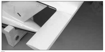
□ 3. Use 30-minute epoxy to glue the two stabilizer halves to the tail and the carbon tubes.
