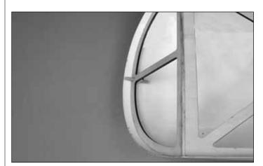
□ 3. Round one end of the  $5/32" \times 1-3/16" [4 \times 30mm]$  wood dowel rod. Glue the dowel in the aft end of the cabin top. The end of the dowel should be flush with the edge of the cabin.
