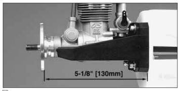
□ 3. Position the engine on the engine mount so that the front of the drive washer (or back of the spinner) is 5-1/8" [130mm] from the firewall. Also make sure the engine is centered on the engine mount.
