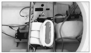
□ 4. Install the receiver on/off switch on the left side of the radio tray. Wrap the receiver and receiver battery in foam and place them on the radio tray. If flying from the water, we recommend placing the receiver and battery in a plastic bag.
