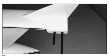
□ 1. Install the horizontal stabilizer tubes in the tail. The short tube is installed in the forward hole.
