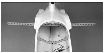
□ 1. Insert the aluminum wing joiner in the fuselage. Space it evenly on both sides of the fuselage.
