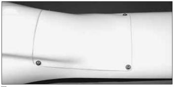
■ 8. Note the four wood blocks, in each corner, under the throttle servo hatch opening. Position the hatch cover over the opening and drill a 1/16" [1.6mm] pilot hole in each corner. Remove the hatch cover and enlarge the holes in the cover to 3/32" [2.4mm]. Secure the hatch cover to the fuselage with four 2 x 8mm sheet metal screws and 2mm washers.
