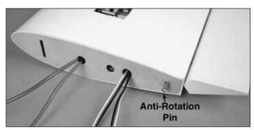
$\Box$  1. Use denatured alcohol to clean the 5/32" x 1" [4 x 25.4mm] metal anti-rotation pins. Then, use epoxy to glue the pins in both wing panels, in the aft hole of the root rib. Apply a thin film of epoxy on the rib to seal the wood.
