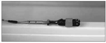
□ 15. Install a 2-56 nut half-way onto the threaded coupler. Install a silicone clevis retainer on a 2-56 threaded metal clevis. Install the clevis on the threaded coupler and tighten it against the 2-56 nut.
