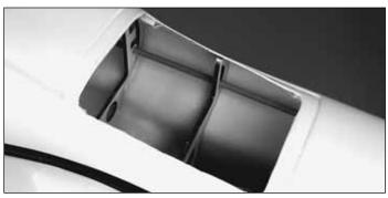
□ 1. Insert the 11-3/4" [298mm] gray outer pushrod tube in the fuel tank compartment through the formers as shown. Note the location that the pushrod tube hits the back of the firewall. This will give you an idea where the pushrod must exit the firewall to allow smooth operation.
