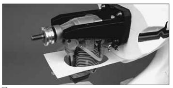
□ 1. Use a piece of thin cardboard or plastic to make a template for the cutout in the cowl for the head of the engine. Tape the template to the fuselage, accurately indicating the position of the head.
