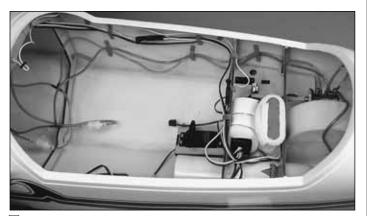
□ 6. Cut a piece of rubber band 3/4" to 1" [19 to 25.4mm] long. Position the rubber band where needed. If you have long servo wires you may need several harnesses. The harnesses can easily be glued to the side of the fuselage with CA. For best adhesion, roughen the area with sandpaper before applying CA.
