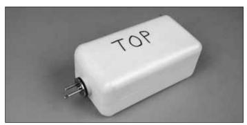
$\Box$  4. Insert the tank stopper in the fuel tank. Check that the two clunks are able to move freely when the stopper is inserted completely. Then, tighten the screw in the stopper to seal the fuel tank. Write "top" on the side of the fuel tank where the pressure tube sticks up.
