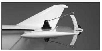
Use a Great Planes AccuThrow (or a ruler) to accurately measure and set the control throw of each control surface as indicated in the chart that follows. If your radio does not have dual rates, we recommend setting the throws at a rate inbetween the high and low rates.
