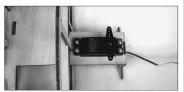
□ 1. Drill 1/16" [1.6mm] pilot holes and mount the steering servo, using the hardware that came with your radio.
