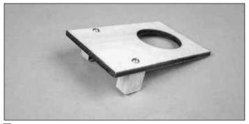
□ 2. Once the glue has cured, remove the servo, turn the servo tray over and drill a 1/16" [1.6mm] pilot hole through the servo tray and into the servo tray blocks, centered in the blocks. Secure the servo tray blocks to the servo tray with two #2 x 3/8" [9.5mm] self-tapping screws.
