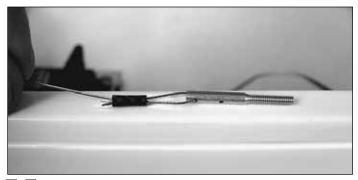
□ 14. Put a piece of masking tape on the end of one of the metal cables. Insert the cable in one of the holes. The masking tape will prevent the cable from pulling through the hole. Slide a metal furl on the cable inside the fuselage. Then thread the cable through the bottom hole in the threaded coupler and then back through the furl. Use a pliers to crimp the furl on the cable.
