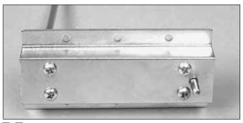
□ 14. Position the landing gear block in the metal main landing gear mount so that the landing gear wire goes through the mount. Drill a 7/64" [2.7mm] pilot hole at each mounting hole location and attach the landing gear block to the metal mount with four #6 x 1/2" [12.7mm] sheet metal screws.
