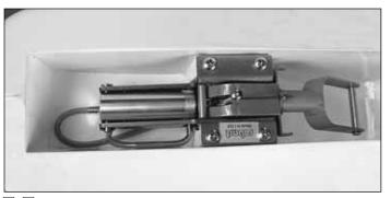
□ □ 12. Mount the nose gear retract in the fuselage with the screws included with the main retract.
