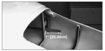
□ 2. Drill a 3/16" [4.8mm] hole through the front of the firewall. Roughen the outer pushrod with sandpaper. Insert the outer pushrod tube through the firewall and the former so that it protrudes through the first former by approximately 1" [25.4mm]. Trim the excess flush with the front of the firewall.
