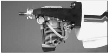
□ 7. Remove the four 8-32 [4mm] socket-head cap screws from the engine mount and rotate the mount 180 degrees so that the engine is mounted inverted. Be sure to use thread-lock on the 8-32 [4mm] socket-head cap screws when reinstalling them.
