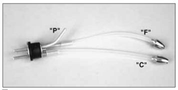
□ 3. Install a piece of fuel tubing on each of the other two tubes. Attach a clunk on the ends of the tubes. Mark a "C" on the outside of the front plate by the short tube, designating carb, and an "F" by the remaining tube, designating fill.
