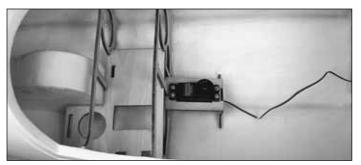
□ 5. Drill 1/16" [1.6mm] pilot holes and mount the steering servo, using the hardware that came with your radio.
