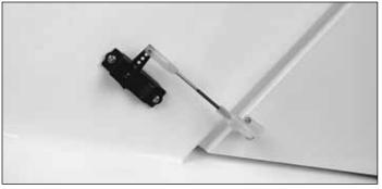
□ 7. Follow the same procedure to install the rudder servo. Make sure the control horn is installed over the hardwood block.
