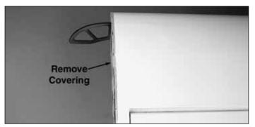
□ 4. Remove the wing tip and use a sharp hobby knife to trim the covering from inside the wing tip outline.
