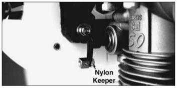
□ 3. Install a screw-lock pushrod connector on the throttle arm and secure it with a nylon keeper.
