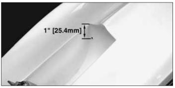
□ 6. Drill a 3/32" [2.4mm] hole through the aft edge of the nose wheel recess, 1" [25.4mm] from the bottom of the fuselage. You will need to remove the nose gear to allow room for the drill. While the nose gear is removed, apply a couple of drops of thin CA to each of the screw mounting holes to harden the wood, before remounting the nose gear.
