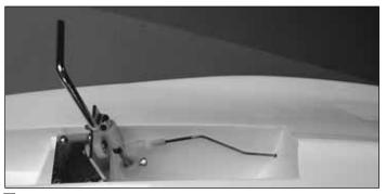
□ 8. Insert the pushrod in the hole at the back of the nose wheel recess. The pushrod will require some bending so that the clevis can be attached to the steering arm.
