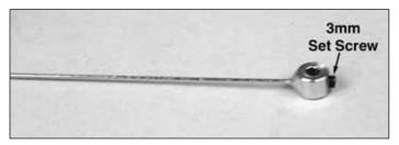
□ 4. Install a 1/8" [3mm] set screw in the water rudder control rod.
