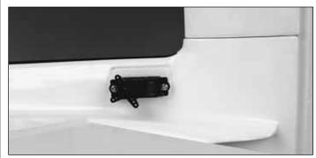
□ 2. Install the elevator servo in the fuselage using the hardware supplied with the servo.
