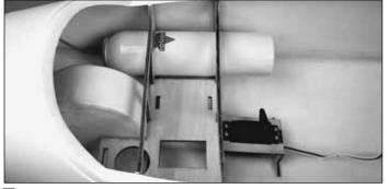
□ 3. Install a piece of air line tubing on the retract air tank. Use silicone adhesive or epoxy to glue the retract air tank in the formers on the right side of the fuselage.
