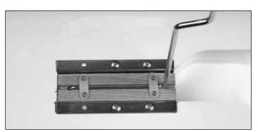
□ 15. Insert the landing gear in the wing so that the landing gear wire is closest to the wheel recess. Mark and drill four 7/64" [2.7mm] pilot holes, in the mounting holes closest to the landing gear wire. Secure the landing gear to the wing with four #6 x 1/2" [12.7mm] sheet metal screws in the positions shown.
