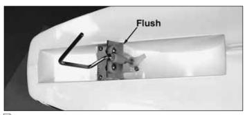
□ 4. Position the nose gear plate so that the aft edge of the plate is flush with the aft edge of the nose gear mount in the fuselage. Mark the four mounting holes and drill a 3/32" [2.4mm] pilot hole at each mark. Attach the nose gear plate to the fuselage with four #4 x 1/2" [12.7mm] sheet metal screws.
