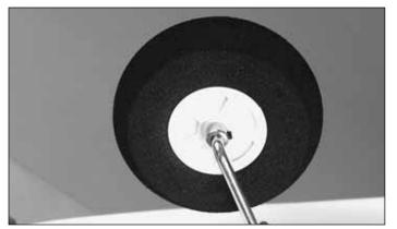
□ 10. Install a 5/32" [4mm] wheel collar and 6-32 [4mm] set screw on the nose gear wire, followed by one of the foam wheels and a second wheel collar and set screw.
