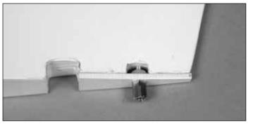
□ 2. Use epoxy to glue the rudder base to the bottom of the rudder. Make sure the epoxy covers all of the bare wood surfaces.
