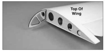
□ 2. Insert and glue the wing tip support in the tip rib of the left wing.
