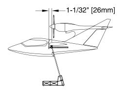
□ 2. With the wing attached to the fuselage, all parts of the model installed (ready to fly) and an empty fuel tank, place the model right-side up on a Great Planes CG Machine, or lift it right-side up at the balance point you marked.
