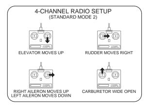
□ 3. Make certain that the control surfaces and the carburetor respond in the correct direction as shown in the diagram. If any of the controls respond in the wrong direction, use the servo reversing in the transmitter to reverse the servos connected to those controls. Be certain the control surfaces have remained centered. Adjust if necessary.
