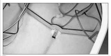
□ 2. Use epoxy to glue the aluminum bailing tube in the hole in the bottom of the fuselage. The rubber bushing goes to the inside of the fuselage. The aluminum bailing tube should be flush with the outside of the fuselage. Do not get epoxy in the tube. The ball must be able to move freely. The ball will float in the water and seal against the rubber bushing. In flight, the ball will roll back and allow water to escape from the fuselage.
