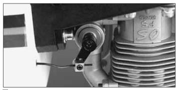
□ 7. Use a pliers to bend the throttle pushrod so that it can be inserted in the screw-lock pushrod connector. Cut off the excess pushrod and secure the pushrod in the screw-lock pushrod connector with a 4-40 set screw.
