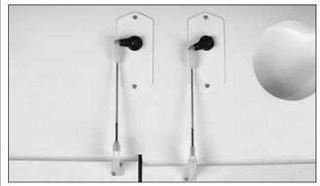
□ 12. Once you have the aileron and flap servos installed, remove the horns and install the servo covers using two #2 x 3/8" [9.5mm] sheet metal screws. Remember to remove the screws and use thin CA to harden the screw holes. If you will be flying the Seawind ARF from water, we recommend that you apply a bead of silicone sealant between the servo covers and the wing to help seal the covers.
