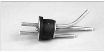
□ 2. Carefully bend one of the long tubes so that it will angle up toward the top of the fuel tank when inserted. Do not kink the tube. Mark a "P" on the outside of the front plate to designate pressure.
