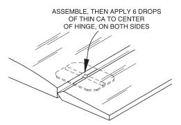
□ 6. Add 6 drops of thin CA to the center of all the hinges on both the top and bottom.
