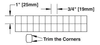
□ 4. Cut the four 3/4" x 1" [19 x 25.4mm] hinges for the stabilizer from the supplied 2" x 9" [51 x 228mm] hinge material. Trim the corners of each hinge.
