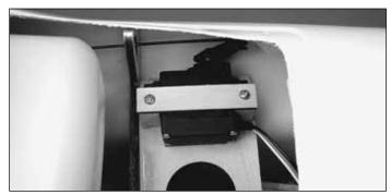
■ 8. Use epoxy to glue the throttle servo tray in the fuel tank compartment.
