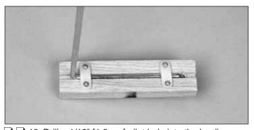
□ □ 13. Drill a 1/16" [1.6mm] pilot hole into the landing gear block at each mark. Secure the landing gear straps to the block with four #2 x 3/8" [9.5mm] sheet metal screws.
