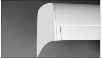
□ 3. Test fit the left fiberglass wing tip on the left wing panel. The wing tip curves downward. Use a felt-tip pen to mark the outline of the wing tip on the wing.
