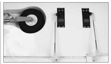
□ 11. Install the flap pushrod on the flap servo arm following the same procedure used to install the aileron pushrod.
