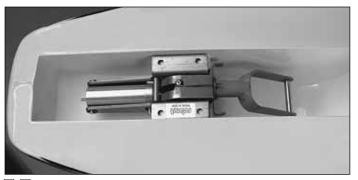
□ □ 10. Position the nose gear retract on the landing gear rail.
