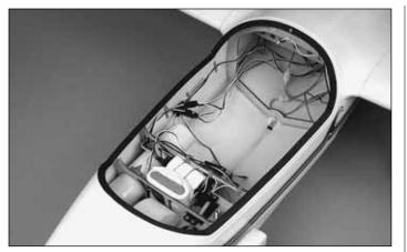
□ 4. Remove the backing from the foam tape and apply it to the cabin area of the fuselage.
