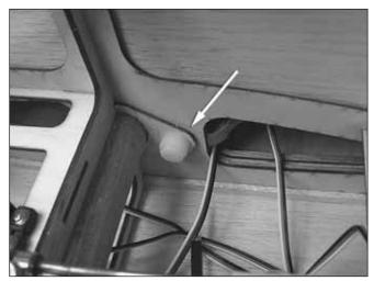
Secure each wing half to the fuselage with a 1/4" x 20" nylon bolt. The bolts only need to be installed and tightened by hand. No screwdriver is required.
