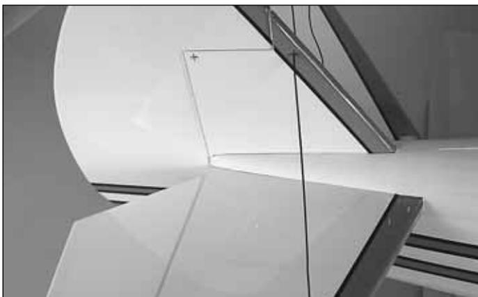
□ □ 5. Thread the cord through the hole in the leading edge of the fin.
