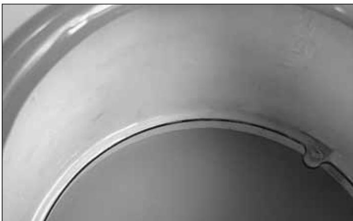
❑ 8. Sand the inside of the cowl, in front of the cowl ring with 220-grit sandpaper. Wipe the area clean with denatured alcohol and allow the area to dry. Mix one ounce of 6-minute epoxy and micro balloons. Apply a fillet of the glue to the cowl and the cowl ring. Set the cowl aside until the glue has cured.
