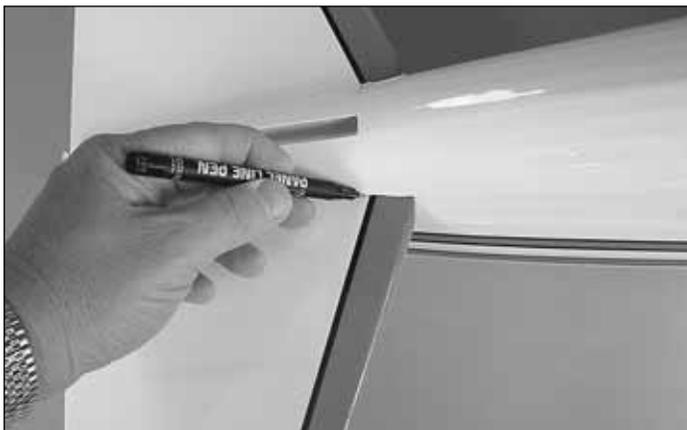
□ 3. Using a felt-tip pen, mark the outline of the fuselage on the top and the bottom of the stab.
