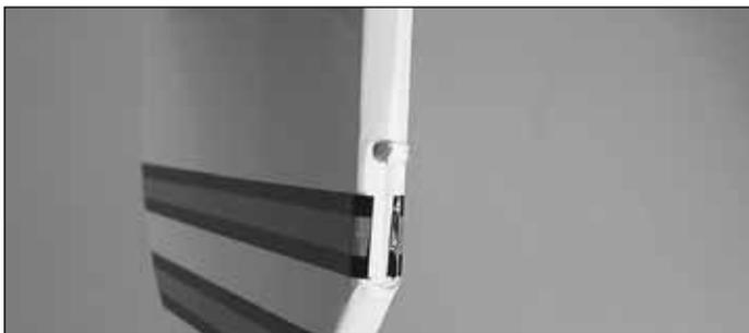
❑ 11. Cut the covering from the hole on the leading edge, bottom of the rudder. Test fit the hinges into the rudder and then fit the rudder to the fin and fuselage. Make any adjustments that may be needed to the slot in the rudder. When you are satisfied everything fits well, put a small amount of epoxy into the hole in the rudder, install the hinges in the rudder and install the rudder to the fin.
