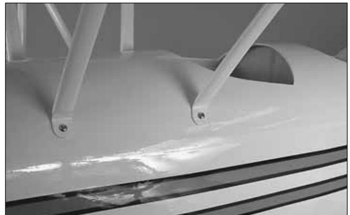
❑ 15. Install and then remove a #4 x 1/2" sheet metal screw into each of the four holes. Apply a couple drops of thin CA into each of the holes to harden the threads. After the glue has cured permanently install the screws into the fuselage.
