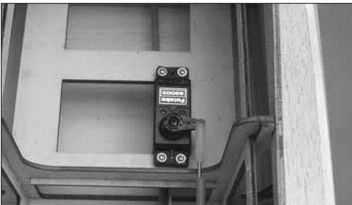
❑ 7. Cut the 1" [25mm] threaded end from the .074" x 17-1/2" [445mm] throttle pushrod wire. Install the wire into the tube and attach it to the servo horn arm with a Faslink. Use the same technique used for the ailerons.
