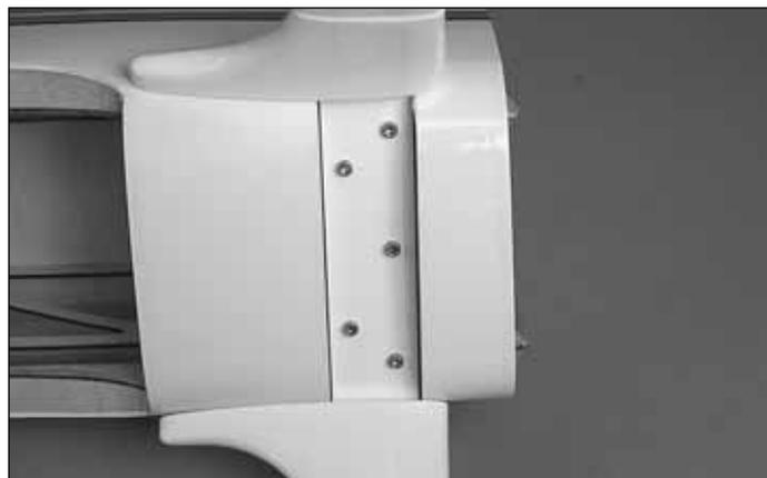
❑ 1. Remove the belly pan from the bottom of the fuselage. Install the landing gear to the fuselage with five 8-32 x 3/4" [19mm] socket head cap screws. Apply a drop of thread locker to each bolt before installing them.
