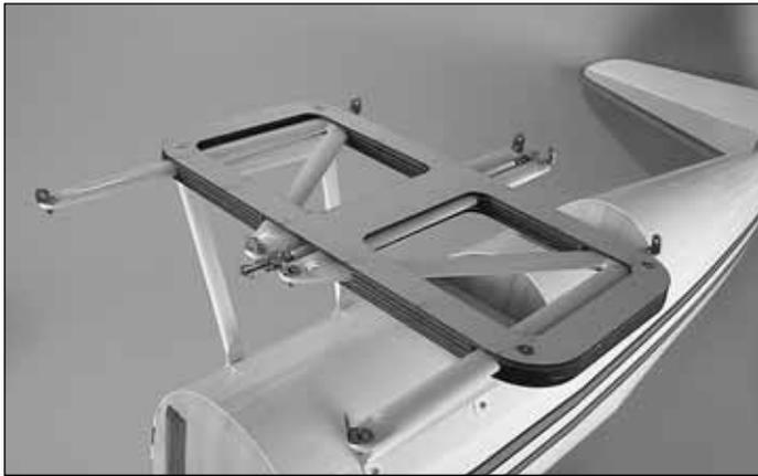
□ 7. Place the two “N” struts into the handle and the two aileron connecting rods between the struts. Put the handle top onto the part of the handle holding the struts and place the completed handle on top of the cabanes. Secure the handle to the cabanes with four 4-40 x 3/4" [19mm] socket head cap screws and #4 flat washers. This is how the completed handle looks when you are storing the parts or taking the plane to the field.
