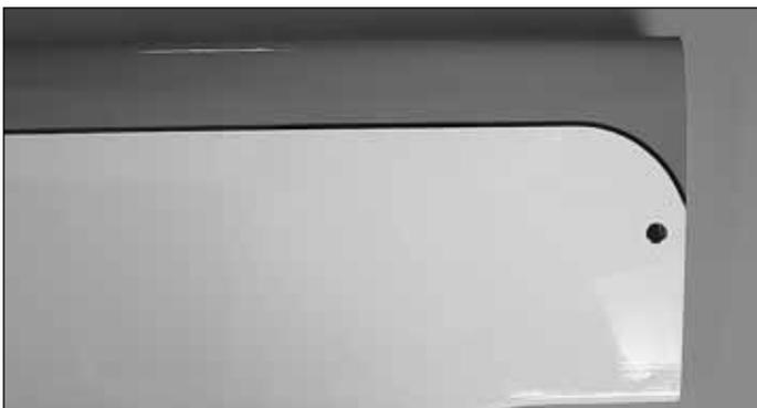
□ □ 4. Starting with the right wing panel for the top wing, cut away the covering from the servo opening on the bottom of the wing and the covering from the hole at the root of the wing. Remove the tape from the root rib, thread the string through the hole and tape the string to the wing. Tape the string in the servo bay to the wing, too.
