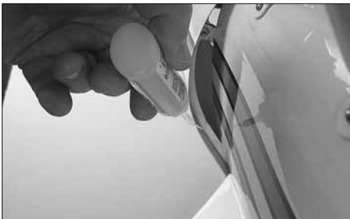
❑ 6. Once you are satisfied with the position of the cowl, tack glue the cowl ring to the cowl with medium CA using a CA applicator tip. Apply the glue on the back of the cowl ring and apply some CA accelerator to the glue to enable it to cure quickly. Do this on both sides of the cowl.
