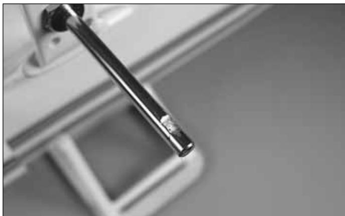
□ □ 8. File a flat spot on the axle on the mark you made. Re-install the wheel pant, wheel and wheel collars onto the axle. Center the wheel and tighten the screws against the axle.
