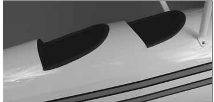
❑ 2. Locate two pieces of black **cockpit coaming**. Look closely and you will see that there is a slit in it. Slide the coaming onto the edge of the cockpits. Glue it in place with R/C 56 canopy glue. This glue sticks well to MonoKote eliminating the need to cut any covering, exposing wood in order to get a good bond.
