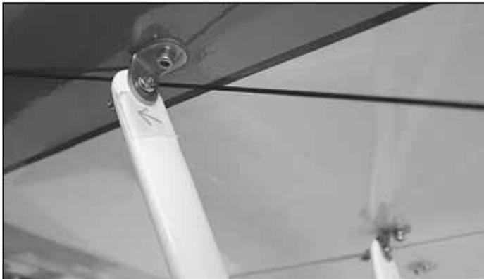
□ □ 10. Bring the elastic cord around the top of the forward strut and pull it back toward the fuselage. Glue the cord into the hole next to the hole you started with
