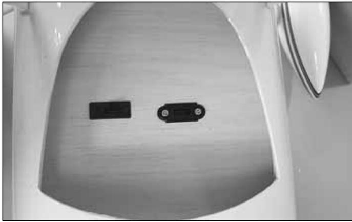
❑ 12. We installed the radio switch and the battery charge jack inside the front cockpit. Place a pilot in the cockpit as your guide for positioning the switch and charge jack.
