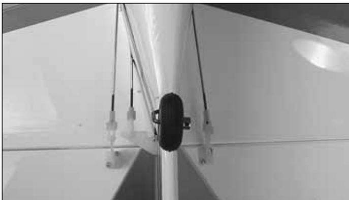
❑ 4. Install the two elevator pushrods using the same procedure used for the rudder. Be sure when installing the control horn on the right elevator that you install it so it does not conflict with the rudder control horn.
