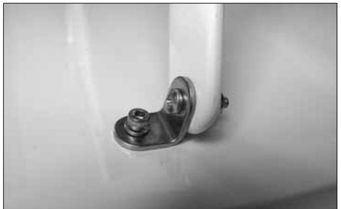
□ □ 6. Attach the strut to the bracket as shown with a 4-40 x 1/2" [13mm] phillips head screw, a #4 washer and a 4-40 nylon lock nut.
