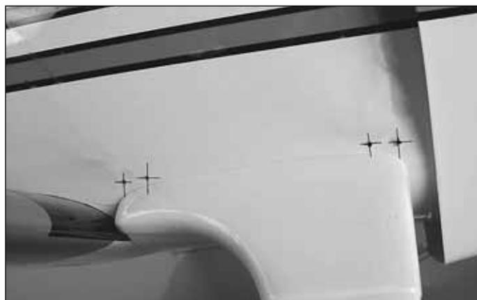
□ □ 8. Make two marks 1/2" [13mm] apart 1/4" [6mm] above the landing gear. Drill partially into the fuselage on each of the four marks 5/64" [2mm].
