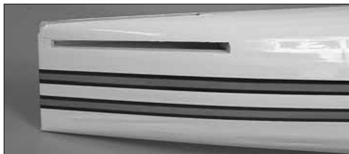
❑ 3. Cut the covering from the fuselage where the horizontal stabilizer fits into the fuselage.
