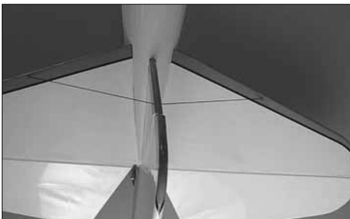
□ □ 6. Continue threading the cord through the hole in the leading edge of the stab on the opposite side of the fuselage.
