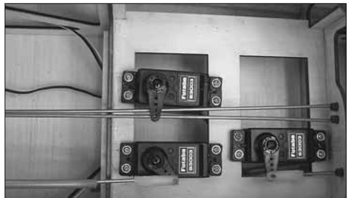
❑ 7. Place your elevator servo into the servo tray as shown, positioning the last hole of the servo arm over the inside pushrod wire. Drill a 1/16" [1.6mm] hole through each of the mounting holes. Remove the servo, then install and remove a servo mounting screw into each hole. Apply a couple drops of thin CA into the holes to harden the threads. When the glue has cured permanently, mount the servo to the servo tray.
