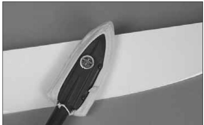
2. Carefully remove the tape and separate the ailerons from the wing and the elevators from the stab. If necessary, use a covering iron with a covering sock on high heat to tighten the covering. Apply pressure over sheeted areas to **thoroughly** bond the covering to the wood.
