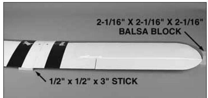
Before the glue cures, set one wing half flat on your bench. Insert the 1/2" x 1/2" x 3" [13 x 13 x 75mm] balsa block under the trailing edge of the wing that sits flat on the workbench. Block up the wing tip of the other wing half with the 2-1/16" x 2-1/16" x 2-1/16" [52 x 52 x 52mm] balsa block included in the kit. Put small weights on the wing half that is flat on the bench to keep it lying flat and leave the block under the wing tip of the other wing half while the glue cures.
