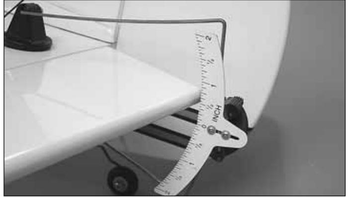
Use a Great Planes AccuThrow (or a ruler) to accurately measure and set the control throw of each control surface as indicated in the chart that follows. If your radio does not have dual rates, we recommend setting the throws at the **low** rate setting.
