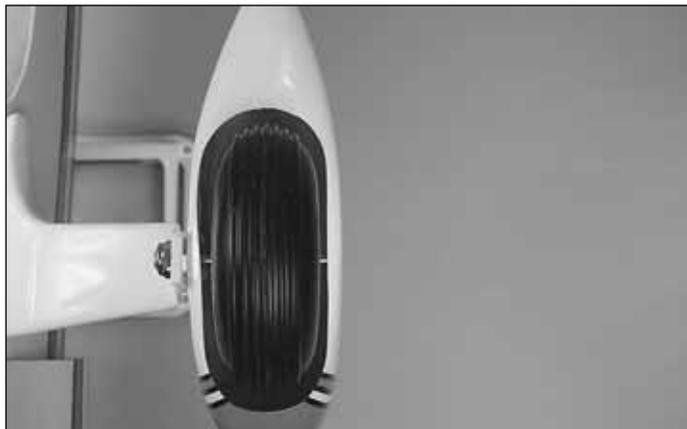
□ □ 7. Center the wheel in the wheel pant with the two wheel collars. Hold the collars in place with the screws. Mark the location where the screw contacts the axle. Remove the wheel pants, wheel and wheel collars from the axle. Apply a couple of drops of thin CA into the two holes you drilled in the wheel pant.
