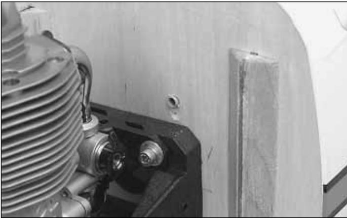
❑ 4. Drill a 3/16" [4.8mm] hole through the firewall in line with the throttle arm on the carburetor.
