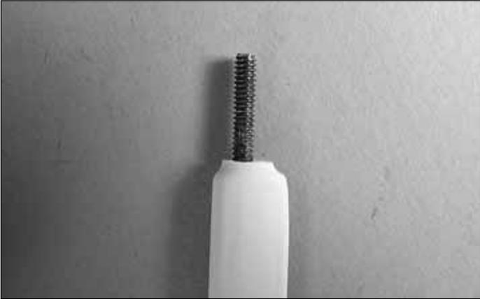
□ □ 6. Locate the **aileron connecting rod**. Cut the excess rubber coating to expose all of the threads.
