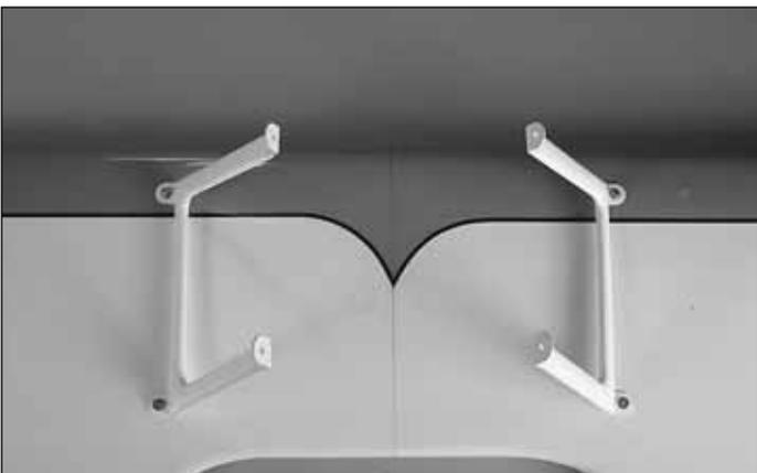
❑ 9. Install the center cabanes with 4-40 x 1/2" [13mm] socket head cap screws and #4 lock washers. Be sure you mount the cabanes as shown.
