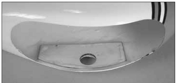
❑ 3. Sand the inside of the wheel pant on the side with the hole. Wipe the area clean with denatured alcohol. Mix a
