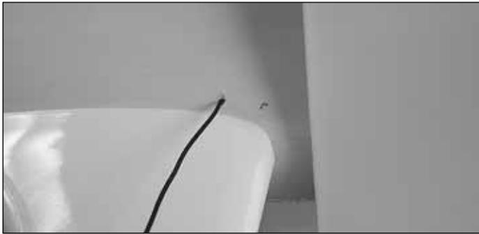
□ □ 9. Put a small drop of CA on the cord, then insert it into the hole shown.
