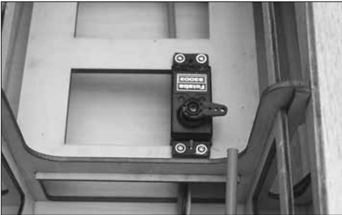
❑ 6. Place your throttle servo into the servo tray as shown. Drill a 1/16" [1.6mm] hole through each of the mounting holes. Remove the servo. Then install and remove a servo mounting screw into each hole. Apply a couple drops of thin CA into the holes to harden the threads. When the glue has cured permanently, mount the servo to the servo tray.
