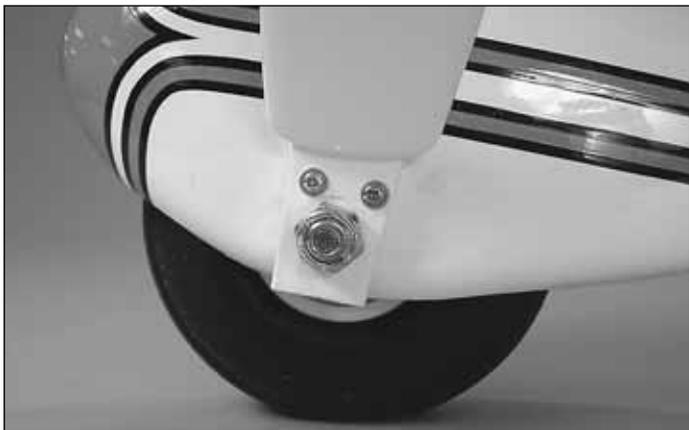
□ □ 6. Holding the wheel pant in that position, drill a 1/16" [1.6mm] hole through each of the mounting holes in the landing gear and into the wheel pant. Secure the pant to the landing gear with two #2 x 1/2" [13mm] screws and #2 washers.
