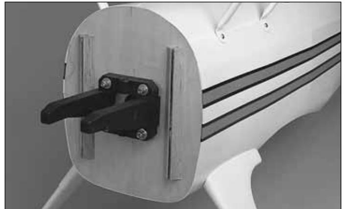
□ 1. Cut the tabs from the engine mount. Install the engine mount (inverted) to the firewall with four 8-32 x 1-1/4" [32mm] socket head cap screws, #8 flat washers and #8 lock washers.
