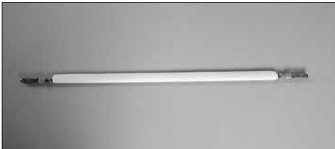
□ □ 7. Install a 4-40 nut, 4-40 metal clevis and a silicone clevis keeper on both ends of the connecting rod.
