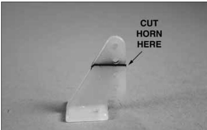
1. Locate two small nylon control horns. Cut them as shown.
