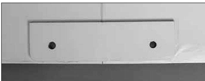
❑ 15. Glue the wing bolt plate to the wing using epoxy. Use small clamps to hold the wing bolt plate in position while the glue cures.
