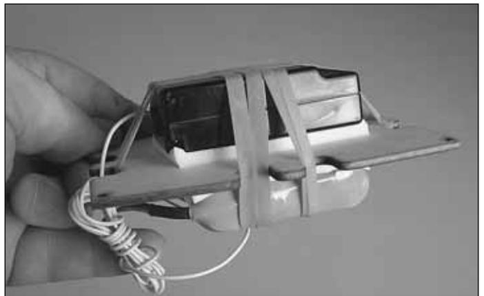
□ 11. On one side of the tray, place 1/4" [6mm] foam between the receiver and the tray. On the other side place 1/4" [6mm] foam between the tray and the battery pack. Use #64 rubber bands to hold the receiver and battery to the tray.
