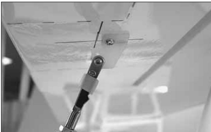
□ □ 8. Install one end of the connecting rod to the outer hole of the control horn on the aileron of the top wing.
