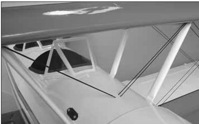
❑ 16. Cut four pieces of elastic cord 4" [100mm] long. Glue a cord into each of the four holes. Stretch the cord to the top of the cabane and glue the cord to the cabane with a small drop of CA.
