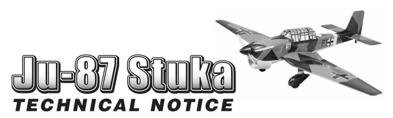
Before beginning the section titled *Install the Radio, Pushrods, & Control Horns* on page 18, make sure that the gray pushrod tubes exit the rear of the fuselage in the proper locations. The inner elevator and rudder pushrod tubes may exit the fuselage at the tail in the improper locations. To determine and/or rectify this problem follow these steps.
