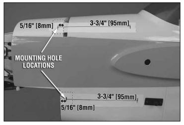
**On Page 22, Step 6:** The cowl mounting blocks may not be positioned as originally shown. Mark the block location 5/16" (8mm) in from the indented areas on the fuselage exterior (see above photo). Next, with the canopy hatch removed, view the blocks from the inside. Find and mark their centers on the outside of the fuselage.
