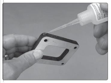
☐ 3. Glue the spacers together after accurately aligning them. Working in a well-ventilated area, use thin CA to thoroughly wet the spacers around the area of the bolt
