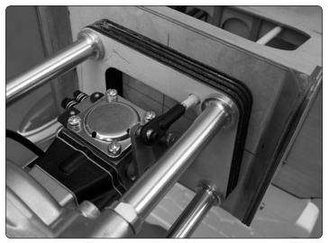
■ 9. Mount the engine. Use the generic servo tray to mount the throttle servo and hook up the throttle as shown and as specified in the instruction manual. The carburetor arm on the DLE 35cc is threaded for an M2 screw, so a DuBro Swivel ball link with 2mm hardware (DUBQ1769) was used on the front of the pushrod.
