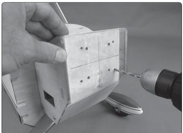
☐ 1. Use the engine mount template to mark, then drill #8 (.199" [5.1mm]) or 13/64" holes through the firewall – note that the top holes in the template are for both the 30cc and the 35cc DLE engines, but the bottom holes are different for each of the two.
