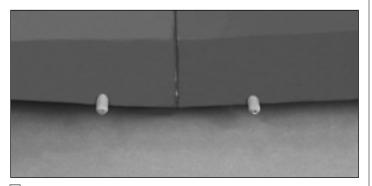
□ 6. Use 6-minute epoxy to glue the two 1-5/8" [41.3mm] wing dowels in the wing dowel holes. The rounded end should protrude from the wing approximately 1/2" [12.7mm].
