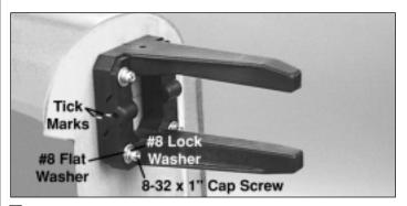
□ 5. Temporarily install the engine mount on the firewall with four 8-32 x 1" socket head cap screws, **#8 lock washers** and #8 flat washers. Do not tighten the screws all the way so you can adjust the mount.
