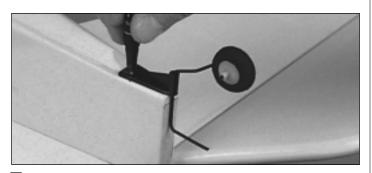
□ 5. Position the tailgear on the bottom of the aft end of the fuselage. Center the tailgear mount with the tailgear
