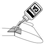
□ 2. Apply 6 drops of thin CA adhesive to both sides of each hinge in the elevator. Allow a few seconds between drops for the CA to wick into the slot.
