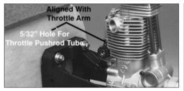
□ 9. Drill a 5/32" [3.9mm] hole through the firewall and the second former, in line with the throttle arm on the engine.
