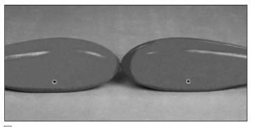
□ 3. Note that there is a bump (axle guide) on each side of the **wheel pant**. Trim one of the molded axle guides from each wheel pant. **Important:** Be sure to make a **left** and **right** wheel pant.
