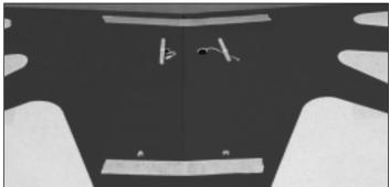
□ 5. Test fit the two wing halves together. The wing halves should seat together without any gaps and the front and back edges of each wing should line up with each other. Completely cover the exposed portion of the wing joiners, spars and root ribs with 30-minute epoxy. Slide the two
