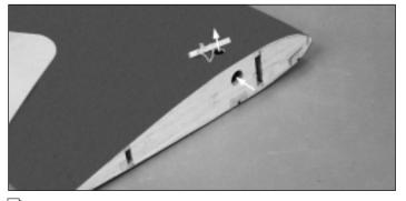
□ 2. Use a sharp hobby knife to cut the covering from the **servo cord exits** on the top of each wing half. Carefully untie the string from the stick at the root rib and route the string through the servo cord exit. Re-tie the strings around the stick.
