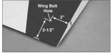
□ 3. Use a sharp hobby knife to cut the covering from the **wing dowel holes** in the leading edge and the **wing bolt holes** at the trailing edge of each wing half. The wing dowel holes are approximately 2" [50.8mm] from the wing root. The wing bolt holes are approximately 2" [50.8mm] from the wing root and 2-1/2" [63.5mm] from the trailing edge.
