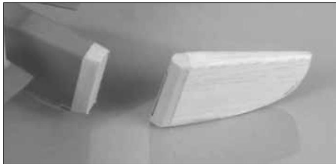
❑ 5. Shape the balsa on the front of the rudder to match the shape of the rudder.
