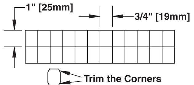
❑ 2. Cut six 3/4" x 1" [19 x 25mm] hinges from the 2" x 9" [50 x 230mm] CA hinge strip. Snip the corners off so they go in the hinge slots more easily.
