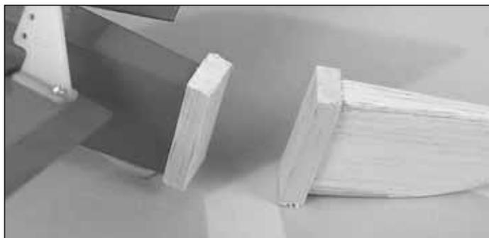
❑ 3. Glue 1/4" x 1/2" x 1-1/2" [6 x 13 x 38mm] balsa to the TE of the fuse and LE of the rudder
