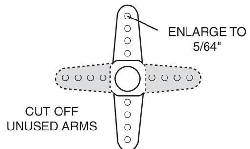
❑ 3. Make a two-sided servo arm. Enlarge the holes in the arm with a Hobbico Servo Horn Drill (or a #48 or 5/64" [2mm] drill bit) so the aileron pushrods will fit.
