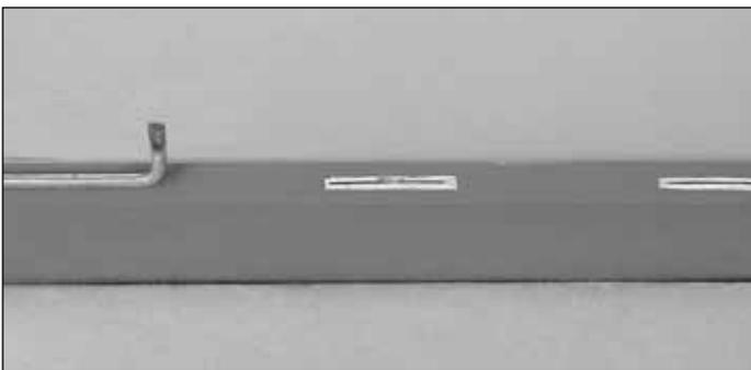
❑ 5. Cut a small strip of covering from both sides of each hinge slot. If not done the covering may interfere with the penetration of the CA into the slot and the free movement of the aileron.
