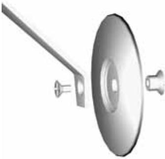
❑ 1. Mount the wheels to the landing gear with the 6-32 x 1/4" [6mm] bolts and axle as shown in the sketch.
