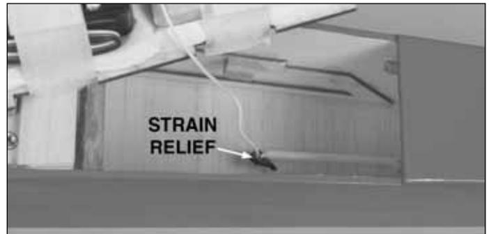
❑ 10. Using an arm cut off the aileron servo, put a strain relief on the antenna and feed the antenna through the antenna tube. The excess antenna hangs out of the bottom of the airplane. **DO NOT CUT THE ANTENNA.**
