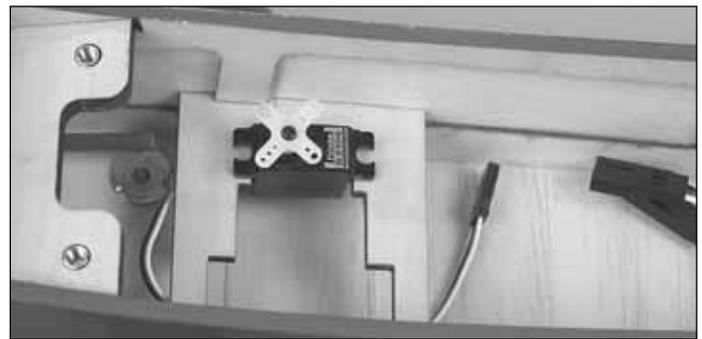
❑ 21. Determine the size of the throttle servo you are going to use. Using the photos as a reference, mount the throttle servo in the tray so that it aligns with the throttle pushrod. Fit the tray in the airplane, being sure to leave at least a 1/16" [1.6mm] gap between the servo and the landing gear rail. Glue the servo tray securely to the fuse sides.
