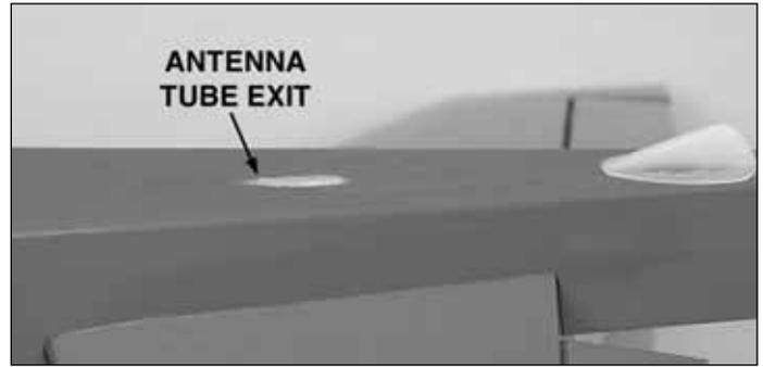
❑ 9. Remove the covering from the antenna tube exit at the rear of the fuse.
