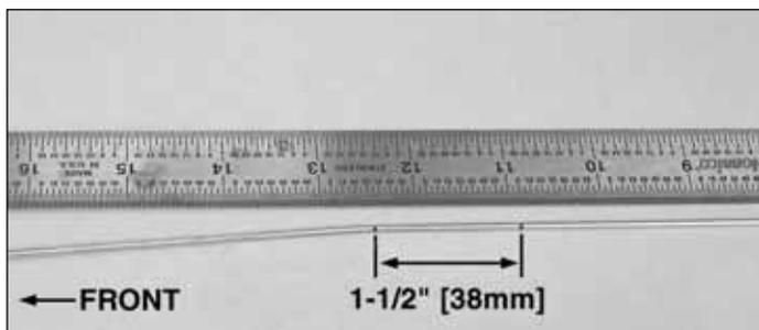
☐ 10. Remove the pushrods. Make another mark 1-1/2" [38mm] in front of the first. At the forward mark make a slight bend. Reinstall the pushrods and attach the clevises. **Note:**
