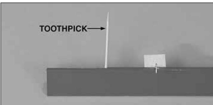
❑ 6. Stick a pin through the center of each hinge. Fit the hinges into the ailerons. Use a toothpick to push epoxy into the torque rod hole in the aileron. Fit the ailerons to the wing
