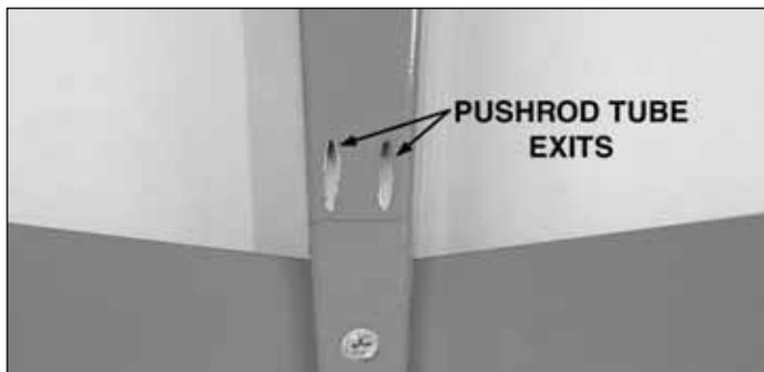
☐ 8. Trim the covering from the pushrod tube exits that are in front of the V-tail on top of the fuse.
