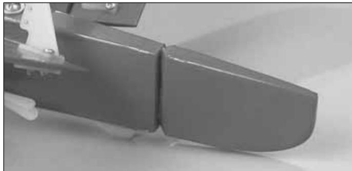
❑ 7. Cut the hinge slots and mount the rudder with one long hinge.
