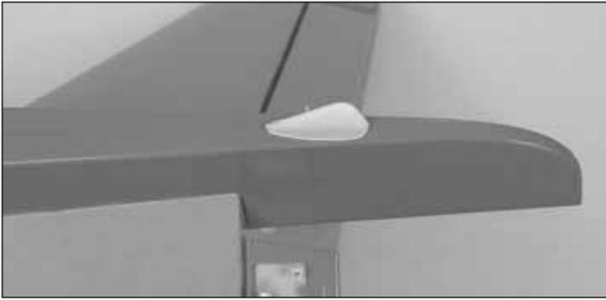
❑ 3. Remove the covering from the two tail-skid mounting holes on the bottom of the fuselage. Enlarge the tail-skid mounting holes with a 1/8" [3mm] drill. Glue the nylon tail-skid in place with medium CA.
