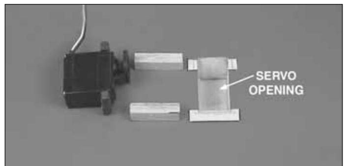
❑ 1. Test fit the aileron servo and the 3/8" x 3/8" x 1-1/4" [9.5 x 9.5 x 32mm] basswood aileron servo rails in the wing. Mark the covering around the rails. Remove the covering from the contact area between the rails and the wing. Epoxy the rails to the wing.
