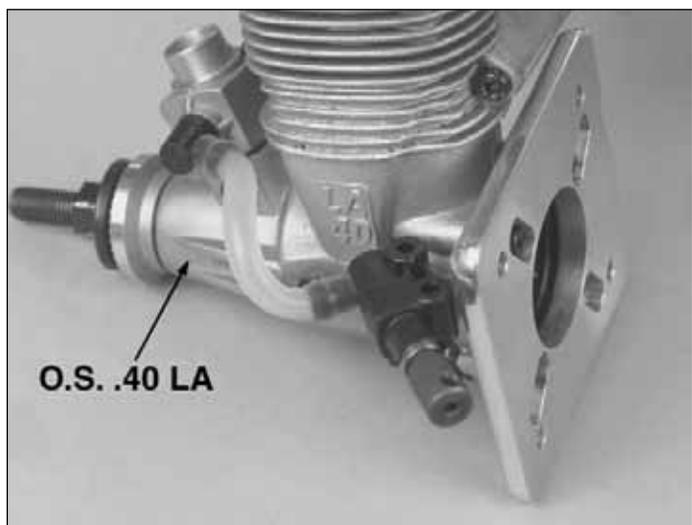
☐ 1. Remove the bolts from the engine backplate. Test fit the mount to the engine. If necessary, file the mount to accommodate the needle valve (required if using the O.S.® .46 FX), or relocate the remote needle to the engine mounting lug (required for the O.S. .40 LA), as shown in the photographs.
