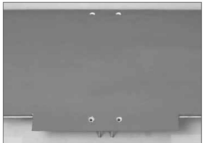
❑ 1. Looking at the bottom of the wing as shown in the top photo (the aileron torque rods protrude from the bottom of the wing), cut the covering from the servo opening and the bottom of the four wing bolt holes. Turn the wing over and cut the covering from the top of the 4 bolt holes.
