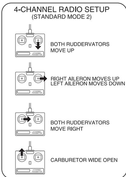
3. Make certain that the control surfaces and the carburetor respond in the correct direction as shown in the diagram. If any of the controls respond in the wrong direction, use the servo reversing in the transmitter to reverse the servos connected to those controls. Be certain the control surfaces have remained centered. Adjust if necessary.
