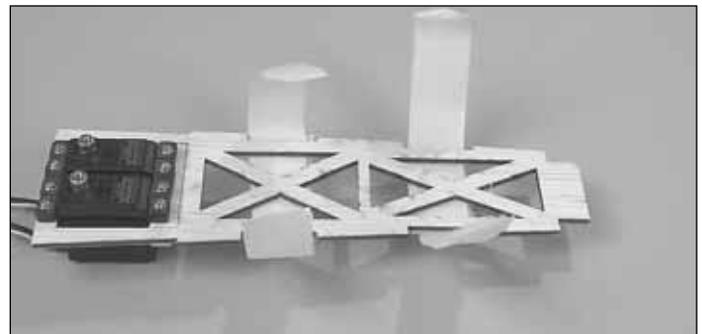
❑ 4. Glue the hook and loop material to the bottom of the servo tray.
