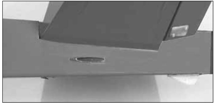
❑ 12. Glue the tube to the fuse with thin CA. Allow the CA to cure and then cut off the excess tube.
