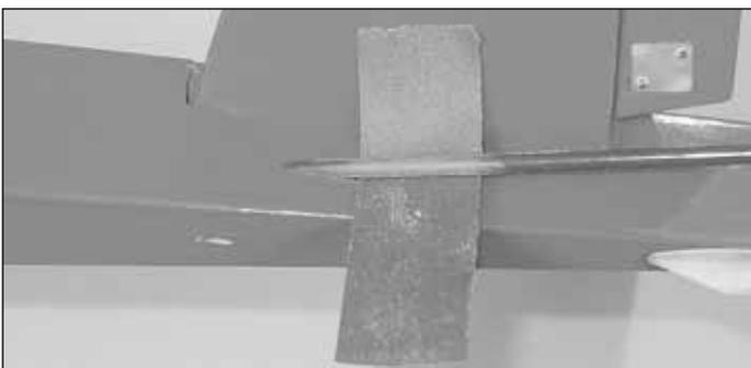
❑ 11. Mark the pushrod tube where it exits the fuse. Use coarse sandpaper to roughen the pushrod tube from the mark to 1-1/2" [38mm] forward of the mark.
