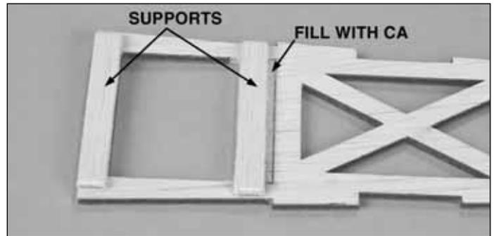
❑ 2. Glue the V-tail servo supports to the servo tray. The side you glued the supports onto is now the bottom. **Note:** If you used servos smaller than standard, fill the cut lines with medium CA.
