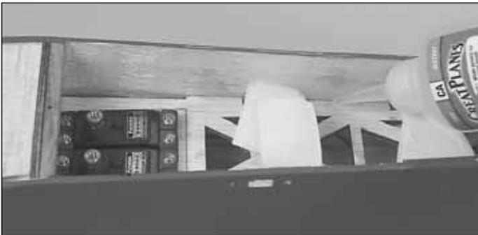
❑ 7. Glue the servo tray to the fuse with thin CA, then with thick CA.
