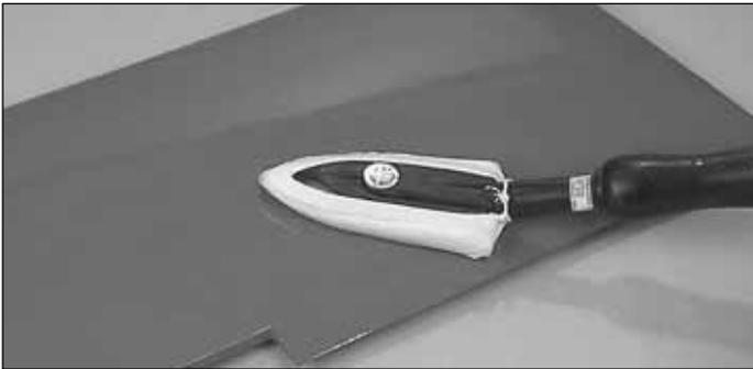
❑ 2. Remove the masking tape and separate the ailerons from the wing and the ruddervators from the V-tail. Where necessary, use a covering iron with a covering sock to tighten the covering that may have loosened during storage or from removing the masking tape. Apply pressure over sheeted areas and the servo openings to **thoroughly** bond the covering to the wood.
