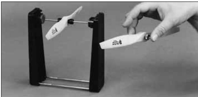
Carefully balance your propeller and spare propellers before you fly. An unbalanced prop can be the single most significant cause of vibration that can damage your model. Not only will engine mounting screws and bolts loosen, possibly with disastrous effect, but vibration may also damage your radio receiver and battery. Vibration can also cause your fuel to foam, which will, in turn, cause your engine to run hot or quit.
