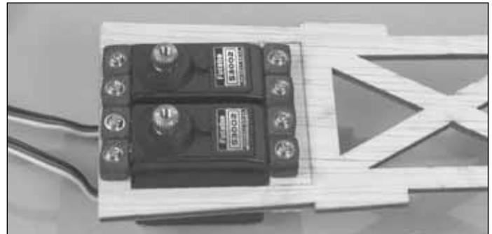
❑ 3. Fit the tail servos into the servo tray. Drill 1/16" [1.6mm] holes for the servo screws and apply thin CA to the holes. Mount the servos to the tray with the screws provided with the radio gear.
