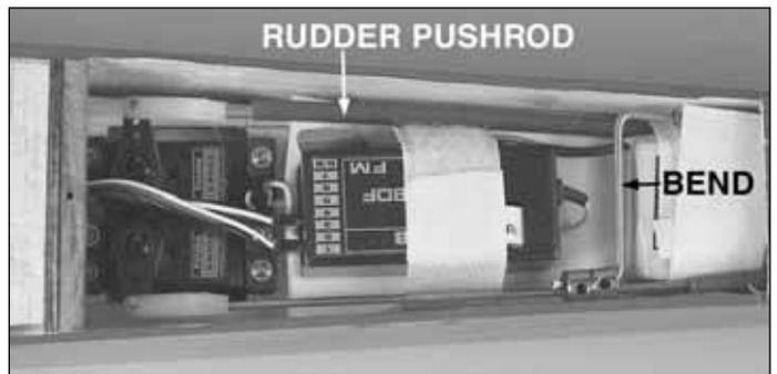
❑ 14. Attach the pushrods to the ruddervators. Bend the right ruddervator pushrod as shown. Connect the two ruddervator pushrods together with two 5/32" [4mm] wheel collars.
