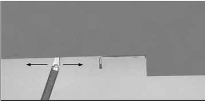
❑ 3. Test fit, but do not glue the aileron to the wing with the hinges. If you have difficulty inserting the hinges, insert a #11 blade into the slot and **carefully** move it back and forth to slightly widen the slot.
