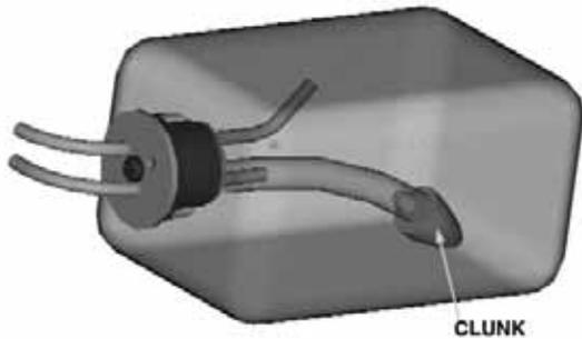
❑ 9. Arrange the stopper and tubes as shown and insert them into the tank. Tighten the screw to expand the stopper, thus sealing the tank. Be certain the fuel line weight (clunk) at the end of the fuel line inside the tank does not contact the rear of the tank. Otherwise, the line may become stuck above the fuel level and discontinue fuel flow.
