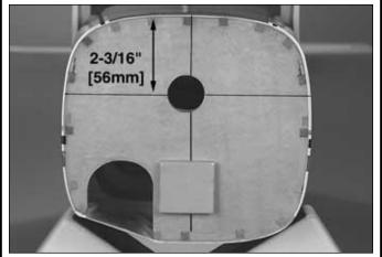
2. Draw a **horizontal** line on the firewall 2-3/16" [56mm] from the top of the fuselage. Draw a **vertical** line on the firewall along the left side of the top and bottom stringers as shown in the photo.
