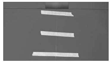
4. Slide the wing joiners into one wing, then slide the remaining wing onto the joiners. Hold the two wing halves together with masking tape. Set the wing aside and allow it to cure for at least two hours before handling the wing.
