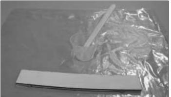
Locate the two plywood wing joiners and glue them together with 6-minute epoxy. Clamp them together and wipe off all excess epoxy.
