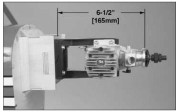
$\Box$  4. Position the **engine** on the mount so the engine drive washer is 6-1/2" (165mm) from the firewall. This will provide the correct clearance between the spinner and the cowl.
