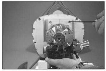
□ 6. Install the four 8-32 blind nuts in the firewall in the holes you just drilled. Install the mount onto the engine with the four mounting bolts through the mount and into the back of the engine. Next mount the engine to the firewall using the four 8-32 x 1" (25 mm) socket head cap screws.
