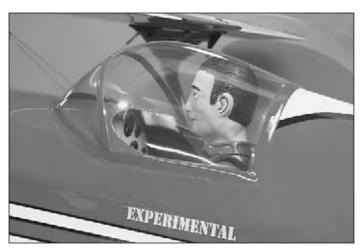
□ 3. Carefully cut the excess plastic away from the **painted** canopy. Glue the canopy into position using R/C-56 Canopy Glue (JOZR5007).
