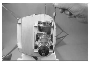
□ 5. Using your Dead Center Hole Locator again, mark the hole locations on the engine mount. Drill #29 (or 9/64") holes through the engine mount at the marks you made, then tap 8-32 threads into the holes. Mount the engine to the mount with four 8-32 x 3/4" Socket Head Cap Screws and #8 washers.
