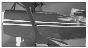
□ □ 11. The placement of the struts in relation to the top wing is determined in the following manner. Measure the distance of the top rear tip of both interplane struts to the trailing edge of the top wing. If necessary, twist the top wing in order to make both distances equal. When satisfied with the alignment, mount the top of the interplane struts to the brackets installed in the top wing using the same method as the bottom of the interplane struts.
