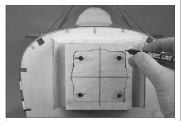
□ 5. Glue the two halves of the plywood mount together using epoxy. Make sure that you assemble the two halves
