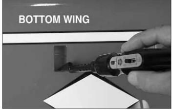
□ □ □ 7. Cut the covering 1/8" (3mm) inside the opening in this wing half for the **aileron servo**. Use a trim iron to seal the covering to the edges of the opening.
