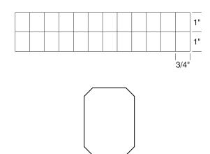
□ 3. Cut twenty-one 3/4" (19mm) x 1" (25mm) **hinges** from the **CA hinge strip**. Snip off the corners as shown so they go in easier. Insert three of the hinges into the aileron hinge slots of each wing half. The rest of the hinges are for the elevators and rudder.
