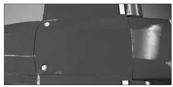
$\Box$  5. After removing the covering use epoxy to glue the belly pan to the wing. Allow the epoxy to cure completely. Be very careful not to get glue into the area where the belly pan fits into the fuselage; glue it only to the wing itself.
