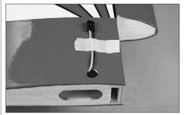
□ □ □ □ 9. Connect a 12" (305mm) servo extension wire (HCAM2711) to an aileron servo lead and secure it with
