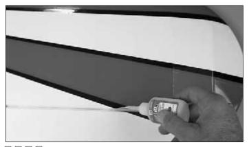
□ □ □ □ 6. Apply six drops of **thin CA** to the top and bottom of each hinge. Do not use CA accelerator. After the CA has fully hardened, test the hinges by pulling on the aileron.
