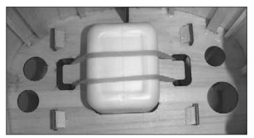
□ 2. Install the fuel tank so the neck fits through the existing hole in the former behind the engine-mounting box. Be certain
