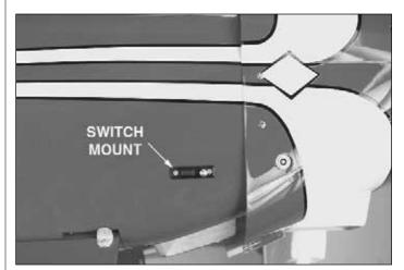
□ 3. A Great Planes Switch & Charge Mounting Set (GPMM1000) was used to mount the switch and charge jack into the fuselage as one unit.
