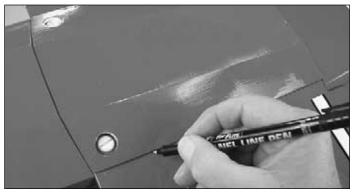
□ 3. Place the belly pan on the bottom of the lower wing allowing it to center over the wing bolt holes (you may want to install the wing bolts to hold the belly pan in place as shown in the photo) and also match up to the bottom of the fuselage in front and behind the wing. When satisfied with the fit, mark the outline with a Top Flite Panel Line Pen (TOPQ2510).
