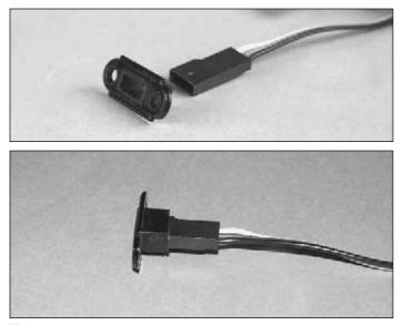
□ 5. Using a Hobbico Pro Series 24" Extension (HCAM2200) insert the female end into the back of the receptacle unit as shown in the photographs above.
