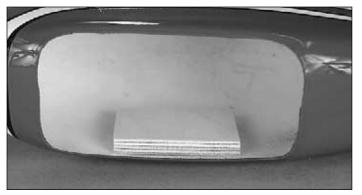
□ □ 5. Locate the four  $3/32"(2.4 \text{ mm}) \times 1"(25 \text{ mm}) \times 2"(51 \text{ mm})$ **plywood doublers** for mounting the wheel pants and the four  $3/32"(2.4 \text{ mm}) \times 1"(25 \text{ mm}) \times 1"(25 \text{ mm})$  **plywood wheel pant bearing blocks.** Make two sets as shown in the above photograph by gluing them together using 6-minute epoxy.
