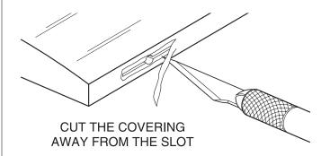
$\Box$  2. Use a sharp #11 blade to cut a strip of covering from the aileron hinge slots in **all four wing halves** and **ailerons**.
