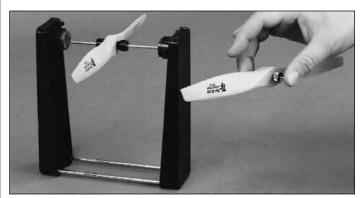
Carefully balance your propeller and spare propellers before you fly. An unbalanced prop can be the single most significant cause of vibration that can damage your model. Not only will engine mounting screws and bolts loosen, possibly with disastrous effect, but vibration may also damage your radio receiver and battery. Vibration can also cause your fuel to foam, which will, in turn, cause your engine to run hot or quit.
