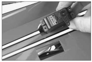
□ 3. With the servos in position in the fuselage, drill 1/16" (1.6mm) holes in the fuselage for the servo mounting screws. Using the technique described on Page 8, mount the elevator servo using the supplied screws.
