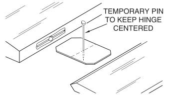
□ 9. Install the hinges into the stab and then test fit both of the **elevators**. If the hinges don't remain centered, stick a pin through the middle of the hinge to hold it in position.
