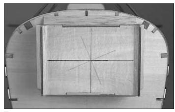
□ 1. Notice the marks on the firewall. Extend the **horizontal** and **vertical** lines with a pen to see them more clearly as shown in the photo above. **Disregard any other marked lines on the firewall**.
