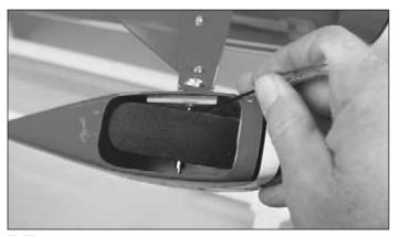
□ □ 11. Next fit one of the supplied wheels onto each shaft followed by another 5/32" wheel collar with a 6/32" setscrew installed. Center the wheels within the wheel pants and temporarily tighten the 6/32" setscrews in the wheel collars to hold them in place.
