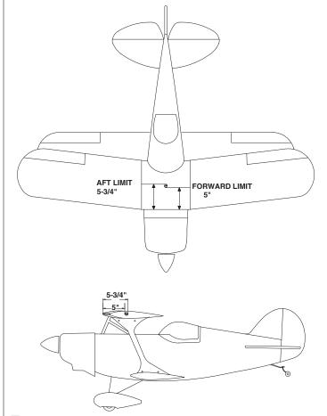
$\Box$  2. With the wings attached to the fuselage, all parts of the model installed (ready to fly) and an empty fuel tank, lift the model with your finger tips at the balance point you marked.
