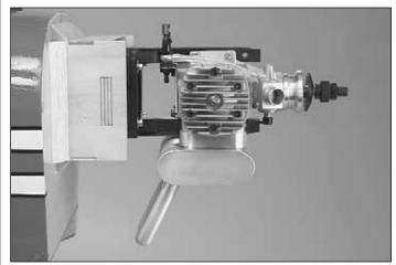
□ 6. Test fit the **muffler** to be used on your engine. The **O.S. 1.60 FX (OSMG0661)** is shown in this manual. Bisson Custom Mufflers produce a **Pitts Style Muffler (BISG4116)** that is designed specially to fit this engine and is shown in the photo above.
