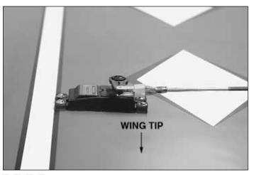
□ □ □ 11. The **servo arms** for the aileron servos are installed so that they point outboard toward the wing tips as shown in the above photograph. This is necessary for proper function.
