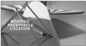
□ 6. The photograph above, looking back from the front of the airplane, shows the placement of your modified receptacle. Make sure that you can access the screws and that it is placed to avoid the spars and formers in this area.
