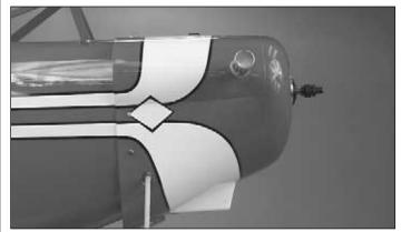
□ 5. You will need to cut other access holes in the cowling for things like the fueling valve, needle valve, and glow driver access to start the engine. Use this same method to locate these holes. When finished you will have accurate locations for these functions.
