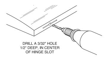
$\Box$  1. Drill a 3/32" (2.4mm) hole, 1/2" (13mm) deep in the center of each hinge slot to allow the CA to "wick" in. Followup with a #11 blade to clean out the slots. **Hint:** If you have one, use a **high-speed rotary tool** to drill the holes.
