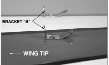
□ 6. Again, using the technique described on Page 8, install the four 110-degree compound bend metal brackets (Bracket B as shown above) in place with four #4 x 1/2" (13mm) wood screws as shown in the photos above.
