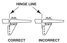
□ 4. Position the elevator control horns directly in line with the servo arms and with the hinge alignment as shown above. At both locations mark and drill the four 1/8" (3mm) holes for each of the horns. Saturate these holes with thin CA, wiping away any residue and allow it to fully harden. Then re-drill the holes to allow the screws to pass through easily. Mount the control horns and back plates to the two elevators with eight 4-40 x 3/4" (19mm) socket head screws.
