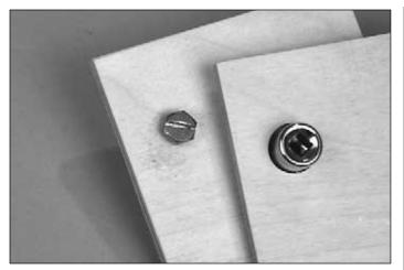
□ 3. Place the four 1" (25 mm) x 1/4" (6 mm) x 20 engine mounting bolts (not supplied) into the rear plate. Place a socket that fits these bolts over the bolt heads and draw a line around all four as shown in the above photograph. Remove the wood from inside these four marks on the rear plate only. Doing this will allow the socket to fit inside the rear plate and countersink the bolt heads when the two halves are assembled.
