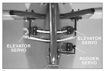
□ 7. The photo above references the completed installation of elevator and rudder servos, control horns, and pushrods. Looking forward from the rear of the fuselage you can see that the rudder servo is placed below the elevator servo.
