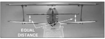
□ 4. Stand ten to fifteen feet behind the model and view the stab and wings. If the stab and wings align with each other, proceed to the next step. If the stab and wing do not align, remove the stab and carefully sand the "high side" of the slot in the fuse where the stab fits until the stab aligns with the wing. If you needed to make any adjustments, reposition the stab into the fuselage, making sure the alignment is correct.
