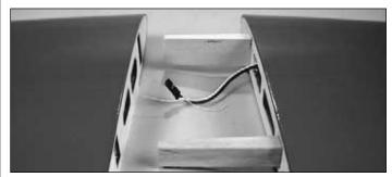
□ □ 3. When satisfied with the fit, glue the joiners into the left wing panel using 30-minute epoxy. Place a generous amount of epoxy into the inside of the pockets and on the half of the joiners that will be inserted into the wing pockets. When the epoxy has cured, tie the string in the center section to the aileron servo extension wire as shown in the photo above.
