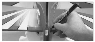
$\Box$  5. Using a felt-tipped pen, carefully mark the location of the fuse sides on both the top and bottom of the stab. Remove the stab from the fuselage and cut 1/8" inside the line in order to remove the MonoKote covering from the stab. Use a hot knife or sharp hobby knife with the same
