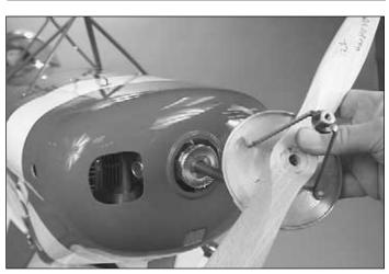
□ 1. The **aluminum spinner** supplied with this model is a new and innovative design, which is universal and eliminates the need for adapter nuts. To assemble the spinner, hold the backplate and propeller (not supplied) together as one unit and place onto the drive shaft.
