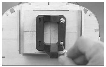
□ 2. After removing the spreader bars from both **engine mount** halves, fit the two halves together using the engine to space the width properly. Notice that when you find the proper width for your engine, the tick marks on the two halves of the engine mount will no longer line up with each other. Measure the distance between the two tick marks and mark the center location between these tick marks. This location will be used to properly align the engine mount with the firewall markings.
