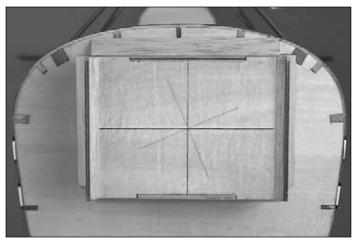
□ 4. The existing firewall on the model has centering marks on the face of the firewall. Highlight and extend these lines with a felt tipped pen as shown in the above photograph.
