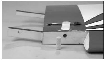
□ 3. After the epoxy has cured, sand off any excess glue and test fit the two lower wing joiners into the two wing halves as shown above. Note that the two 3/8" (9.5mm) wood dowels will be placed into the front of the wing. Test fit them into the wing at this time also. Make sure the wing halves fit together properly and form a good fitting joint. If the wing does not fit properly, carefully sand the tips of the wing joiners until you get the proper fit.
