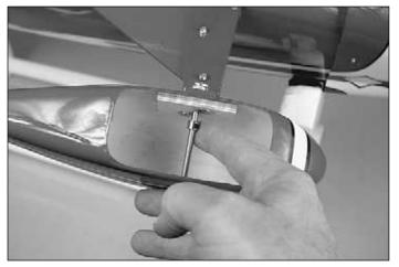
$\Box$   $\Box$  10. Insert the axle shaft through the wheel pant and plywood doubler while at the same time slipping one 5/32" wheel collar with a 6/32" setscrew installed onto the shaft.
