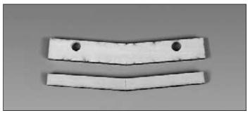
□ 2. Use epoxy to glue the joiners together to form two plywood joiners as shown.
