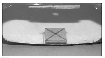
□ □ 7. Mark the location of the center of the plywood wheel pant bearing block you prepared earlier as shown in the photograph and drill a 5/32" (4mm) hole at this location.
