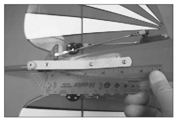
□ 8. To install the **tail gear**, position it so the forward edge is 4-1/2" (115 mm) from the aft end of the fuselage as shown in the above photo. Mark the location of the holes in the tail gear on the fuselage and drill two 3/32" (2.4 mm) holes. Be sure to again use the method of installing screws into the model described on page 8 and install the gear with two #4 x 1/2" (13 mm) Phillips head wood screws.
