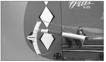
□ Use a **Great Planes AccuThrow Deflection Gauge** (GPMR2405) or a ruler to accurately measure and set the control throw of each control surface as indicated in the chart that follows. If your radio does not have dual rates, we recommend setting the throws at the **low** rate setting.
