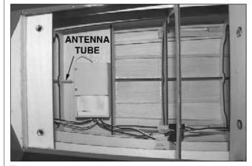
□ 2. To mount the receiver we used a Great Planes Receiver Guard Protective Case (GPMM1010) and mounted it to the bottom of the cockpit floor. There is a tube installed for the receiver antenna that is located at the bottom of the cockpit floor as shown in the above photograph. The Receiver Guard should be mounted first, then servo leads attached to the receiver. Then simply insert the receiver antenna into the tube.
