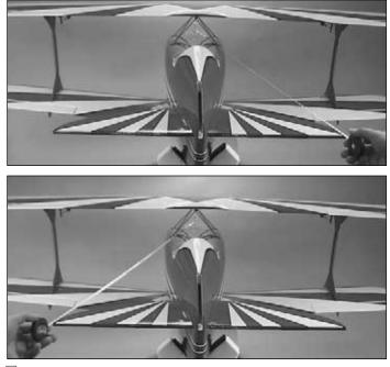
□ 3. With the wings still attached, place the model in a building stand such as a Robart Super Stand II (ROBP1402). Place a T-pin on the center line of the fuse at the forward most former. Measure from the pin to each tip of the stab. A Hobbico Retractable Fabric Tape Measure (HCAR0478) works well for this step. The distance from the pin to the stab tips needs to be equal on both sides.
