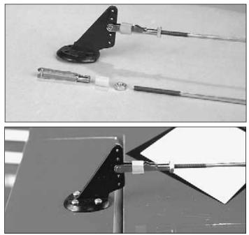
□ □ □ 13. Install a metal clevis, a 4-40 hex nut, and a clevis retainer on the 4-40 x 12" (305mm) threaded one end pushrod approximately 15 turns. Remember to use Great Planes Pro Threadlocker (GPMR6060) on these clevises and hex nuts after the radio is set up and control throws have been finished later on in this manual.
