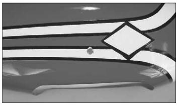
$\Box$   $\Box$  4. Look closely at the **painted fiberglass wheel pants** and you will notice there is a mark which indicates the correct position for the 5/32"(4 mm) hole to be drilled to allow the axle shafts to pass through.
