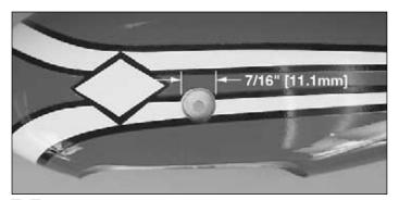
□ □ 6. Use a rotary tool or a drill to carefully create a 7/16"(11.1mm) clearance hole in the fiberglass wheel pant and plywood doubler as shown in the above photo for the axle unit base to fit into. Do not make this hole deeper than 9/64" (3.6 mm).
