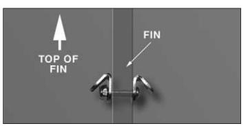
□ 4. Locate three 4-40 x 5/8" (15.9 mm) Phillips Head Machine Screws, three 4-40 stop nuts, and eight 70-degree metal brackets as shown in the photograph. Mount six brackets at the three drilled locations; two brackets are placed on top of the stab and two under it. The proper installation is shown in the photographs.
