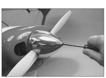
$\Box$  3. Place the spinner cone over the blades of the propeller and secure it with the supplied bolt.
