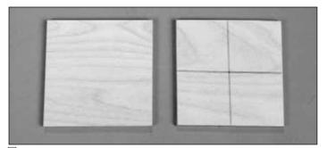
□ 1. Since this engine mounts with bolts from the rear of a traditional firewall, we will make a plywood mount to be attached to the engine. After this mount is attached to the engine it will then be mounted to the existing firewall. First of all make two 4" [102mm] x 4" [102mm] x 1/4" [6 mm] plywood mounting plates [not supplied]. Draw center marks
