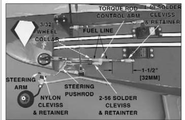
□ 10. In order to make the ground steering as positive as possible we are using a 2-56 pushrod extended from the rudder control rod to the tail wheel steering arm. This is shown in the above photograph. It is assembled by first removing the rudder pushrod, metal clevis, clevis retainer and hex nut from one end of the assembled pushrod.
