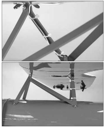
□ 7. The photographs above illustrate the Y-harness plugged into the receptacle. You can secure and hide the wire on the cabane with zip ties, Velcro, tape, or just leave it loose depending on your preference. Use a Y-harness (FUTM4130) to plug into your receiver. Plug the extension from your modified receptacle to one side of the Y-harness and the other side will be available when you attach the bottom wing and plug the bottom wing aileron servos into it.
