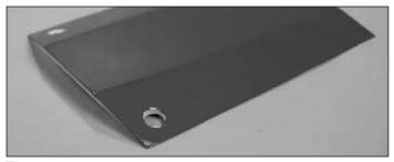
□ 2. Locate the belly pan and cut the MonoKote from the two holes which allow access for the wing bolts. Saturate the exposed wood with thin CA to make it stronger, and paint this area after the CA has cured to make it fuel proof.
