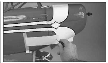
$\Box$  4. Repeat this process at the locations of the other five cowl mounting blocks. Mount the cowl using six #2 x 1/2"(13 mm) Phillips head screws and six #2 flat washers.
