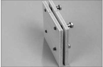
□ 2. Place the front side of the front plate (the one with the center marks) against the back of the engine and mark the location of the mounting holes with the engine centered on the mount. Also draw the outline around the back of the engine as shown in the photograph. **Note**: Depending on the muffler used you may need to relieve a portion of the mount to accommodate your muffler. Drill 1/4" [6mm] holes in these four locations through both plates.
