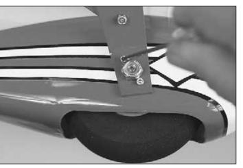
$\Box$  12. Install the 4/40 x 5/8" (15.9 mm) Phillips Head Machine Screws through the holes in the landing gear and into the blind nuts installed inside the wheel pant.
