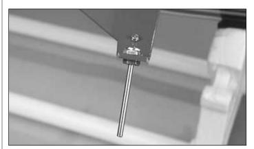
□ □ 8. Install the axles onto the landing gear, making sure the **stop nuts** are securely tightened.
