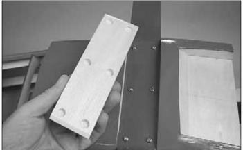
□ 2. Place the **landing gear cover** on top of the landing gear itself and press on it firmly in order to mark the location of the six truss head screws. Using a drill or a rotary tool, make clearance holes for the heads of the six screws. You may glue this cover into place or attach it with landing gear straps in order to retain access to the landing gear and its hardware if you wish.
