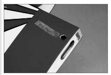
□ □ 8. Cut the covering away from the hole in the top of the bottom wing halves and feed the string, which is taped to the root rib, through the hole in top of the wing. Re-tape it securely near the hole. This step is different for the two top wing halves. There is one hole in the center of the top wing center section. Remove the covering from this hole also.
