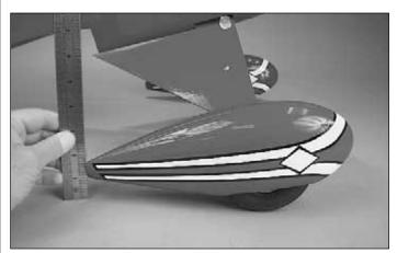
□ □ 9. Temporarily place the wheels into the wheel pants and slip them onto the axle shaft. As shown in the above photograph, set the model on a flat surface and position the aft end of the wheel pants 1" (25mm) above the surface. Mark the locations, on the wheel pant, of the two holes drilled in the landing gear while the aft end of the pants are still elevated 1" (25mm) off your flat surface.
