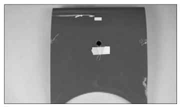
□ 1. If you haven't already, cut the covering away from the hole in bottom of the top wing center section and feed the string, which is taped to the sheeting, through the hole in bottom of the top wing center section. Retape it securely near the hole.
