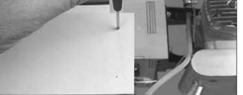
□ 2. After the epoxy has cured cut a piece of a file folder, index card, or any similar material and securely tape it to the side of the fuselage so that it covers one of the mounting blocks. Find the center of the mounting block and place a mark on the card taped to the fuselage.
