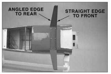
□ 1. To mount the **main landing gear** set it into place using the above photograph for the proper orientation and mark the location of the six holes drilled in the landing gear on the landing gear plate. Using the technique described on Page 8, mount the landing gear using the six # 8 x 5/8" (16 mm) truss head screws.
