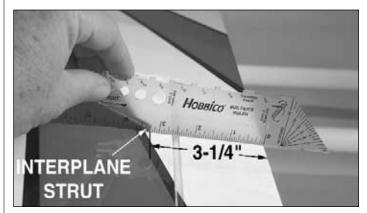
$\hfill \Box$  10. For location of the interplane struts on the bottom wing, measure from the TE of the aileron to the rear tip of
