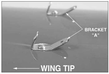
□ 4. Again, using the technique described on Page 8, install the four 70-degree compound bend metal brackets (Bracket A, as shown in the diagram) in place (two on each wing panel) with four  $#4 \times 1/2"$  (13mm) wood screws as shown in the photo above. The orientations of these brackets are shown in the photograph.
