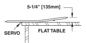
After properly fitting the wing halves together check for the correct dihedral angle. Place one wing panel on a flat surface and measure the distance from the elevated wing tip to the tabletop. This distance should be 5-1/4" (135 mm). **Note:** You will need to hang the aileron servo off the edge of the table in order to get the wing flat on the table as shown in the sketch above.
