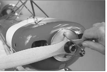
□ 2. Place the drive washer and the propeller nut onto the drive shaft. Tighten the nut securely with a box-end wrench of the correct size to fit your engine. Next install the lock nut, again with a box-end wrench.
