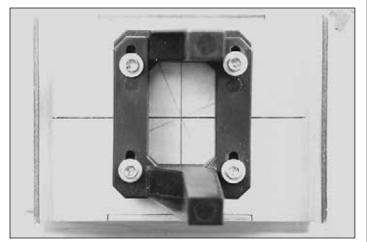
□ 3. Drill four 7/32" (5.6mm) holes through the firewall at the marks. Apply 30-minute epoxy to the four **8-32 blind nuts**, being careful not to get the glue into the threads and place them into the holes on the back of the firewall. Attach the engine mount to the firewall with four 8-32 x 1" (25mm) socket head cap screws and #8 flat washers. This will draw the blind nuts into the back of the firewall. Allow the epoxy to cure.
