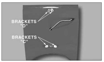
□ 2. Using the technique described on Page 8, install two 90-degree metal brackets (Bracket D, as shown above) into the pre-drilled holes in the front of the bottom of the top wing center section with two #4 x 1/2" (13mm) wood screws. Mount two 90-degree compound bend metal brackets (Bracket C, as shown above) using two #4 x 1/2" (13mm) wood screws. The cabane struts and flying wires will attach to these "C" brackets in a later step.
