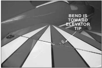
$\Box$  6. The brackets that are mounted on the stab have the "bend" toward the outboard end of the stab as shown in the photograph above.
