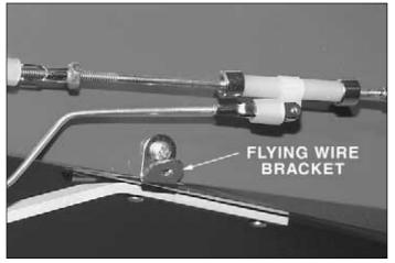
□ 7. Mount the brackets at the bottom of the fuselage, with the "bend" to the bottom as shown in the photograph above, use two #4 x 1/2" Phillips head wood screws to attach the brackets using the procedure described on page 8.
