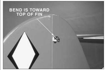
□ 5. Notice that the brackets are mounted on the fin as shown with the indicated "bend" at the top as shown in the photograph above.
