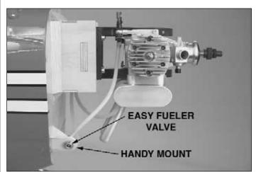
□ 3. Run the fuel line to the needle valve or if you are using an **Easy Fueler Valve** (GPMQ4160) as shown in the photograph above, attach the fuel line to the valve first and then the needle valve. Attach the vent line to the pressure tap on the muffler. The Easy Fueler Valve can be mounted easily by using a **Great Planes Handy Mounts** (GPMQ6000) which is also shown in the photograph.
