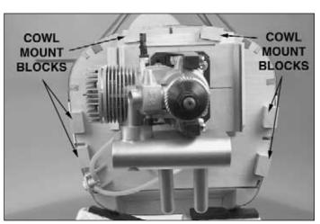
□ 1. Mark the location of the six **cowl mounting blocks** on the forward fuselage former as shown in the photograph above. Using 80-grit sandpaper, rough up the surface in this area in order to allow a better glue joint. Use epoxy to glue the six cowl mounting blocks to the front of the fuselage in the locations shown in the above photograph. After the epoxy cures, fuelproof these blocks using additional epoxy.
