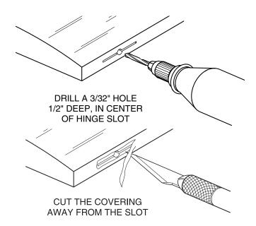
□ 8. To attach the elevators, drill a 3/32" (2.4mm) hole, 1/2" (13mm) deep in the center of each hinge slot to allow the CA to "wick" in. Follow up with a #11 blade to clean out the slots and cut a strip of covering from the hinge slots in the stab and elevators.
