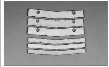
□ 1. Locate the six die-cut ply **wing joiners** for the bottom wing. Note that there are two different sizes of wing joiners for the front and back of the bottom wing.
