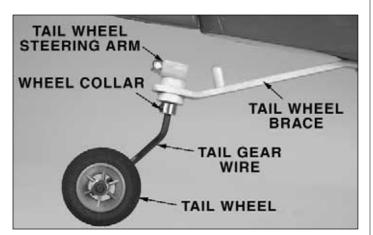
□ 9. Grind or file a flat spot on the tail wheel wire where the steering arm will be located. To locate its proper position align the tail wheel with the rudder and mark the tail wheel
