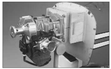
$\Box$  7. Mark the location for the throttle push rod (the supplied throttle pushrod will not be long enough for this purpose) and drill a 1/8" (3 mm) hole through the mount, firewall and the front former.
