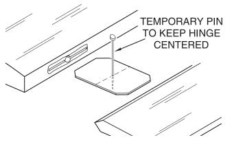
□ □ □ □ 4. Test fit the aileron to the wing with the hinges. If the hinges don't remain centered, stick a pin through the middle of the hinge to hold it in position.
