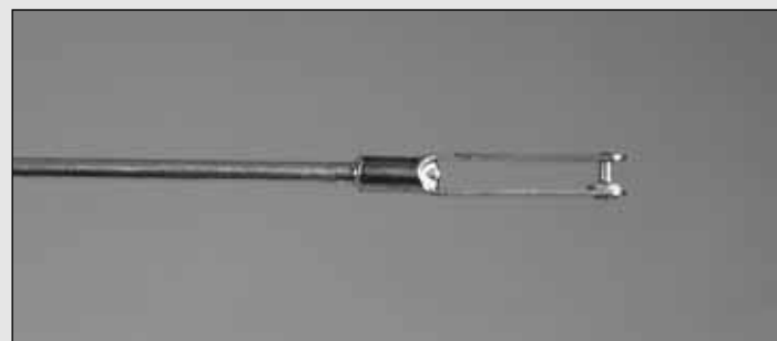
This is what a properly soldered clevis looks like; shiny solder with good flow, no blobs, flux removed.
