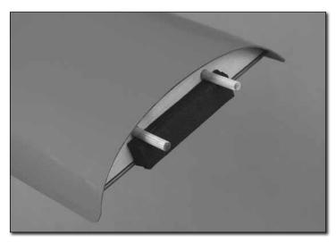
To make certain the canopy hatch always remains latched and secure, stick two or three layers of 1/8" [3.2mm] single-sided foam wing seating tape on the front of the canopy hatch as shown. This will assist the magnets in pushing the canopy all the way back assuring that the tabs remain locked. Additionally, always make certain the canopy is all the way back and locked before taking off.
