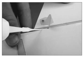
To improve the security of the elevator joiner wire, a small amount of CA can be carefully wicked into where the joiner wire enters the elevator halves.
