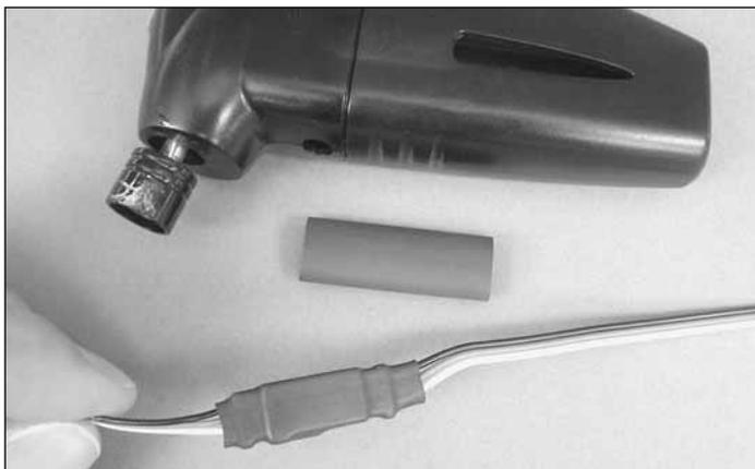
❑ 2. Connect a 6" [150mm] servo extension to the aileron servo and secure the connection with a 1-1/2" [40mm] piece of heat shrink tubing included with this kit—shrink the tubing with a heat gun or a hobby torch—use care not to scorch the wires!
