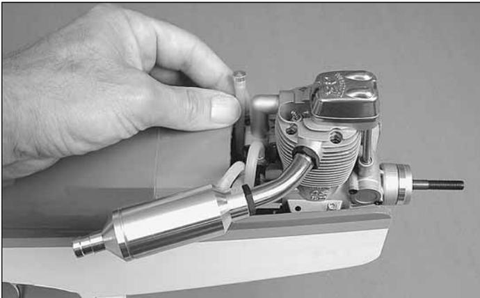
❑ 6. Mount the muffer to your engine and connect the fuel lines to the fuel tank as shown in the diagram. Note that the O.S.® FL .70 has two fuel fittings on the muffer. The fitting with the larger hole goes to the vent line on the fuel tank and the other fitting with the smaller hole goes to the crankcase vent in the backplate of the engine. The line with the fuel line plug goes to either of the “clunk” lines on the fuel tank that will be used for fueling and defueling the tank.
