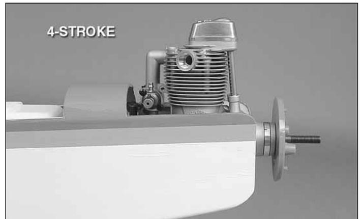
❑ 3. Place the backplate of the spinner on the engine and position the engine on the mount so there will be a 1/8" [3mm] space between the backplate of the spinner and the front of the fuselage. **Note:** Most 4-stroke engines will not be able to be positioned far enough aft on the mount to achieve this spacing, so just move the engine as far back as possible.
