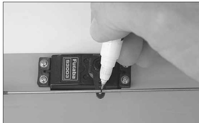
❑ 9. Use a fine-point felt-tip pen to mark the pushrod wire where it crosses the outer hole in the servo arm.
