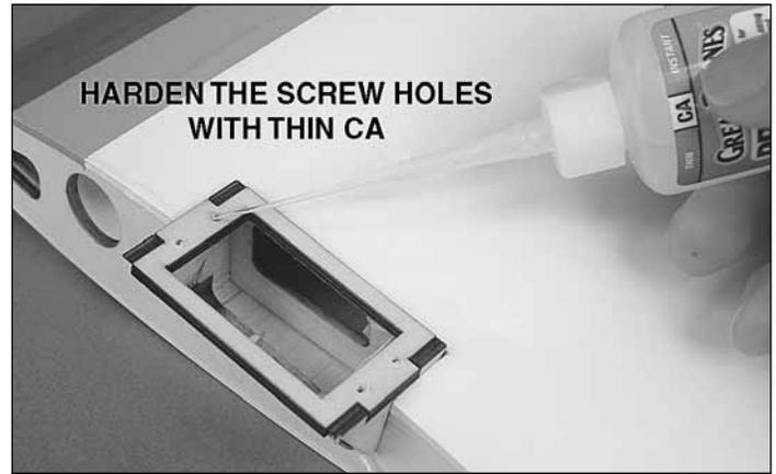
2. Temporarily mount the servo with the screws that came with it. Remove the screws and take out the servo. Add a few drops of thin CA to each screw hole. Wait a minute for the CA to harden and re mount the servo (guiding the wire between the right side of the servo and the servo mount). Don't overtighten the servo mounting screws—just make sure the heads of the screws apply a little pressure to the grommets and that the servo is secure.
