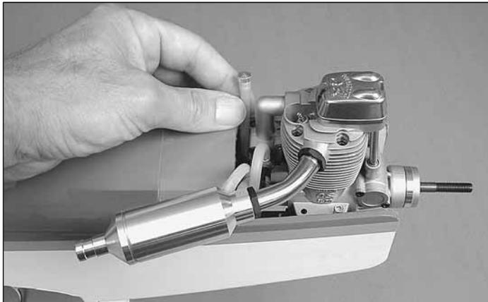
❑ 6. Mount the muffler to your engine and connect the fuel lines to the fuel tank as shown in the diagram. Note that the O.S.<sup>®</sup> FL .70 has two fuel fittings on the muffler. The fitting with the larger hole goes to the vent line on the fuel tank and the other fitting with the smaller hole goes to the crankcase vent in the backplate of the engine. The line with the fuel line plug goes to either of the "clunk" lines on the fuel tank that will be used for fueling and defueling the tank.
