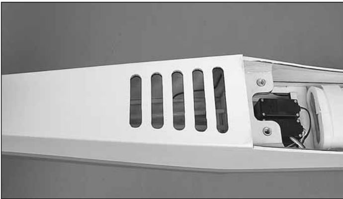
❑ 8. Use a hobby knife with a sharp #11 blade to cut the covering from the rounded air exit slots in the bottom of the fuselage behind the wing.
