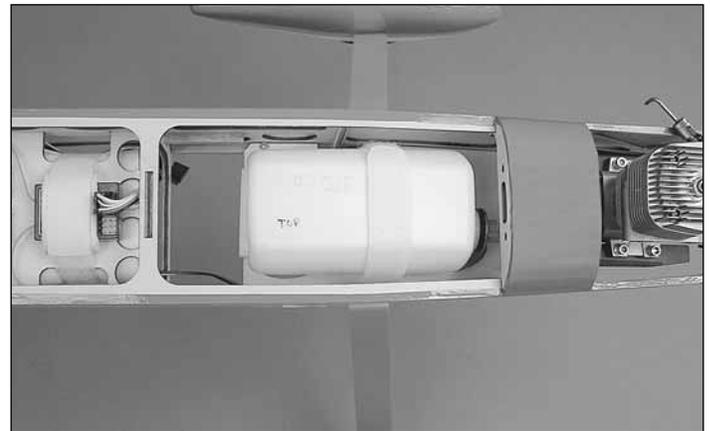
❑ 7. If using a glow engine, mount the fuel tank with the strap and foam rubber sheet. The fuel lines will be connected later.
