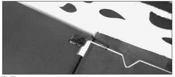
□ □ 6. Install a black nylon **snap keeper** onto the pushrod at the control horn.
