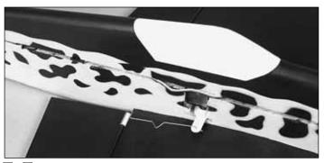
□ □ 1. Locate the two 2-3/4" [70 mm] prebent **aileron pushrods**. Slightly enlarge the outer hole on the aileron servo arm. Insert the Z-bend end of the pushrods into the outer hole in the aileron servo arm.
