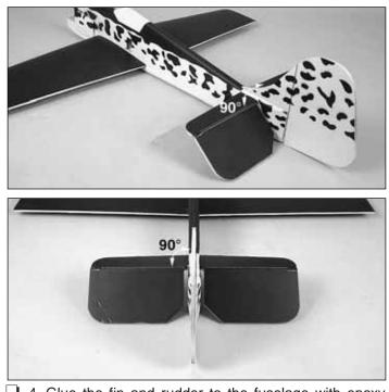
□ 4. Glue the fin and rudder to the fuselage with epoxy. Make sure that the fin remains perpendicular to the stab and centered on the fuselage.
