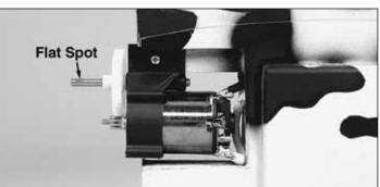
Install the Motor & Speed Control
