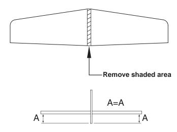
□ 3. Slide the wing out just enough to see the entire area covered by the fuselage. Remove the covering from the wing using a hobby knife 3/32" [2 mm] inside the marks you made. Apply a thin layer of epoxy and slide the wing into place. Use the marks from the previous step to align the wing. Clean up any excess glue with a paper towel. **DO NOT** use alcohol or any other solvent for cleanup as the paint finish will be affected.
