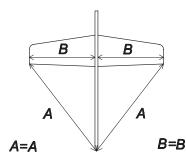
□ 1. Insert the wing into the fuselage. Be sure that the wing is centered and square by making sure all measurements are equal as shown in the sketch.
