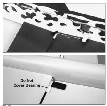
□ □ 5. Apply a small spot of foam-safe CA to the bottom of the control horn and insert it into the cut in the aileron. Press a nylon **backplate** on the backside of the control horn as shown.
