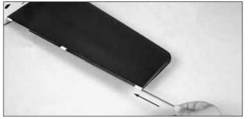
□ □ 3. Slide the loose carbon rod through the bearings.
