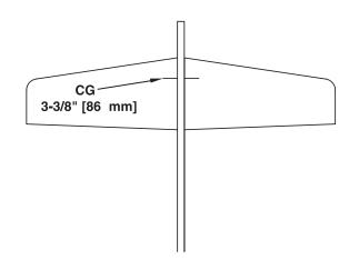
□ 1. Use a felt-tip pen or 1/8" [3 mm]-wide tape to accurately mark the C.G. on the top of the wing on both sides of the fuselage. The C.G. is located 3-3/8" [86 mm] back from the leading edge of the wing.
