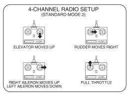
□ 3. Arm your ESC according to the manufacturers instructions. Make certain that the control surfaces and the motor respond in the correct direction as shown in the diagram. If any of the controls respond in the wrong direction, use the servo reversing in the transmitter to reverse the servos connected to those controls. Be certain the control surfaces have remained centered. Adjust if necessary.
