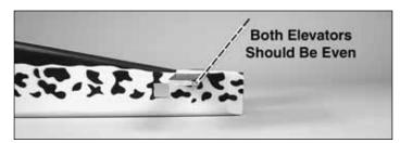
□ 3. Use foam-safe CA to glue one of the **elevator halves** to the carbon elevator rod. Then glue the other elevator to the carbon rod. Be sure the two halves are even as shown.
