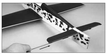
□ 2. Locate the 13.5" [343 mm] carbon **elevator rod**. Insert this rod into the preinstalled plastic bearings on the stab. DO NOT glue in place.
