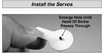
□ 1. Remove the screws and servo arms from all of your servos. Enlarge the hole in the center of the servo extender until the head of the servo screw passes through.
