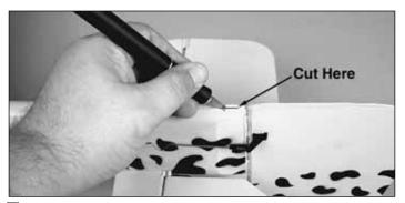
□ 5. Cut a 1" [25 mm] long groove in the bottom of the fuselage at the tail as shown. The exact location is not important; it simply needs to be at the tail of the fuselage. Do not attach the mount to the rudder control surface.
