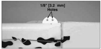
☐ 7. Drill two 1/8" [3.2 mm] holes in the mount. If not flying combat, use the two holes to route the antenna from the receiver.
