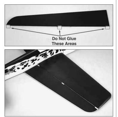
□ □ 4. Test fit an aileron onto the carbon rod as shown. If satisfied with the fit, glue the aileron to the carbon rod using CA. DO NOT glue the aileron to the bearings. The rod must freely rotate in the bearings, so the aileron must only be glued to the carbon rod.
