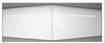
□ 1. Using epoxy, join the two **wing halves** together, making sure to align the root sections.
