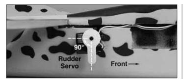
□ 5. Epoxy the other tail servo into the cutout from the right side of the plane side with the output shaft toward the front. Center the servo with your radio and screw the extended arm onto the output shaft with the arm oriented straight down.
