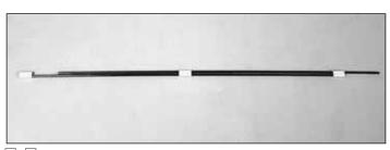
□ □ 1. Locate one of the carbon **wing hinge assemblies**. One of the carbon tubes is glued to the bearings; the other is free to rotate. Remove the loose carbon tube to prevent accidental gluing in the next steps.
