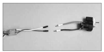
□ 1. Connect the output wires of your ESC to the motor. Check that the motor operates in the proper direction prior to installing it.
