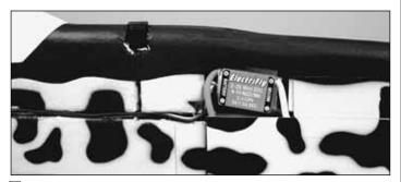
□ 2. Install the ESC as shown using a small section of hook and loop tape. Place the hard "hook" side in the provided cutout in the fuselage and the softer "loop" side on the back of the ESC. If your ESC has a BEC switch, install it in the provided cutout. For some electronic speed controls, it may be necessary to trim the foam slightly to allow for wire clearance and switch mounting.
