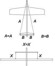
□ 1. Slide the stab into the slot in the rear of the fuselage. Center it as you did with the wing. Make sure the measurements shown in the sketches are equal. Glue the stab in place when satisfied with the fit.
