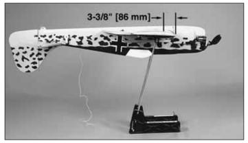
□ 2. With the wing attached to the fuselage and all parts of the model installed (ready to fly), place the model upsidedown on a Great Planes CG Machine, or lift it upside-down at the balance point you marked.
