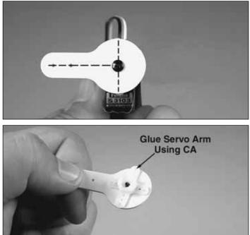
□ 3. Place the original servo arm over the screw, and glue the top of the arm to the extender with CA. Some servo arms have small flanges projecting from the top. If your servo arms have these flanges, sand them off before gluing.
