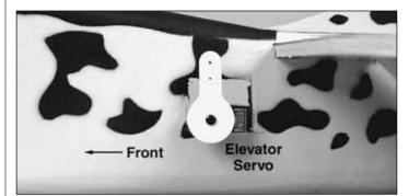
□ 4. Use epoxy to glue a servo into the bottom of the rear servo cutout from the left side of the plane. The output shaft should be toward the front of the fuselage. Center the servo with your radio and screw the extended arm onto the output shaft with the arm oriented straight up.
