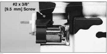
$\Box$  3. Slide the gearbox onto the square **wood stick** in the nose. Secure it with the supplied #2 x 3/8" [9.5 mm] screw.
